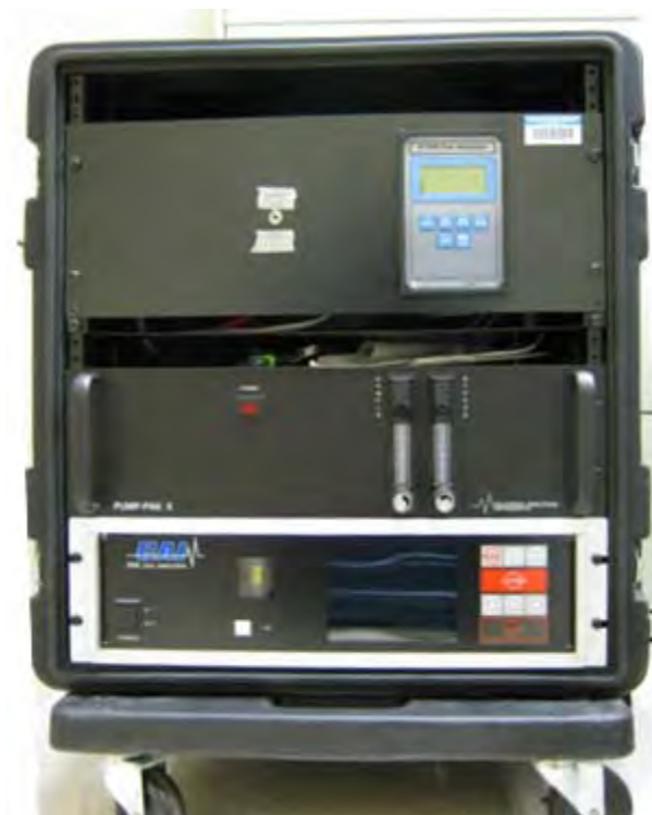
Figure 9-14: Gas analyzer train used during experiments. HiTech K1550 top right, California Analytical ZRE bottom, California Analytical Pump Pack II middle
