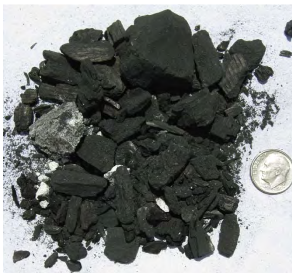
Figure 10-28: 'Rest of Gasifier' sample, comprised mostly of charcoal and wood char
