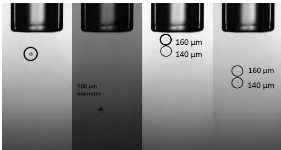
Figure 2-28: Images of 50 % glycerin droplets produced at 3.0 Hz, 0.01 \mu\text{L}/\text{min} , 55 V drive amplitude. Images are taken using PCO camera with Nikon 105mm lens at 143 FPS
