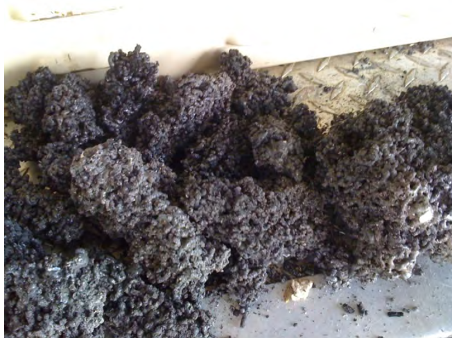
Figure 10-19: Poultry litter pellet clinkers from 40% pellet run
