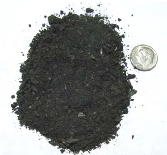
Figure 10-29: Char collected from chamber below gasifier grate, labeled 'Below Grate'
