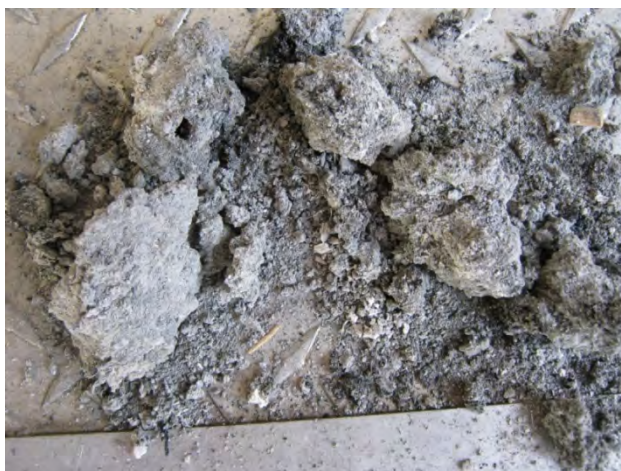
Figure 10-24: Easily crumbled, grey amorphous ash from raw poultry litter with limestone
