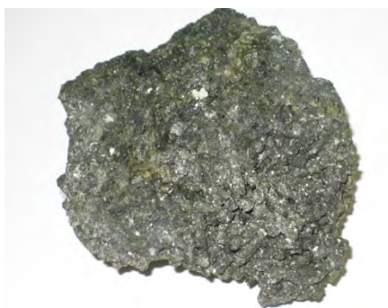
Figure 10-18: Poultry litter clinker from initial trial, ~18 cm wide
