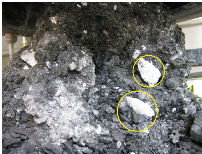
Figure 10-26: Ash mound found when gasifier is opened at seam above the grate, white deposits circled
