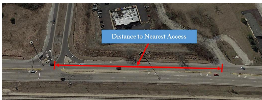
Figure 3. Distance to the Nearest Access Point in the Vicinity of an Interchange Terminal
