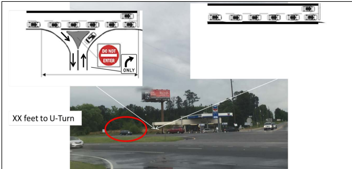
Figure 5.13 Example of Countermeasures for Preventing WW Left Turns from a Gas Station in AL
