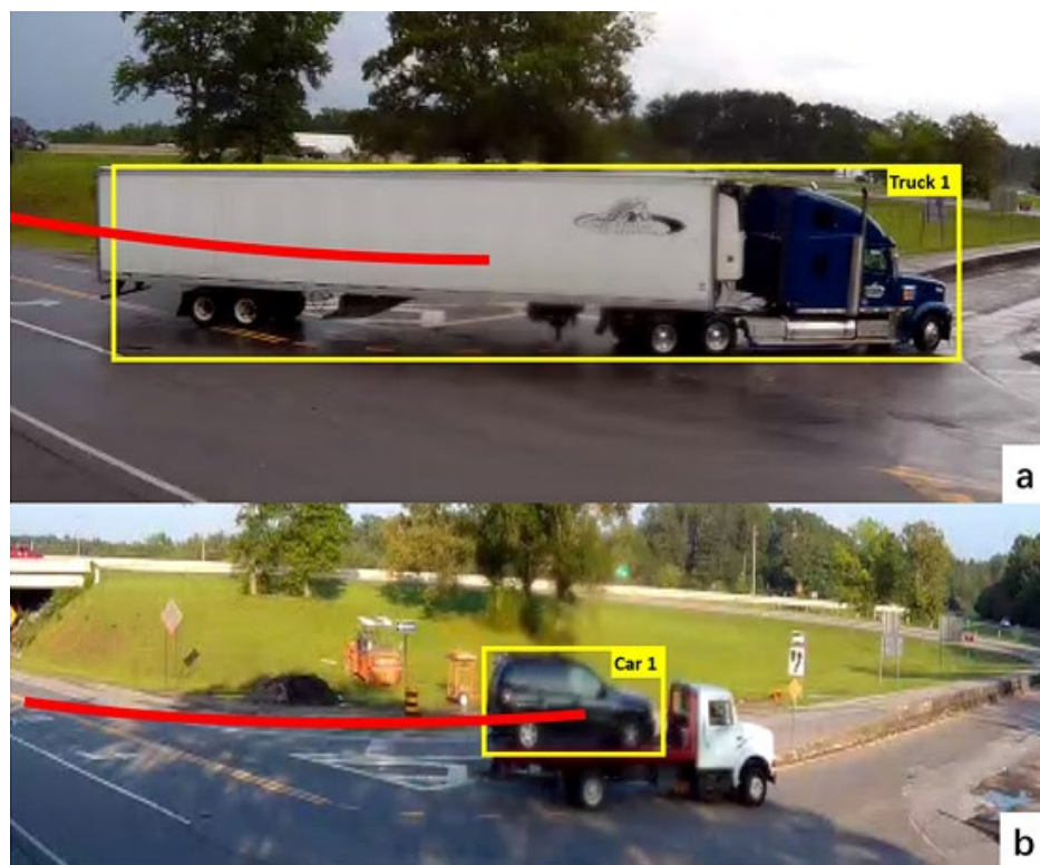
Figure 12 Two types of false alert: (a) oversized vehicle and (b) passenger vehicle carried by truck
