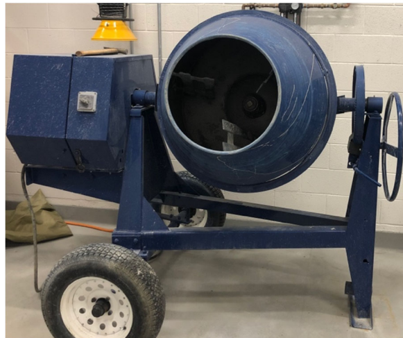
Figure 3-1: Concrete mixer used
