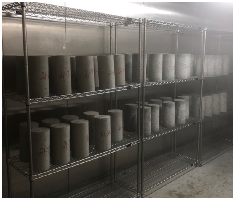
Figure 3-9: Cylinders in Final Curing Room
