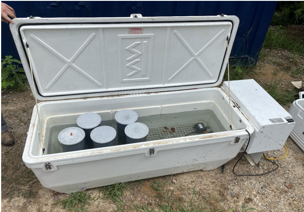
Figure 6-28: Jobsite 4 SIC Curing Box
