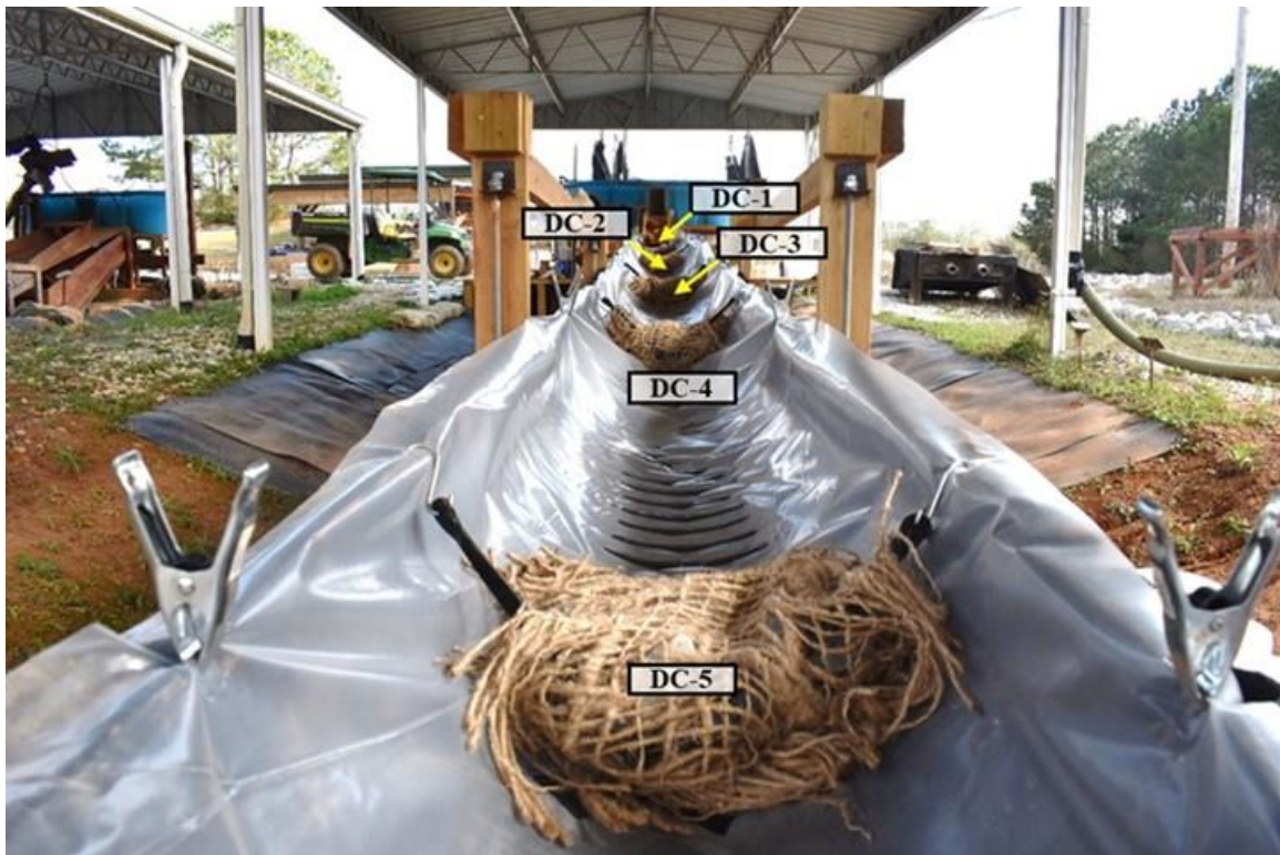
Figure 5-11: Scaled-down Rock Ditch Checks in the Flume
