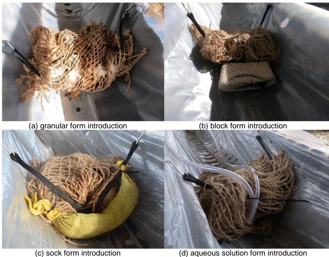
Figure 5-15: Introduction of Different Flocculant Forms in Flume Experiments
