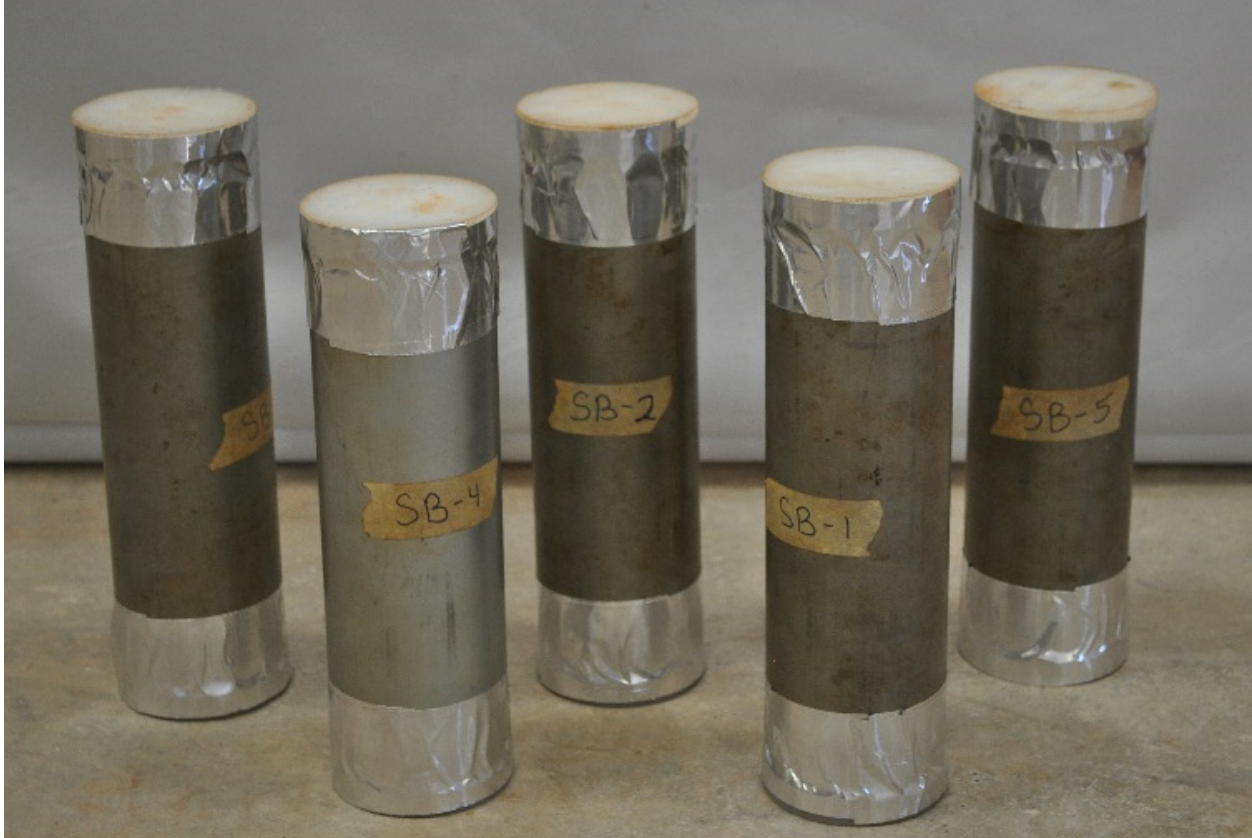
Figure 2.49: SM Cylinders During Initial Curing Period
