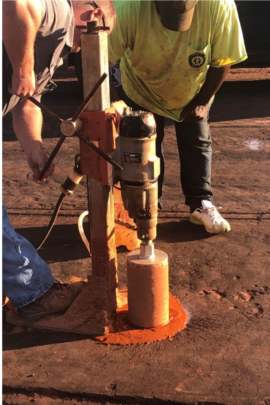
Figure 3.33: Core being Recovered from the Section
