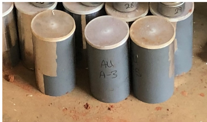
Figure 3.28: PM Specimens During Initial Curing on Site
