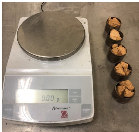
Figure 3.16: Dry Soil Cement Samples about to be Weighed
