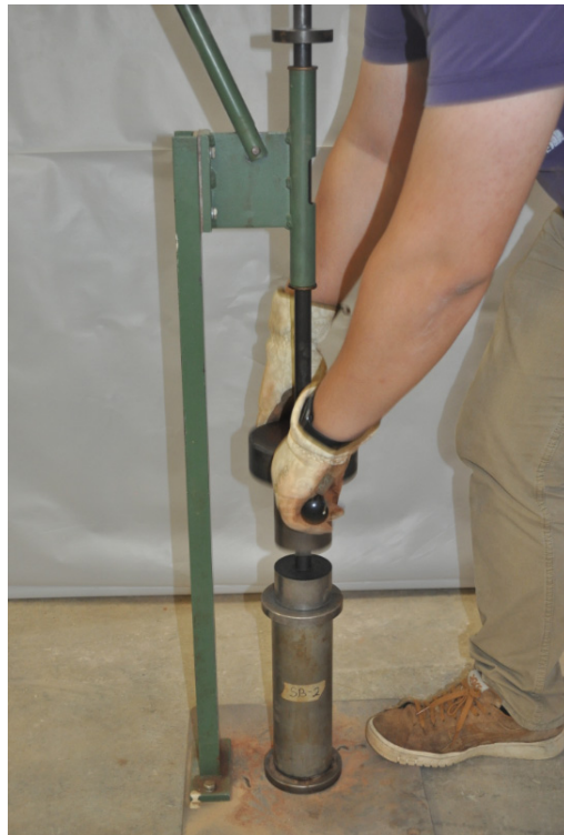
Figure 2.48: SM Cylinder Compacted with Drop-Weight Machine
