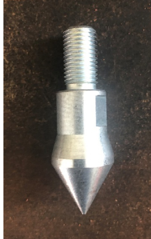
Figure 3.30: Replaceable DCP tip
