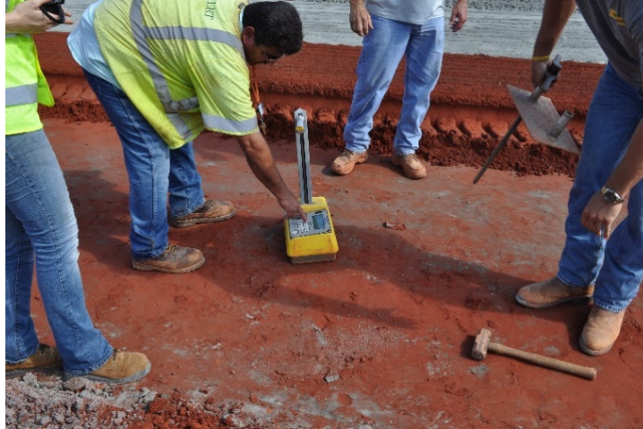
Figure 3.29: Use of Nuclear Gauge on Test Section
