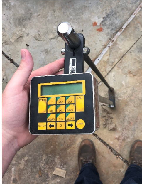
Figure 3.20: Kessler Magnetic Ruler
