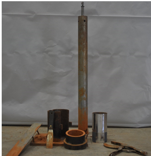
Figure 2.42: Plastic-Mold Preparation Apparatus
