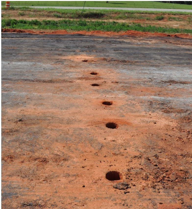
Figure 3.35: Multiple Attempts at Retrieving a Valid Core Sample
