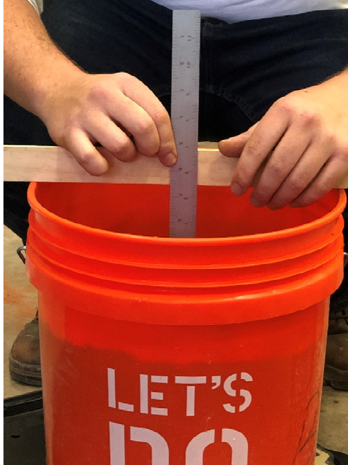
Figure 3.19: Height Measurement of DCP Specimen
