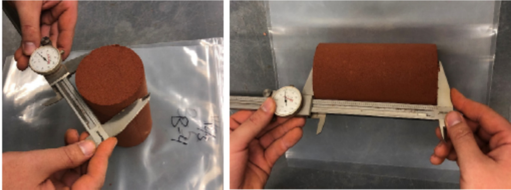
Figure 3: Measurements of the soil cement cylinder using a caliper
