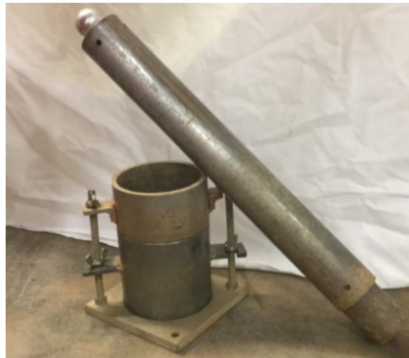
Figure 2.41: Proctor Mold and 5.5-Pound Hammer
