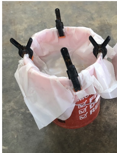
Figure 3.13: Initial Curing of DCP Specimen
