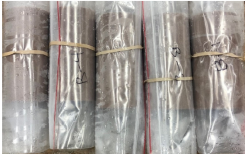
Figure 2: Cylinders in sealable plastic bags
