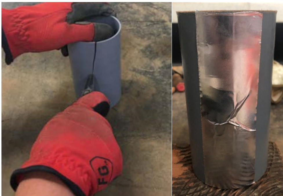
Figure 2.45: Plastic Mold Modification Process (McLaughlin 2017)
