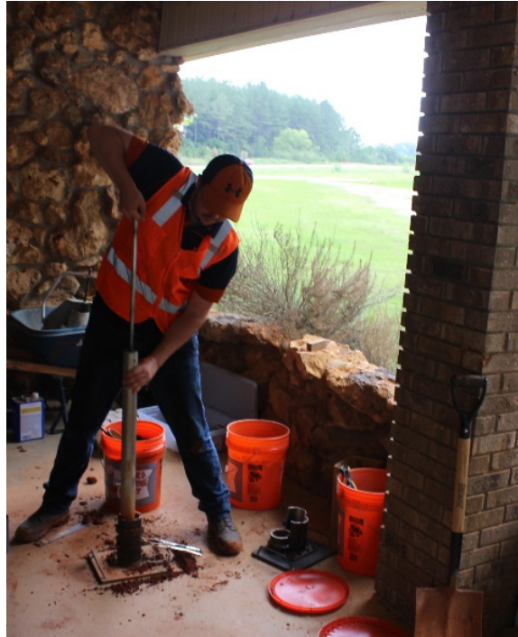
Figure 3.27: Soil Cement Cylinder being Compacted at Jobsite House
