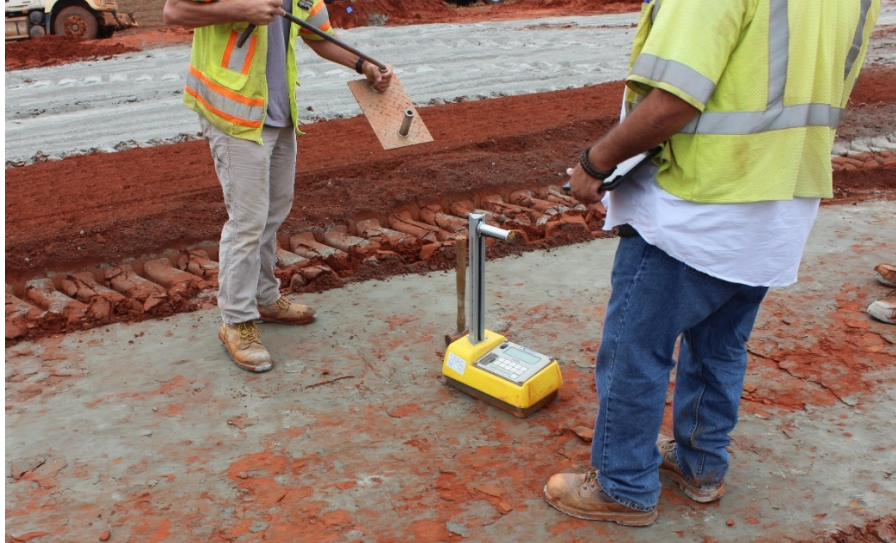
Figure 2.20: Nuclear Gauge Method Right after Rolling
