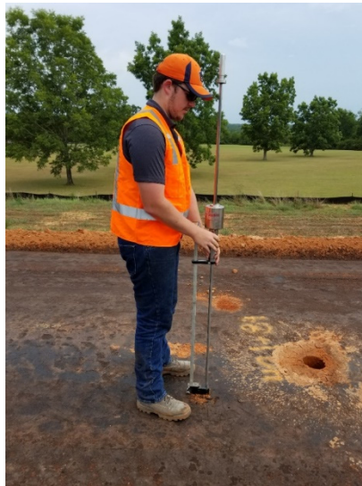
Figure 2.29: DCP Equipped with a Magnetic Ruler Used for Testing
