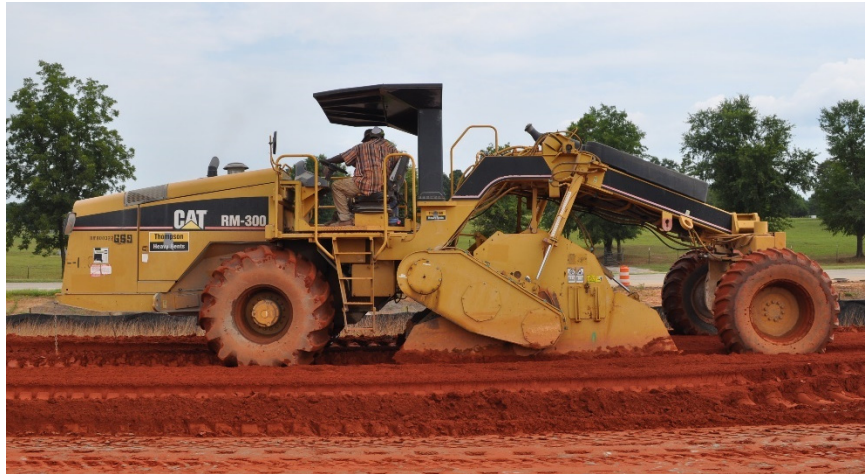
Figure 2.10: Transverse Single-Shaft Mixer
