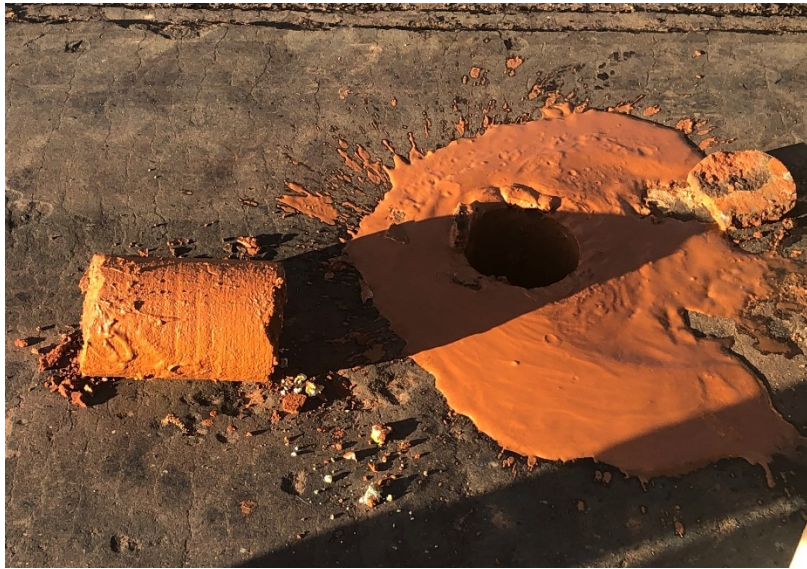
Figure 2.24: A sampled core that broke off during removal
