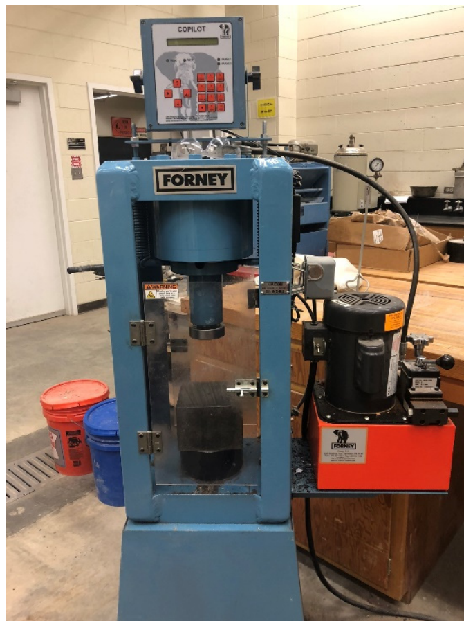
Figure 3.17: Forney 100-kip Compression Testing Machine
