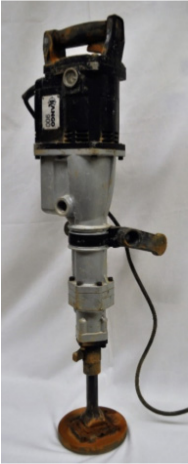
Figure 2.32: Vibrating Compaction Hammer with Circular Steel Plate
