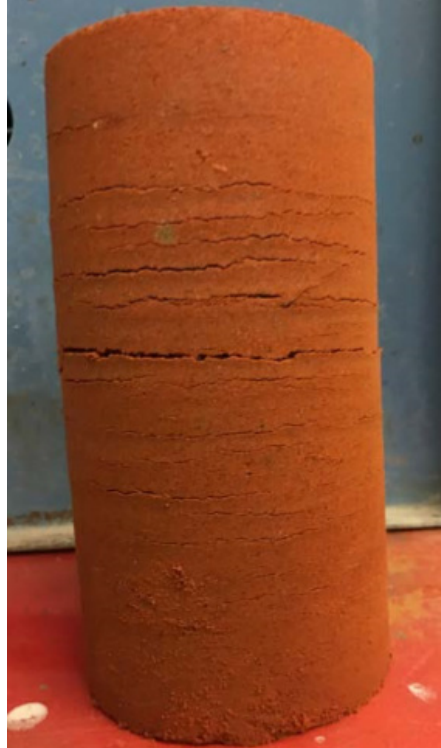
Figure 2.44: Plastic-Mold Specimen Damaged by the Extrusion Process (McLaughlin 2017)
