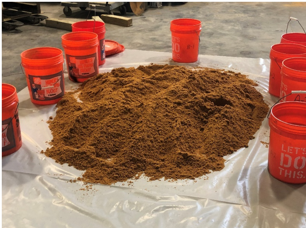
Figure 3.7: Mixing of Soil Prior to Batching
