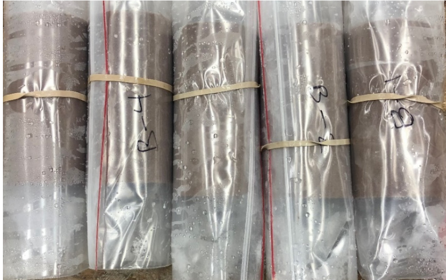
Figure 3.14: Final Curing of the PM Cylinders
