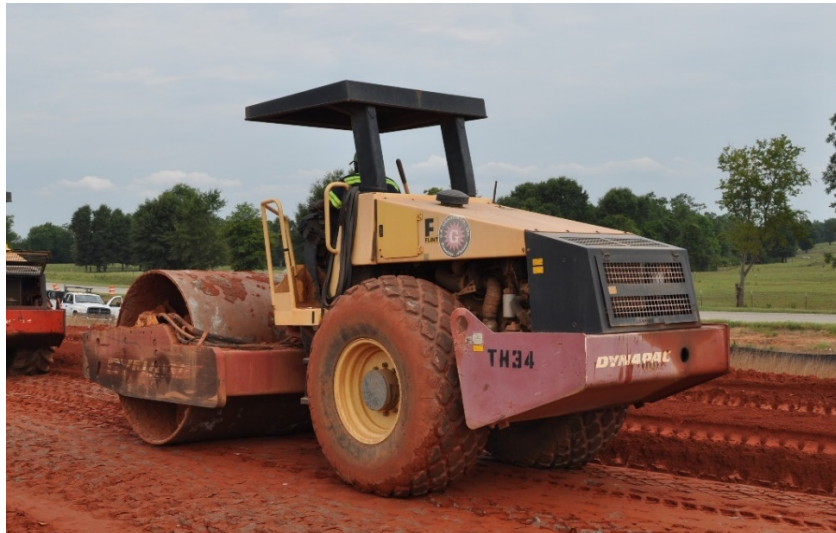
Figure 2.17: Vibratory Steel-Wheeled Roller
