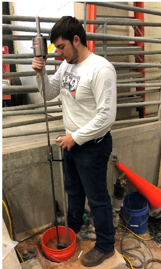
Figure 3.21: DCP Testing Arrangement in the Specimen
