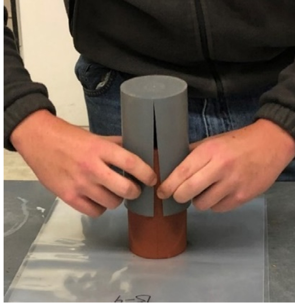
Figure 3.12: Specimen Removal from Plastic-Mold
