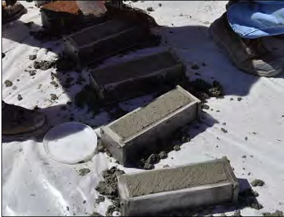
Figure 4-3: Preparation of concrete prisms on the jobsite
