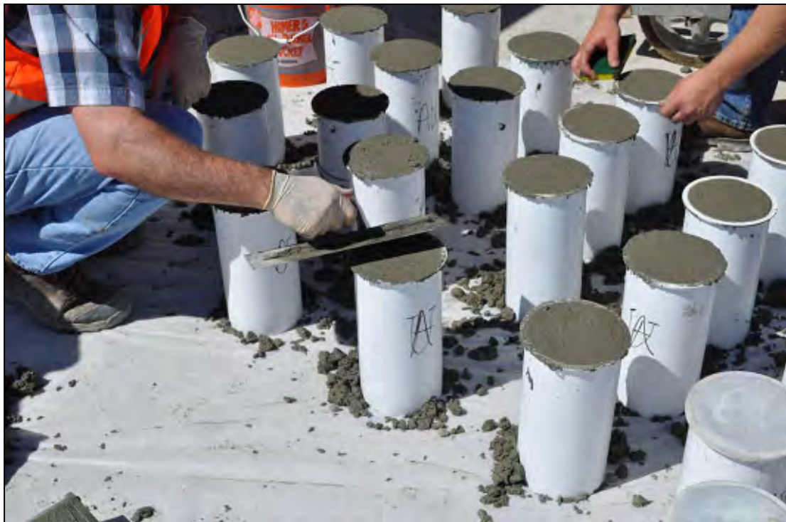
Figure 4-2: Preparation of concrete cylinders on the jobsite
