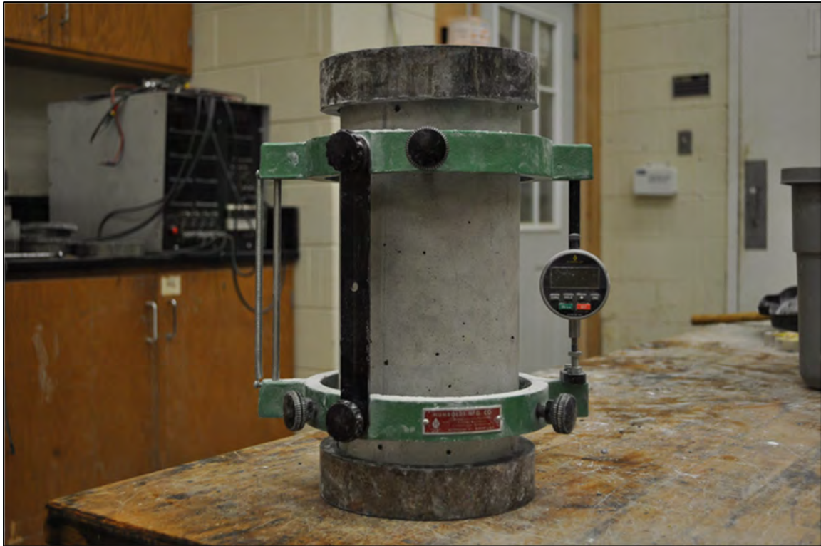
Figure 4-6: Compressometer used to test modulus of elasticity
