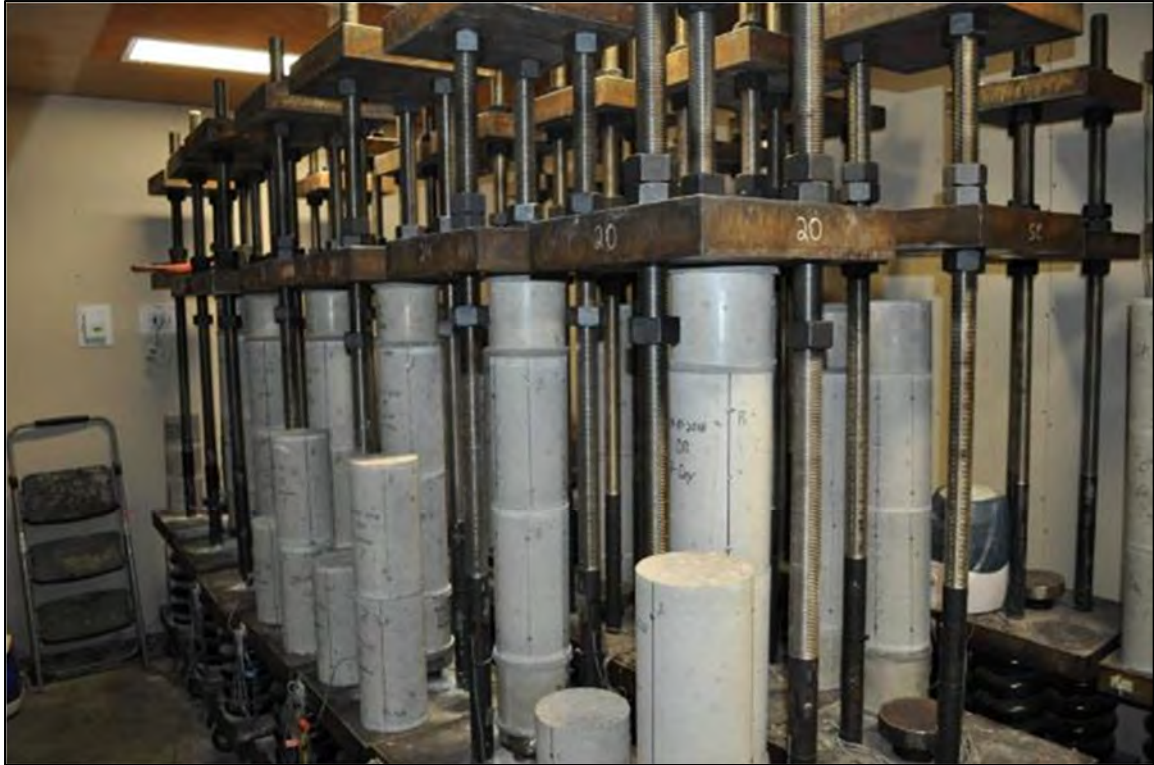
Figure 4-10: Creep testing room
