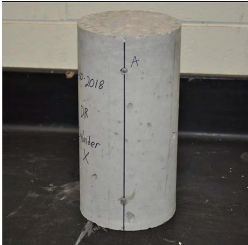
Figure 4-8: DEMEC points installed on shrinkage cylinder
