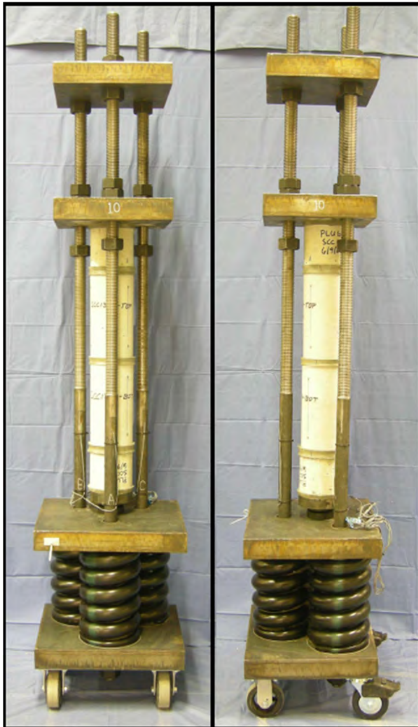
Figure 4-12: Creep testing frame (Kavanaugh 2008)
