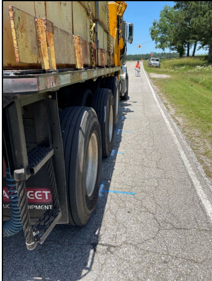
Figure 5.32. Load truck in 1/4 stopping point (load line 2) at the Bain's Gap Road culvert.
