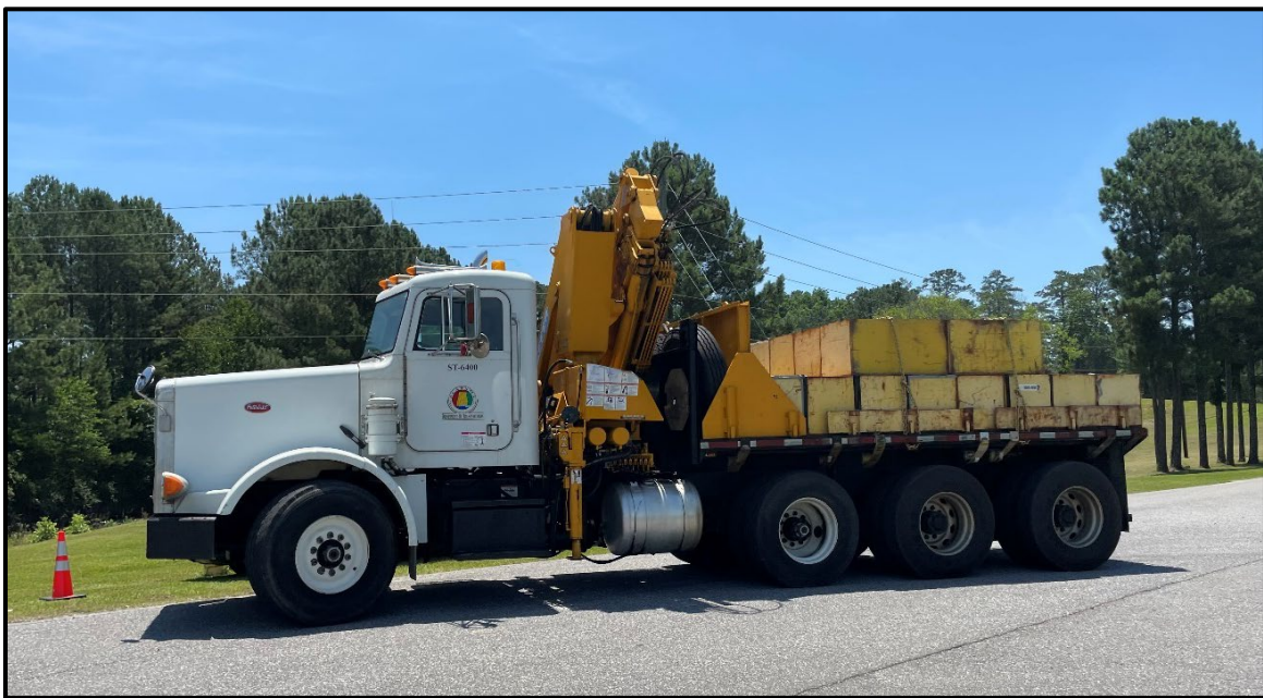
Figure 5.10. ALDOT load test vehicle.
