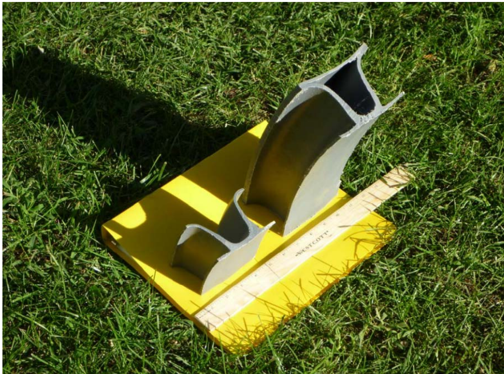
Figure 5-11: Dual-Wall and Triple-Wall Profiles of ADS Pipes (Hoppe 2011)
