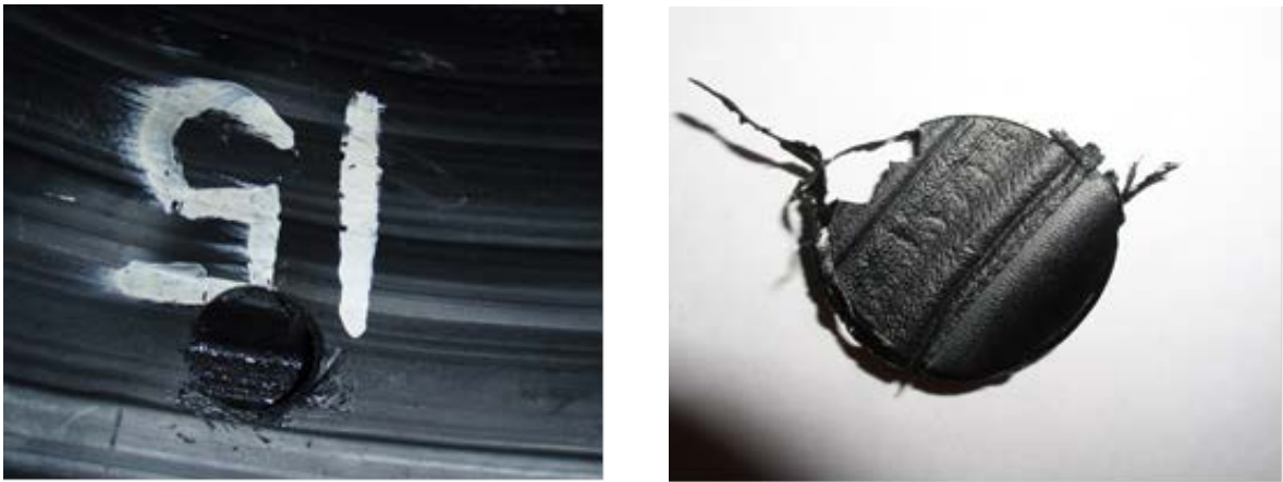
Figure 2-7: Samples taken for Oxidation Induction Time Tests (Goddard 2008)
