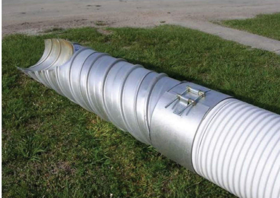
Figure 5-35: Polyvinyl Chloride Pipe with Metal Pipe Ends (Maher et al. 2015)
