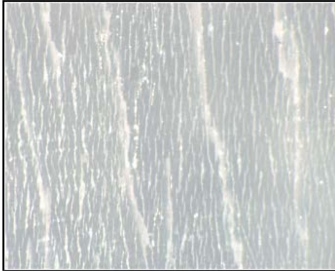
Figure 5-33: Micro-cracking of UV Exposed Polypropylene (Jones 2002)
