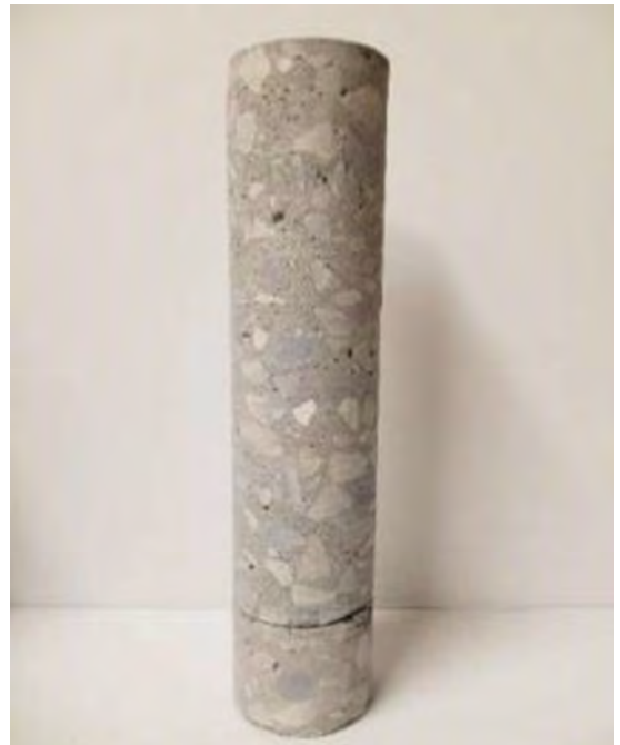
Figure 4-34: Deep Delamination Simulation using Sand Layer in Specimen DL4
