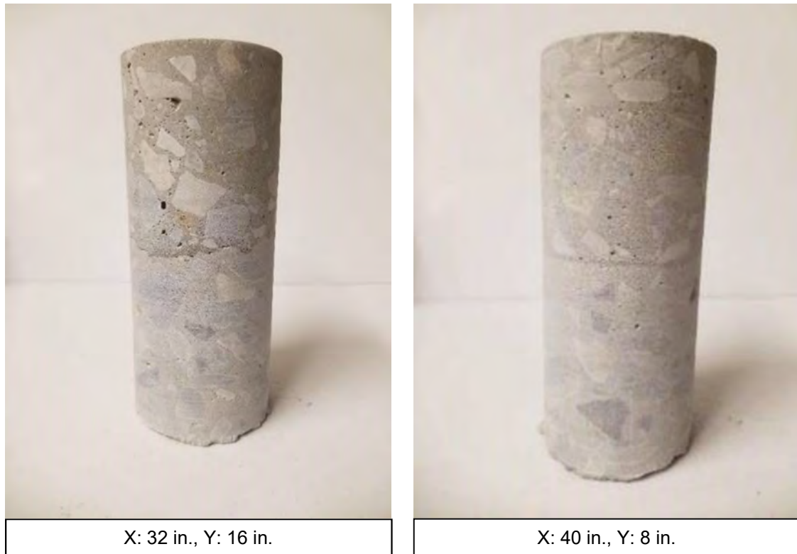
Figure 4-43: Well-Consolidated Cores from Specimen PC1
