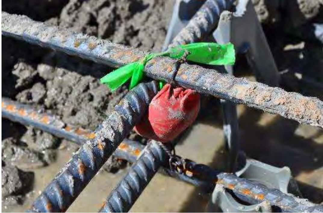
Figure 5-8: Shallow Void Simulation in Defect V1
