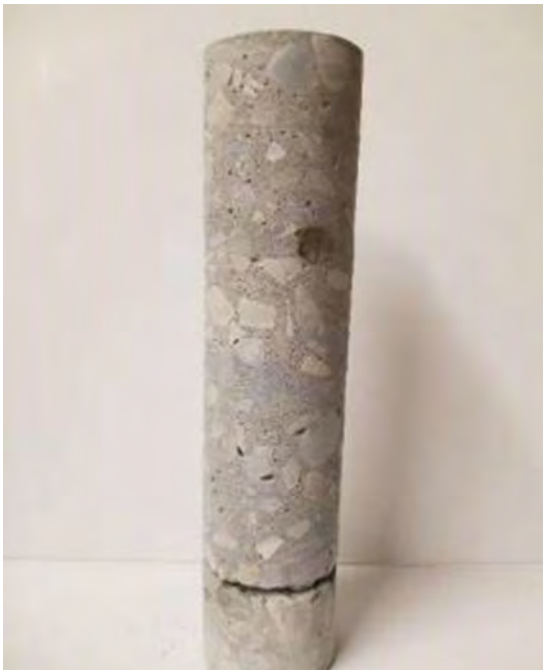
Figure 4-34: Deep Delamination Simulation using Sand Layer in Specimen DL4
