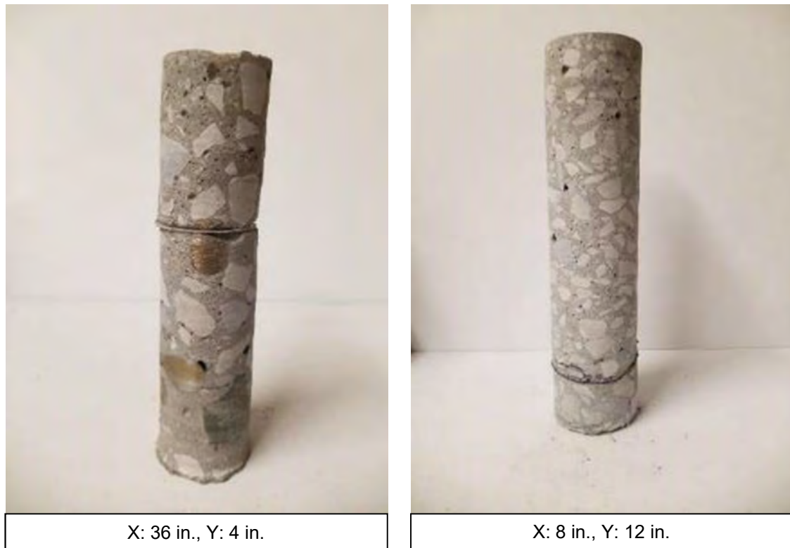
Figure 4-36: Specimen DL5 Shallow Delamination (Left) and Specimen DL6 (Deep Delamination (Right)
