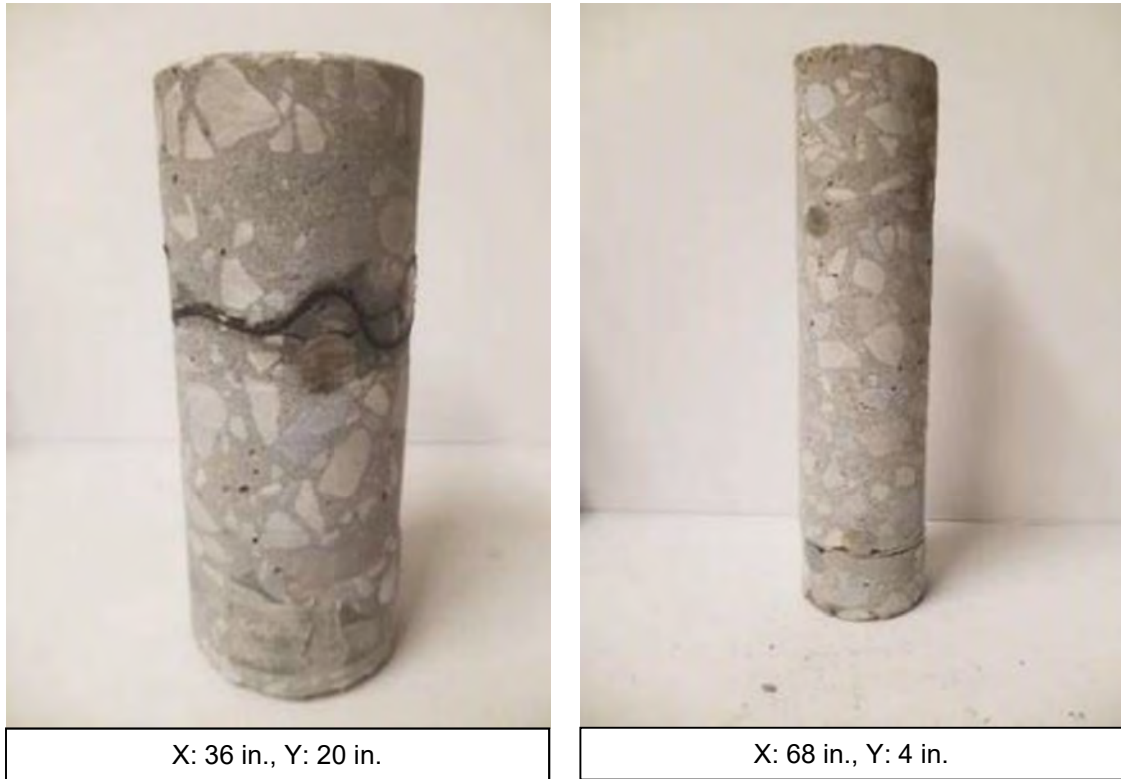
Figure 4-31: Specimen DL1 Shallow Delamination (Left) and Specimen DL2 Deep Delamination (Right)
