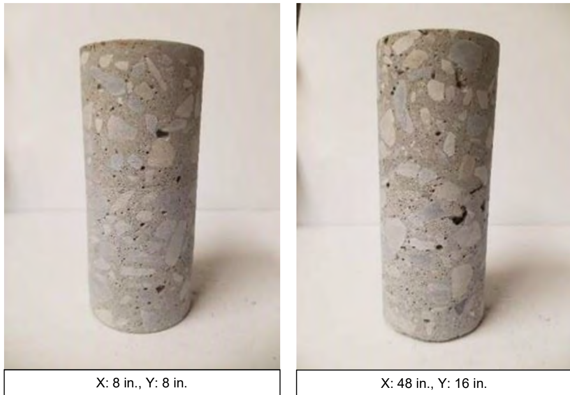
Figure 4-44: High Entrapped Air Content in Specimen PC2 Cores
