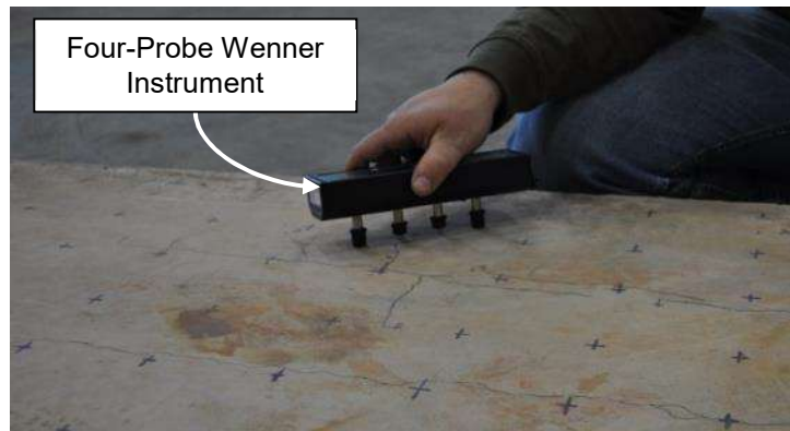
Figure 2-13: ER Evaluation of Deteriorated Laboratory Specimen
