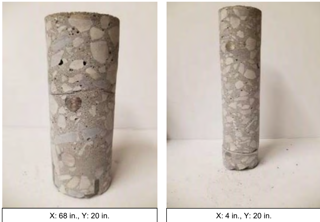
Figure 4-37: Partially bonded Delaminations in Specimens DL7 (Left) and DL8 (Right)
