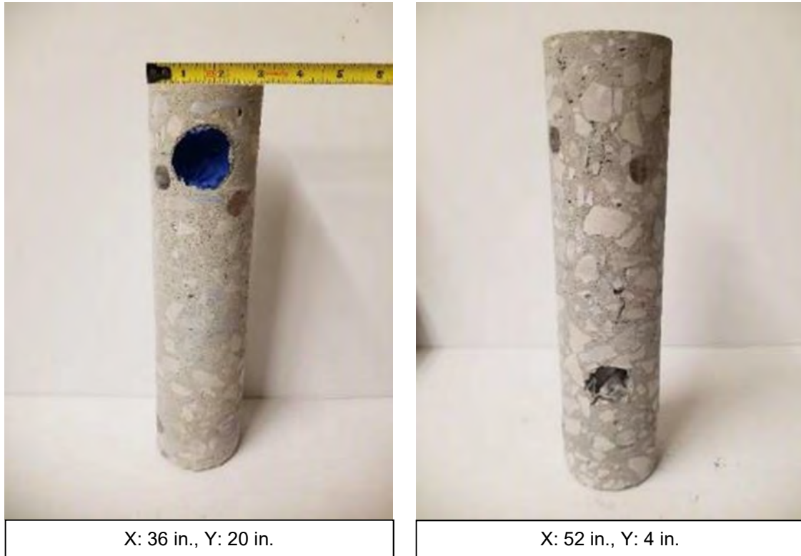
Figure 4-45: Floated Void in Specimen V1 (Left) and Deep Void in V2 (Right)
