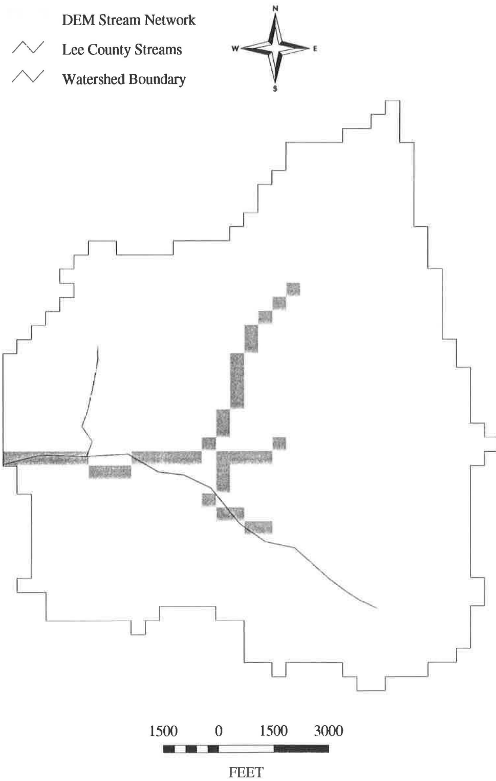
Figure 6. TIGER File Streams Overlaying Stream Network Derived from a DEM.
