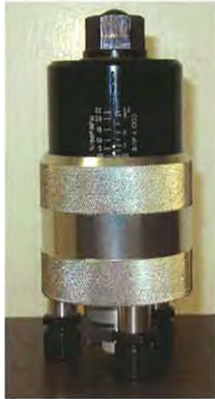
Figure A.1 - Elcometer 106 Fixed-alignment Portable Adhesion Tester
