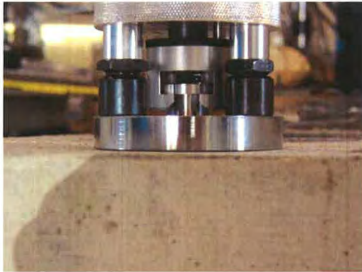
Figure A.7 – Claw of the Elcometer 106 Engaged with a Typical Test Dolly
