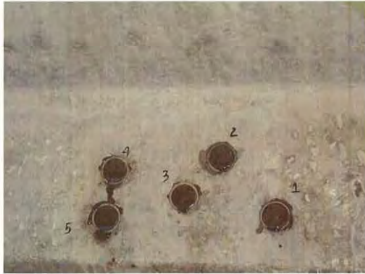
Figure A.5 – Test Surfaces after Application of Tyfo S Epoxy and Light Sanding
