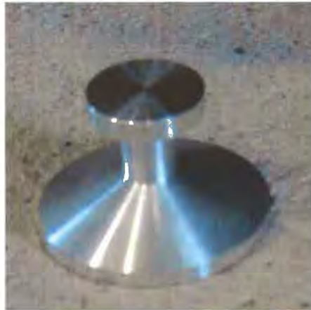
Figure A.2 – Typical 1.57-in. Diameter Test Dolly
