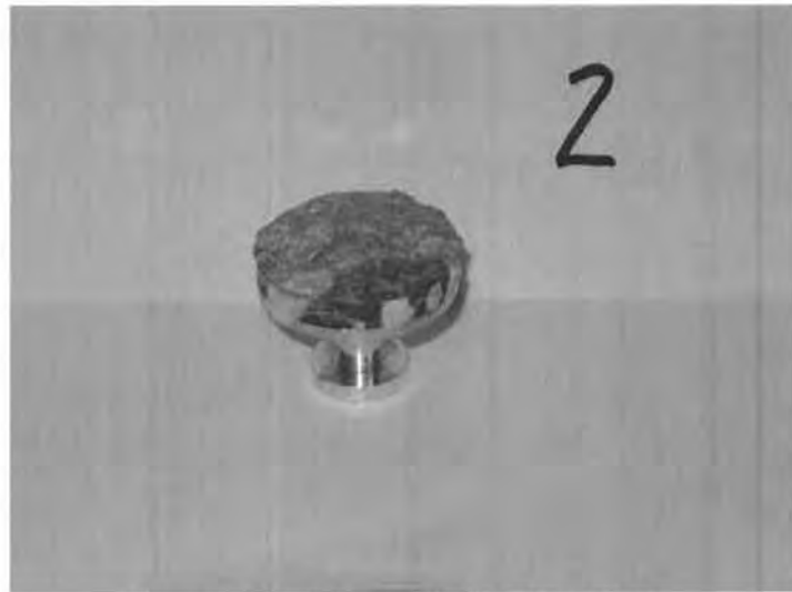
Figure A.9 – Test Dolly #2 after Failure
