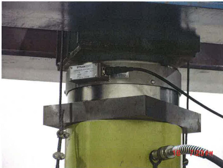
Figure 3.8 The 300-kip Compression Loadcell
