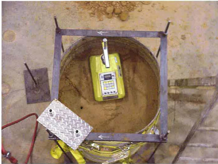
Figure 3.5 Nuclear Density Gauge Checks the Density
