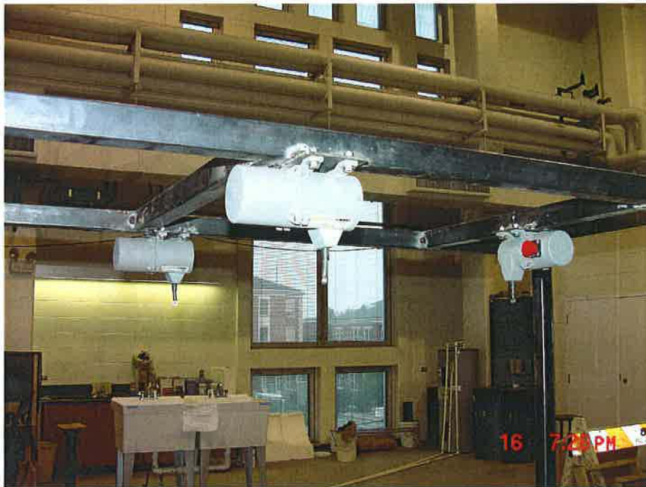
Figure 3.9 Cable Extension Displacement Transducers
