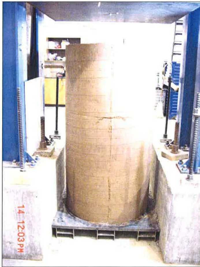
Figure 3.7 Reinforced Cylinder Prior to Testing
