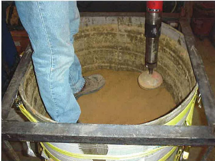
Figure 3.4 Compaction of Sample Using a Pneumatic Compactor
