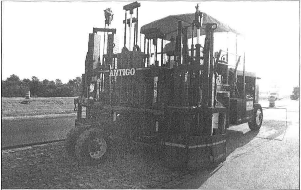
Figure 2.5 Multi-Head Breaker (photo courtesy of Dr. Kevin Hall, University of Arkansas).
