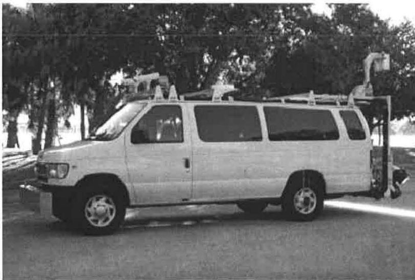
Figure 2.4 Automated Pavement Condition Survey Vehicle (ICC, 2003).
