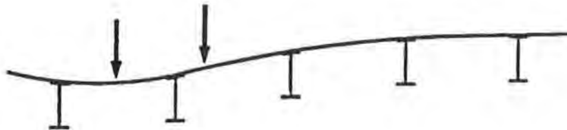
b. deck-girder displacements (superposition of local and global)
