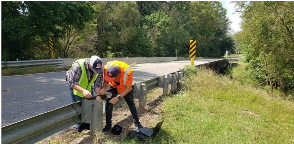
Figure 61. BIN 010738, Lapine, AL. Installation of HOBOT atmospheric pressure sensor and HOBOT Rain Gauge.
