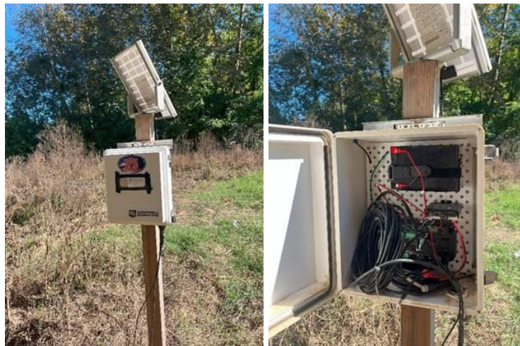
Figure 78. BIN 008598, Tuskegee, AL. Solar panel and enclosure containing data acquisition system.
