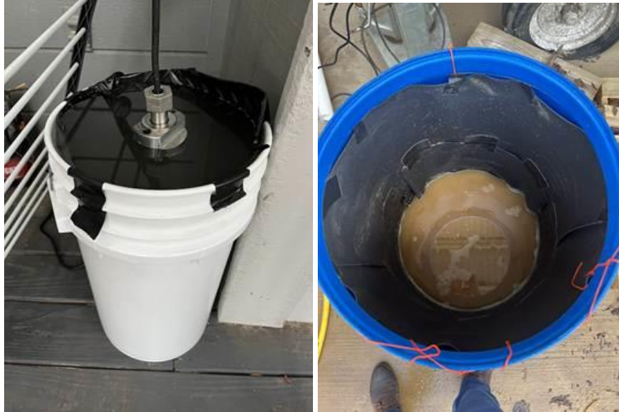
Figure C2. Turbidity tests were conducted in a 7-gallon bucket and a 55-gallon barrel.
