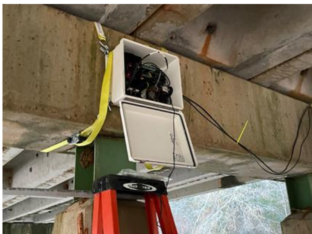
Figure 66. BIN 015002, Enterprise, AL. Enclosure housing the data logger and battery.
