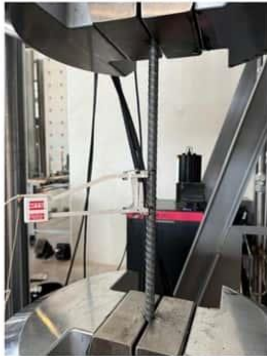
Figure 3-2 Tensile test of #4 reinforcing steel
