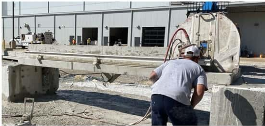
Figure 6-12 Cutting groove for positive bending test (Top) and for negative bending test (Bottom)
