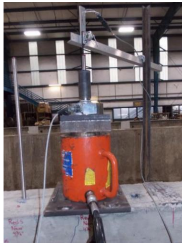
Figure 2-5 Pull-out test setup for TiAB (Barker 2014)
