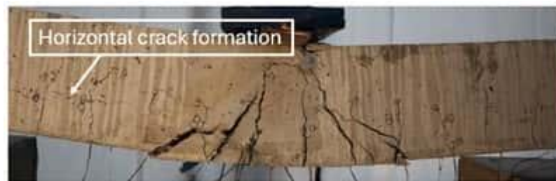
Figure 5-16 Horizontal crack formation in the shear span of SB96
