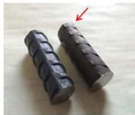
b) shallow deformations on Ti bar (rotated 120° from Figure a)
