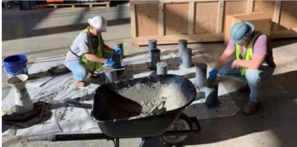
Figure 4-7 Cylinder preparation for strength evaluation
