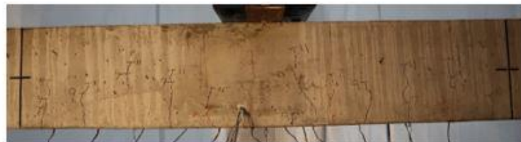
Figure 5-1 Condition of Specimens at yielding of the tension steel reinforcement.
