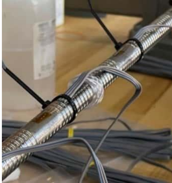
Figure 4-14 TiAB with wedge and strain gauges
