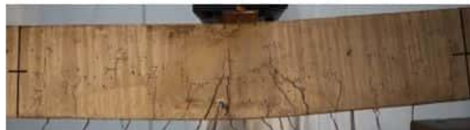
Figure 5-2 Condition of Specimens during detection of concrete crushing.
