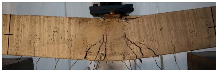
Figure 5-3 Condition of Specimens after peak load.
