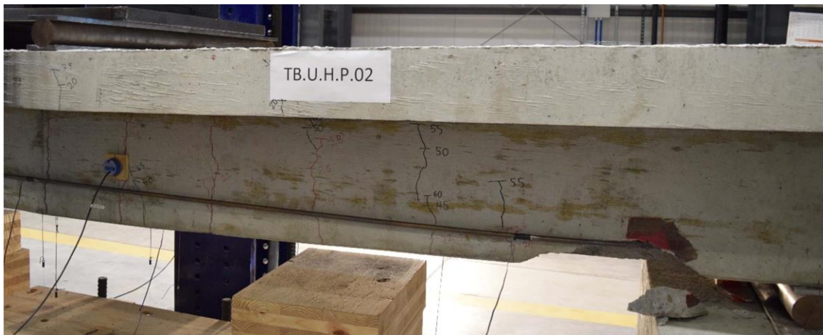
Figure 7-17 Anchorage failure of Specimen TB.U.H.P.02
