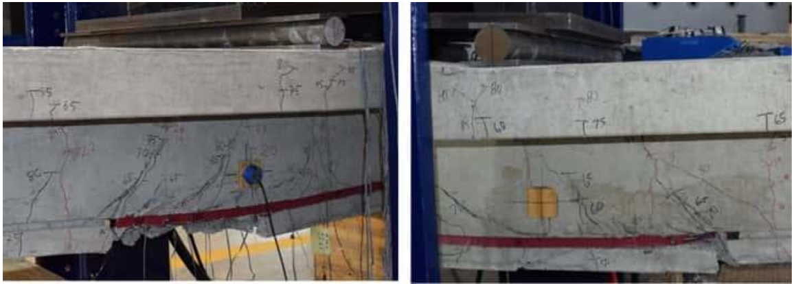
Figure 7-3 Inclined shear cracks near hook ends and interface failure for Specimen TB.G.H.P.01
