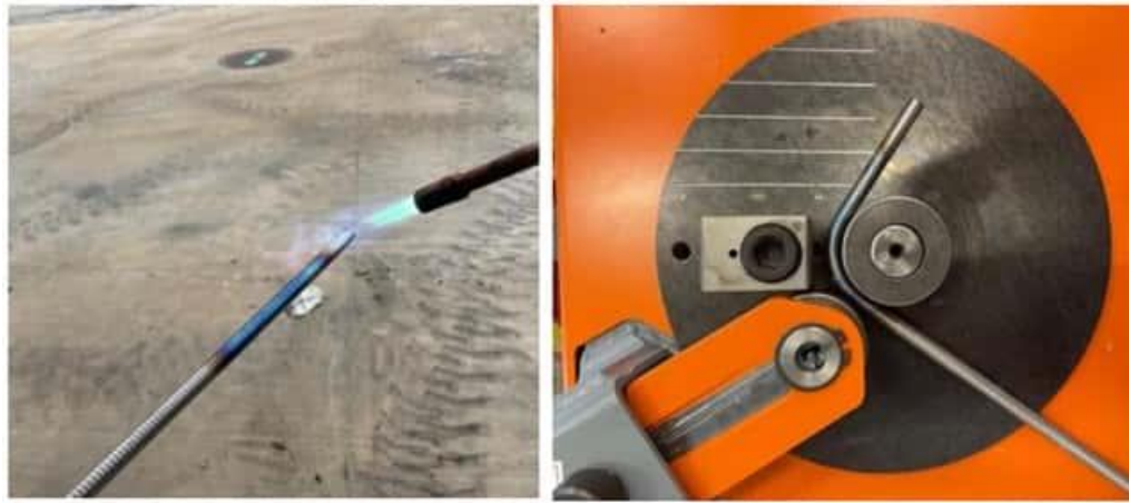
Figure 4-13 TiAB heating (heating) and bending (right)
