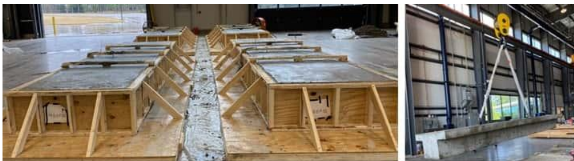
Figure 6-5 Specimen after casting (Left) and Lifting of the specimen (Right)
