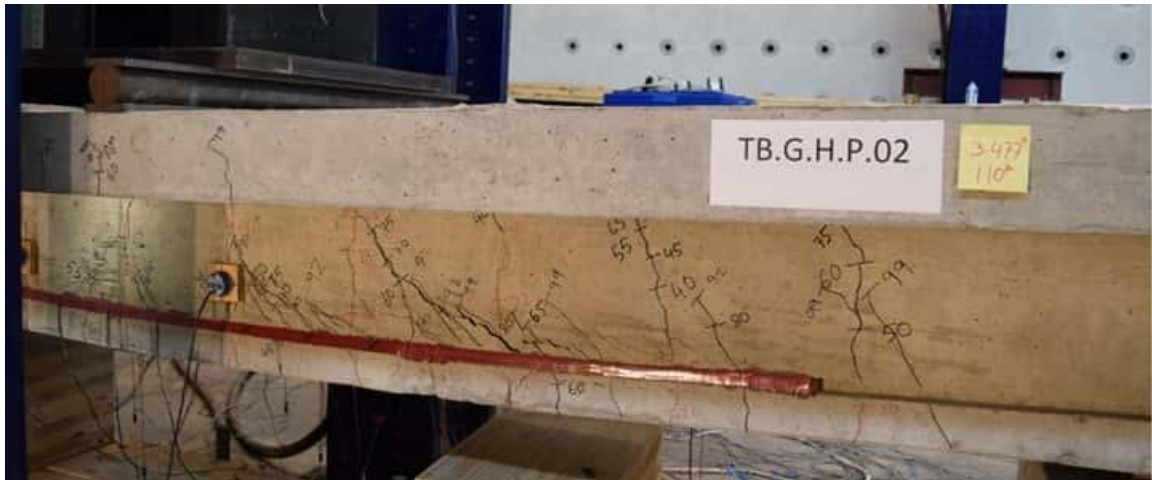
Figure 7-4 Concrete-epoxy interface failure for Specimen TB.G.H.P.02
