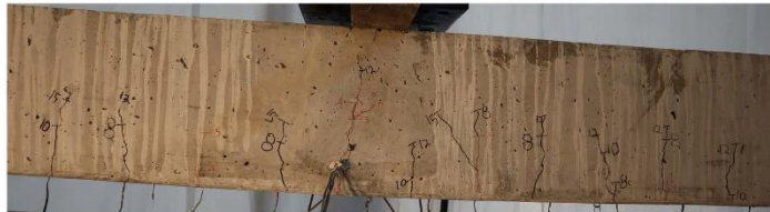
Figure 5-11 Cracking condition of specimens at 0.005 steel strain
