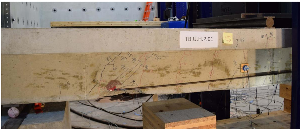
Figure 7-16 Anchorage failure of Specimen TB.U.H.P.01
