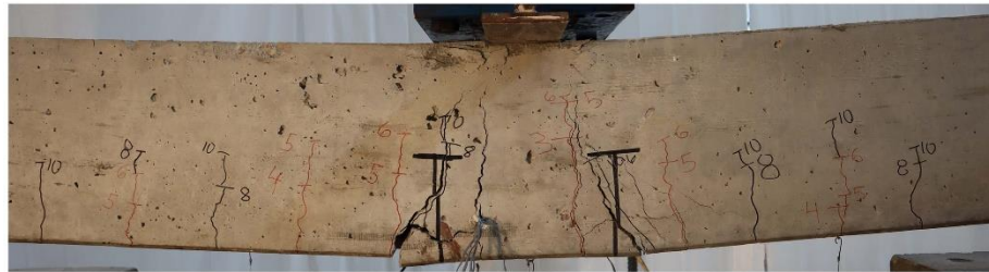
b) Widened inclined cracks at 13.8 kips
