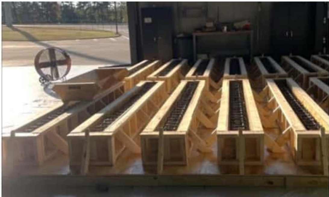
Figure 4-5 Concrete forms and sliding funnel
