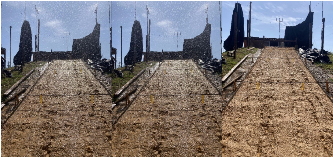
(a) during 2.0 in./hr (51 mm/hr) (b) during 4.0 in./hr (102 mm/hr) (c) after 6.0 in./hr (152 mm/hr)
