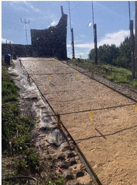
Figure 3-26: Rainfall Gauge Suspension Method
