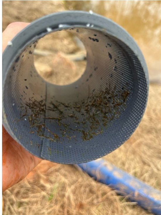
Figure 3-19: Debris Caught by Filter
