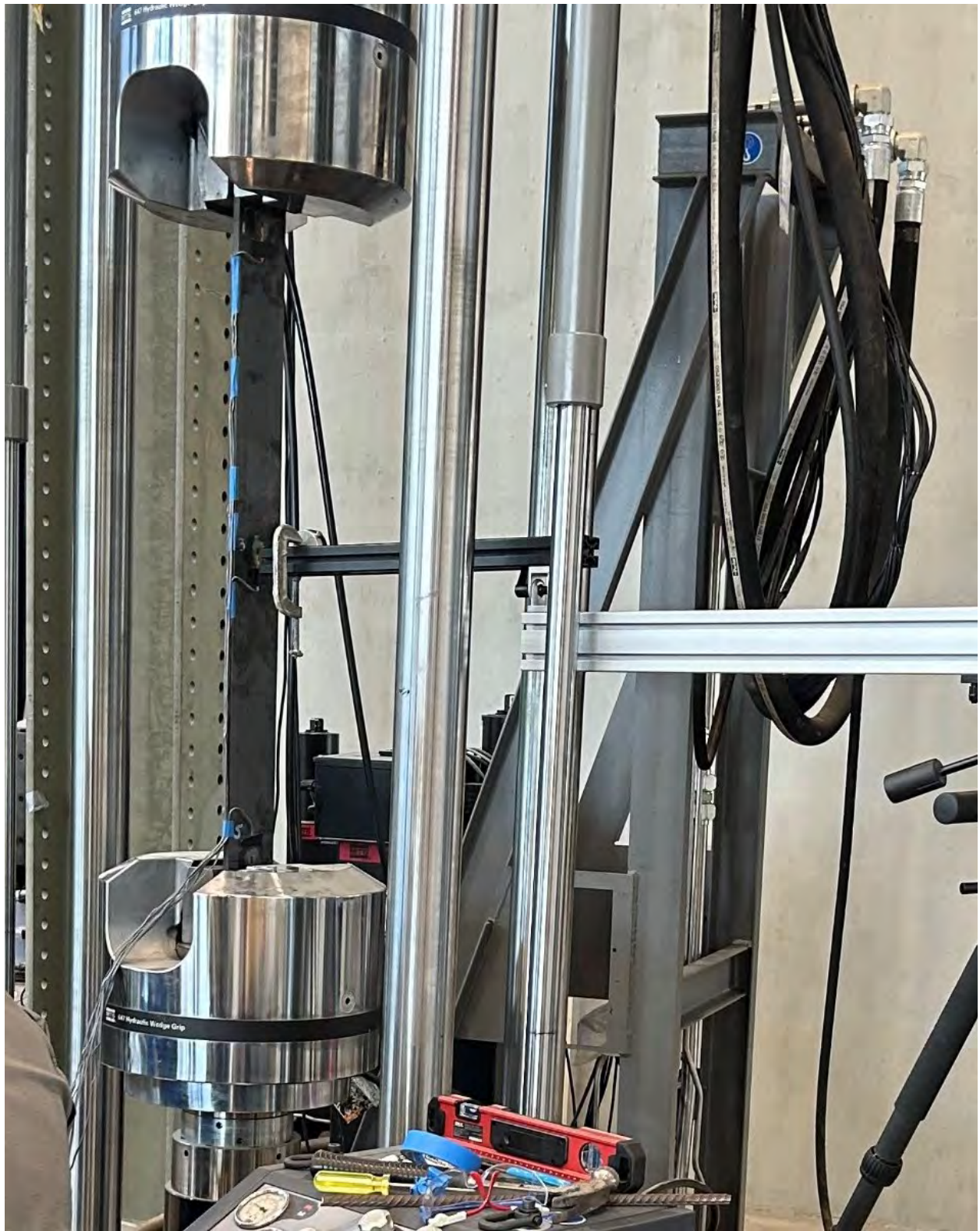
Figure 4.34: Picture of 0.5 inch thick plate during buckling test
