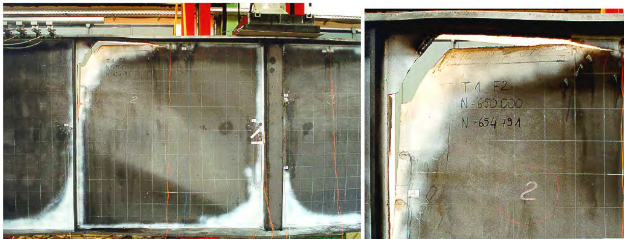
Figure 3.49: Fatigue cracks under combined loading test (Kuhlmann and Spiegelhalter 1999)
