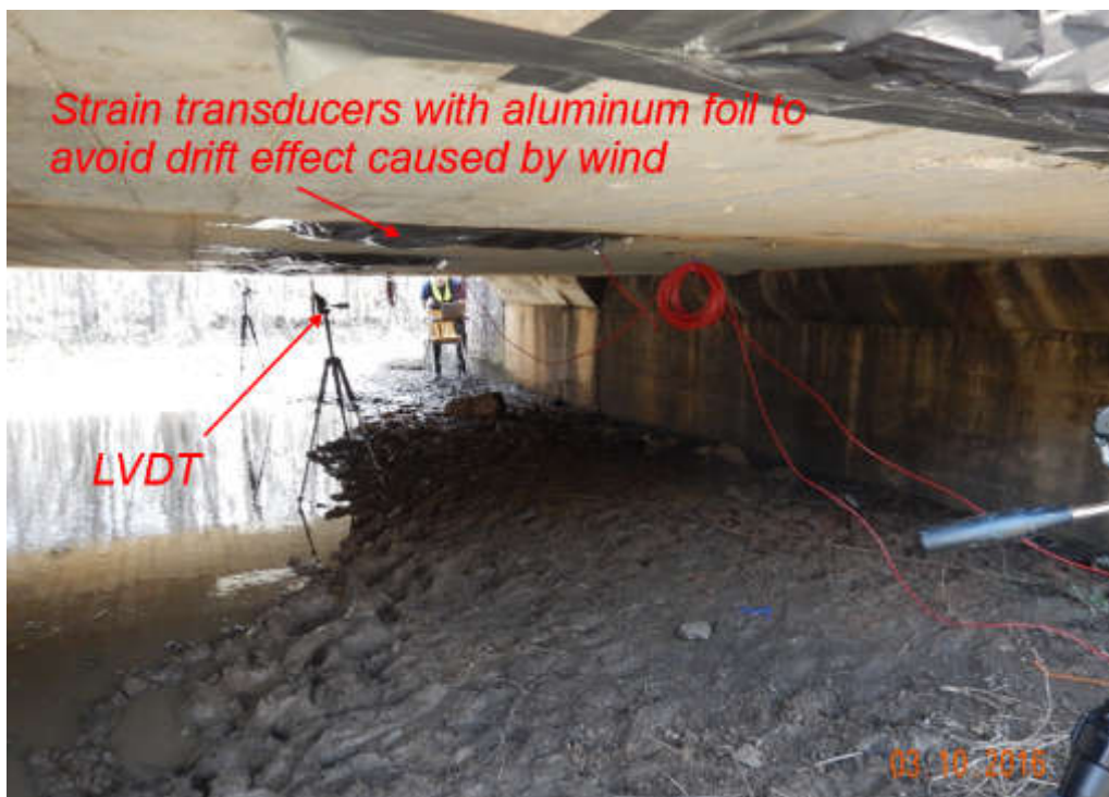
Figure 6-3: Sensors Mounted Under the Bridge (Photo by ALDOT)
