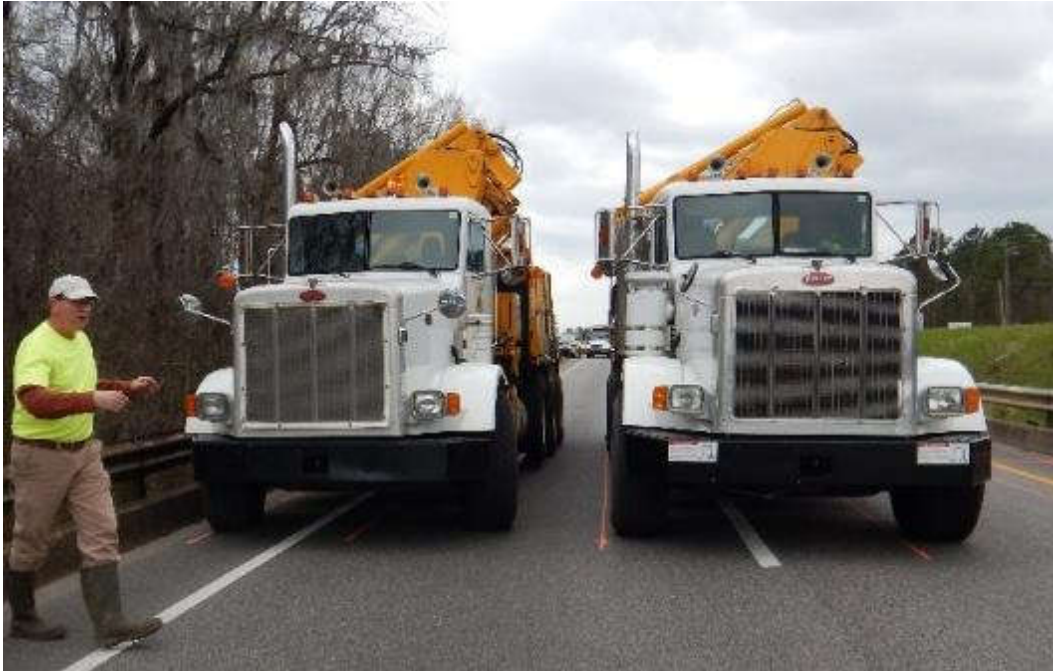
Figure 6-7: Example of Load Pattern (Photo by ALDOT)
