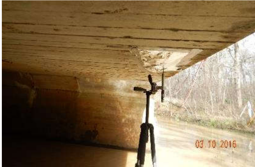
Figure 6-2: Strain Transducer Covered with Aluminum Foil and One LVDT (Photo by ALDOT)
