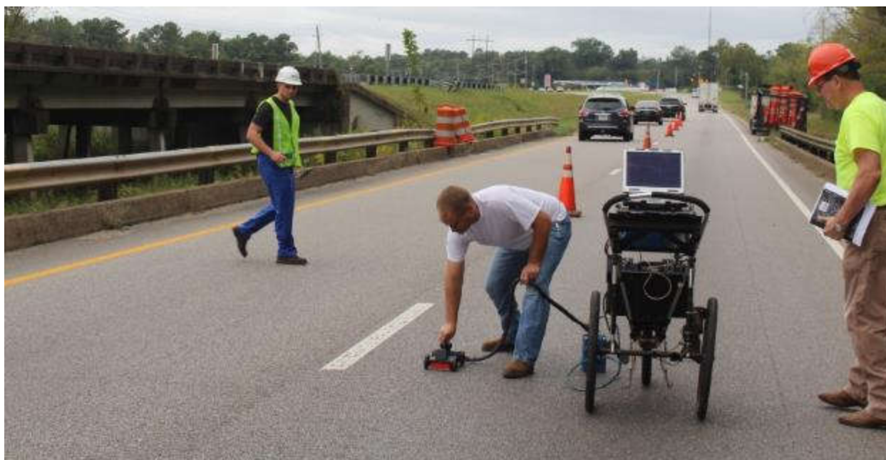
Figure 4-7: Ground Penetrating Radar Tests
