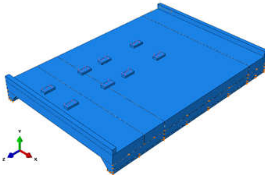
Figure 7-6: Boundary Conditions for the Bridge Model
