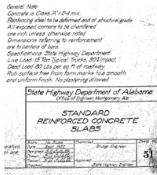
Figure 3-1: Title Block and General Notes for Standard Drawings of Simple Span Bridges (SHDA, 1922)
