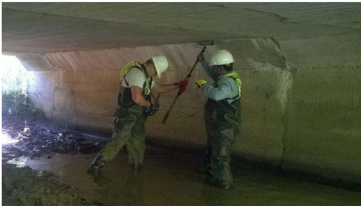
Figure 4-6: Reinforcement Detection and Measurements with Proceq Profometer
