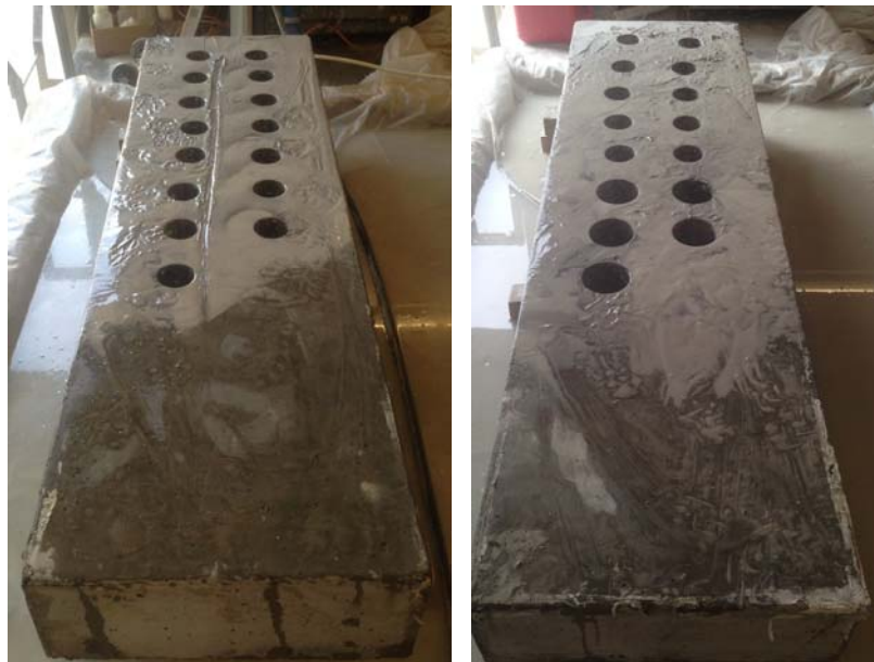
Figure 3-12: Cores taken when primarily testing 3 in. core diameters
