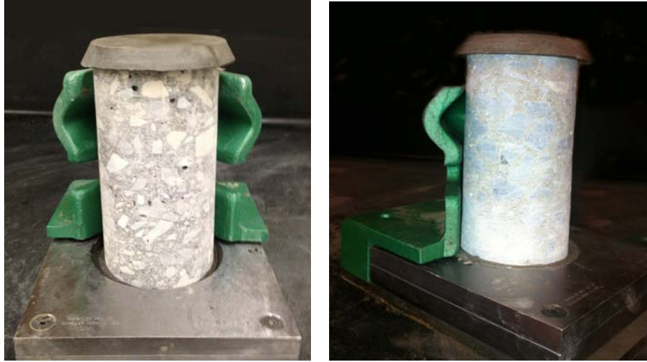
Figure 3-18: Example of sulfur capping
