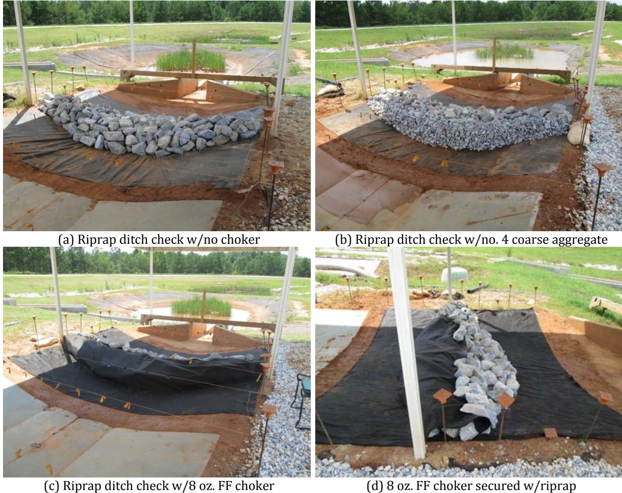
Figure 4: Riprap Ditch Check Installation Configurations
