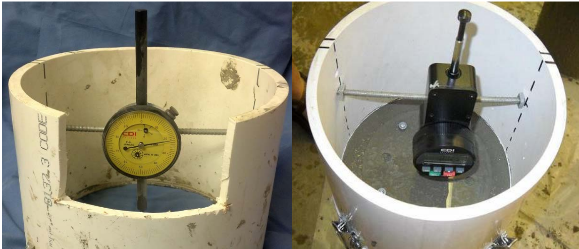
Figure 2.9: Surface settlement test equipment with (left) analog dial gauge and (right) digital indicator
