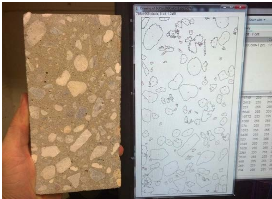
Figure 2.14: Comparison of actual specimen to digital identification of coarse aggregate
