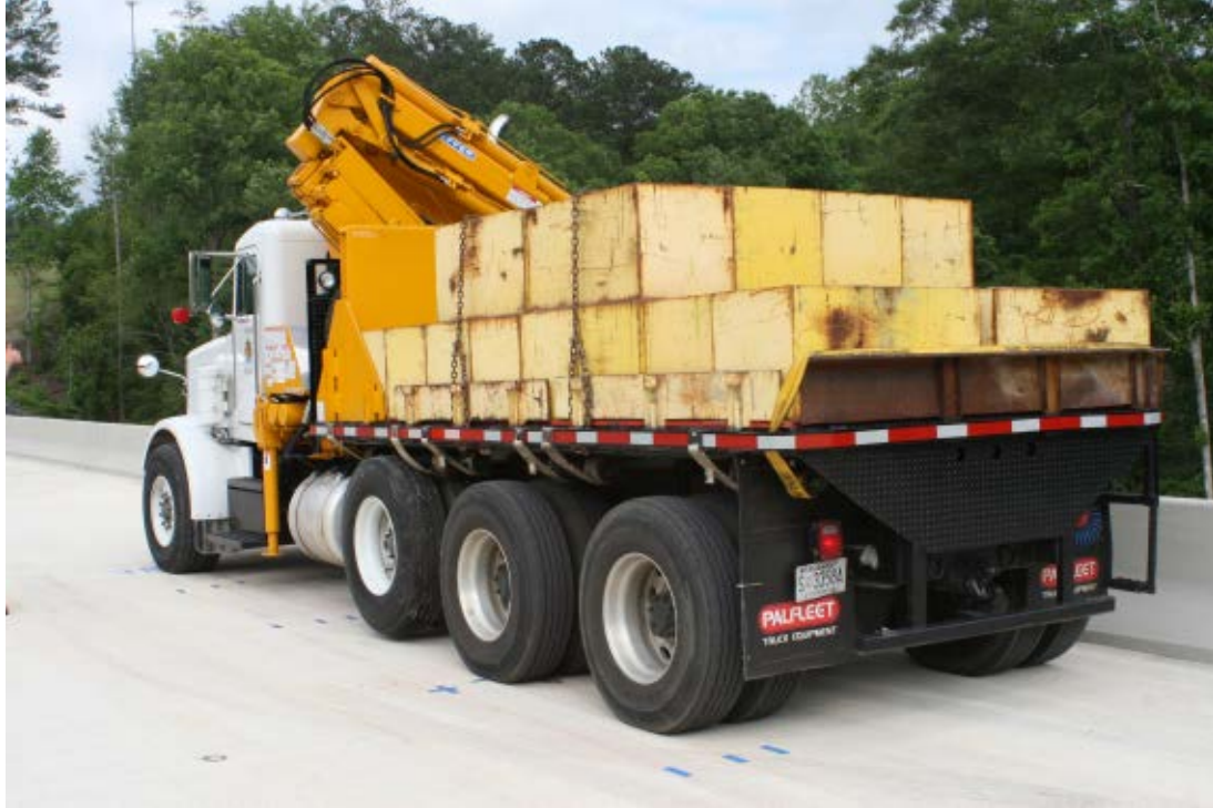
Figure 5.4: ALDOT load test truck used for this research (Note: only rear two axles of the tri-axle rear end of the vehicle are in contact with the deck)
