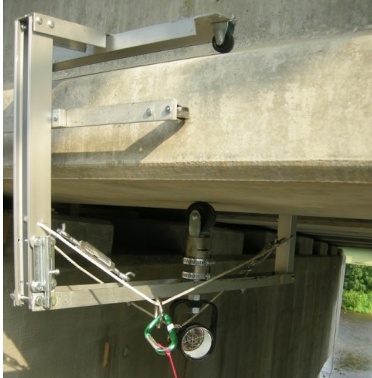
Figure 4.11: Apparatus used to survey underside of girders during construction
