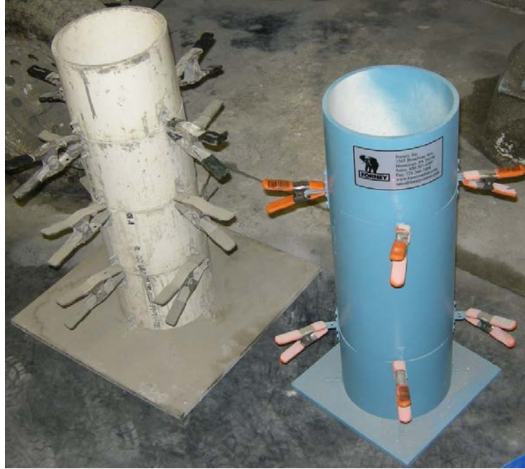
Figure 2.8: Two column segregation molds used during simultaneous testing
