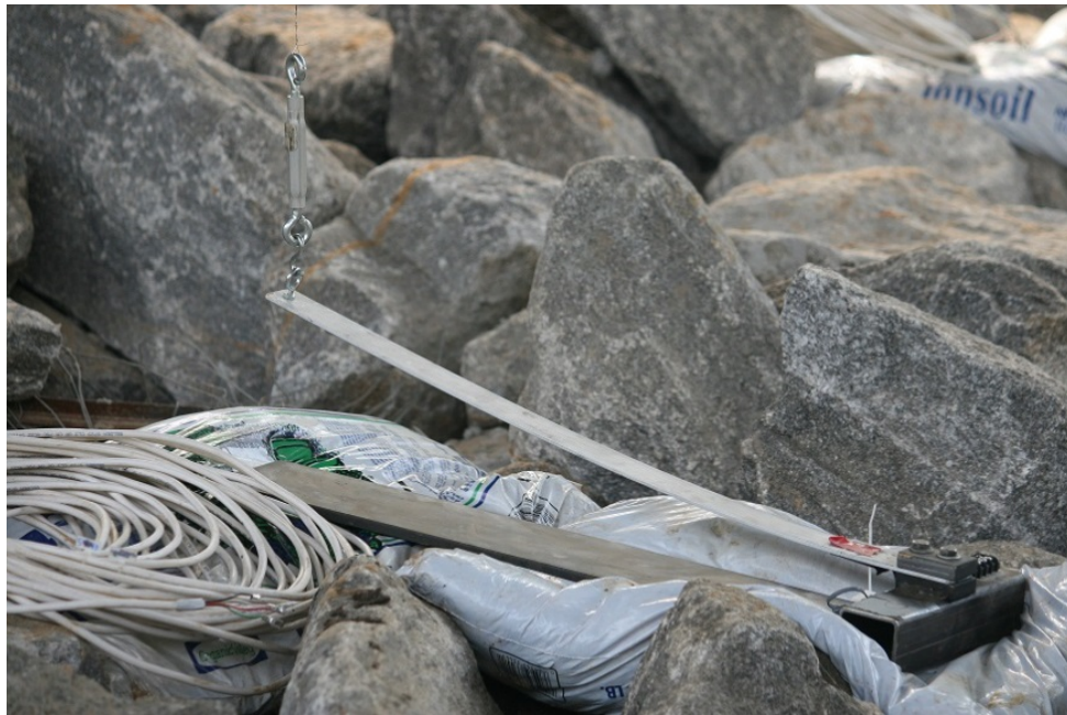
Figure 5.2: Deflectometer used to measure midspan live-load deflection
