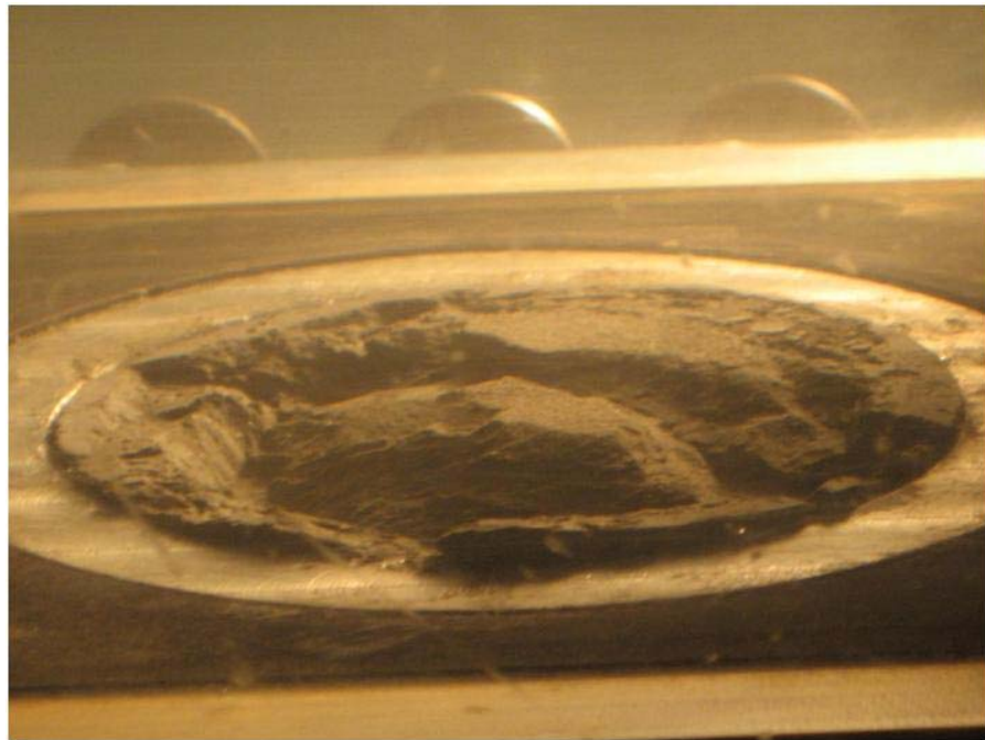
Figure C-22. Bucatunna 26.0_3 Sample Approximately 15 Minutes into 3.0 m/s EFA Test.
