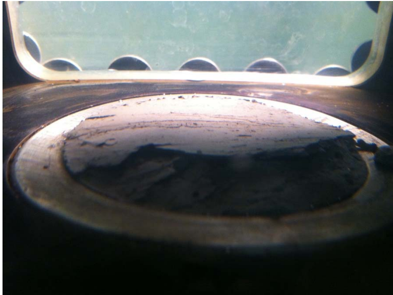
Figure B-5. Yazoo Clay 18.5_1 Test Failure Wedge
