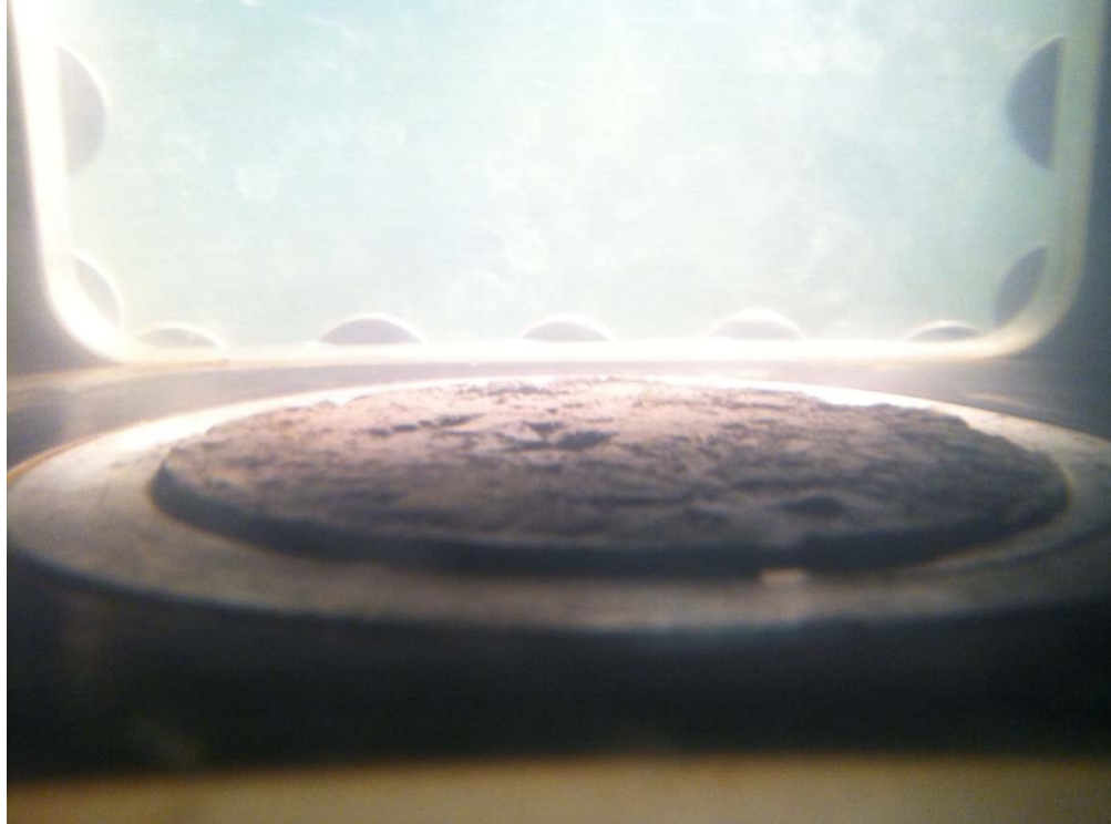
Figure 2-11. Soil Sample in EFA Advanced 1 mm.
