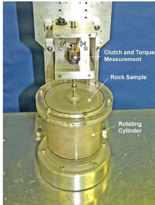
Figure A-4. Rotating Erosion Test Apparatus (RETA)
