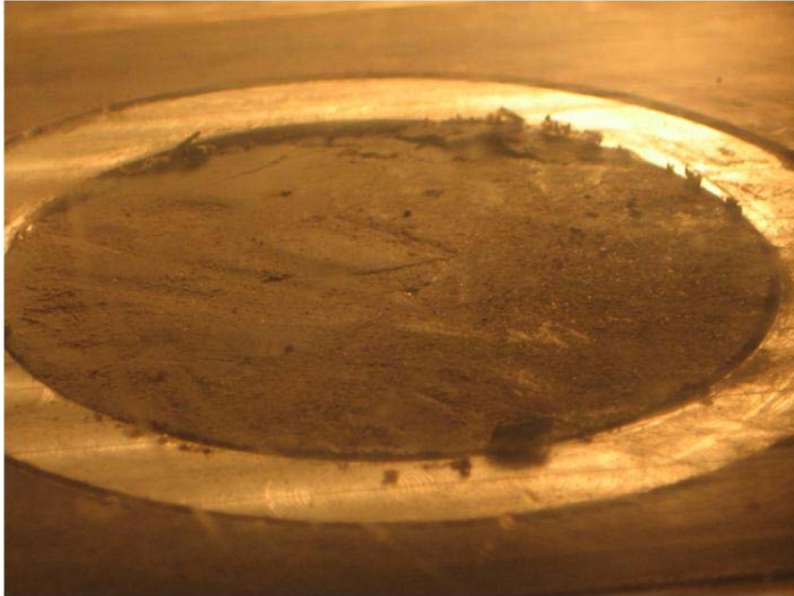
Figure C-9. Naheola Clay 16.0_1 Sample Prior to 1.5 m/s EFA Test.
