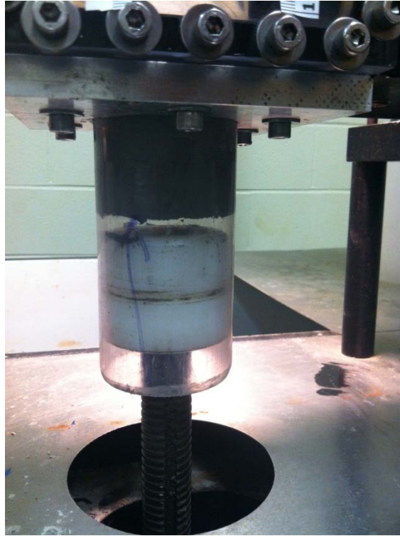
Figure 2-9. Soil Plunger Advancing Sample.
