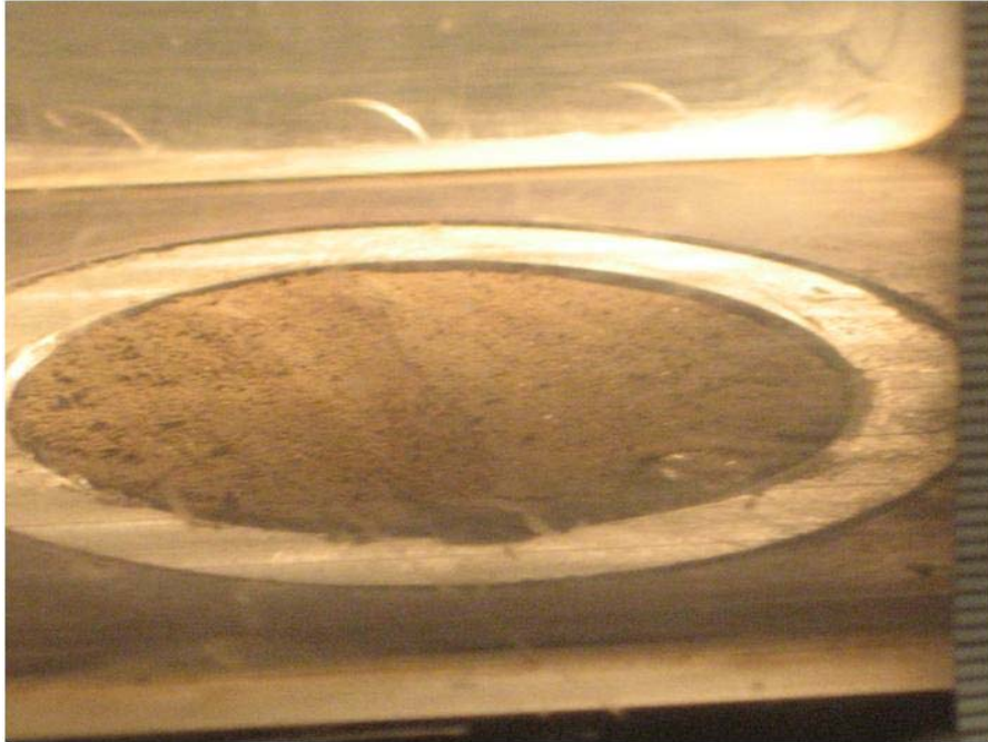
Figure C-6. Naheola Clay 17.2_1 Sample Prior to 2.0 m/s EFA Test.
