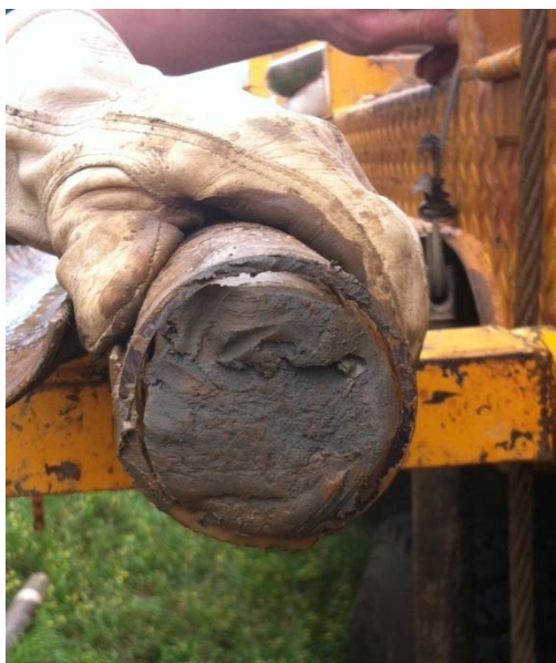
Figure B-1. Bucatunna Clay Sample Smaller Radially than Sample Tube
