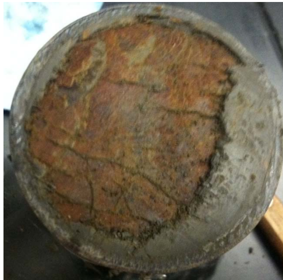
Figure B-19. Porter's Creek Clay Formation Scoured along Weathered Planes
