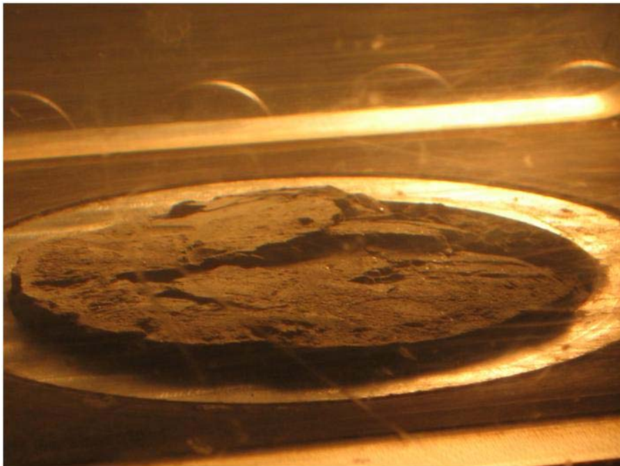
Figure C-10. Naheola Clay 16.0_1 Sample at the End of 1.5 m/s EFA Test.
