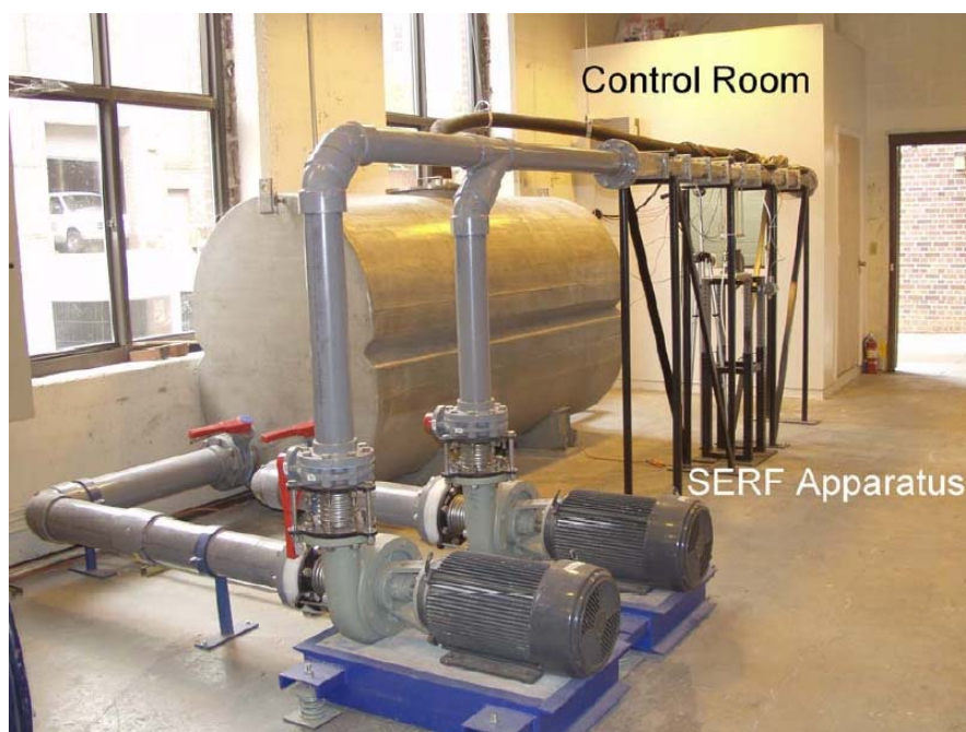
Figure A-5. Sediment Erosion Rate Flume (SERF)
