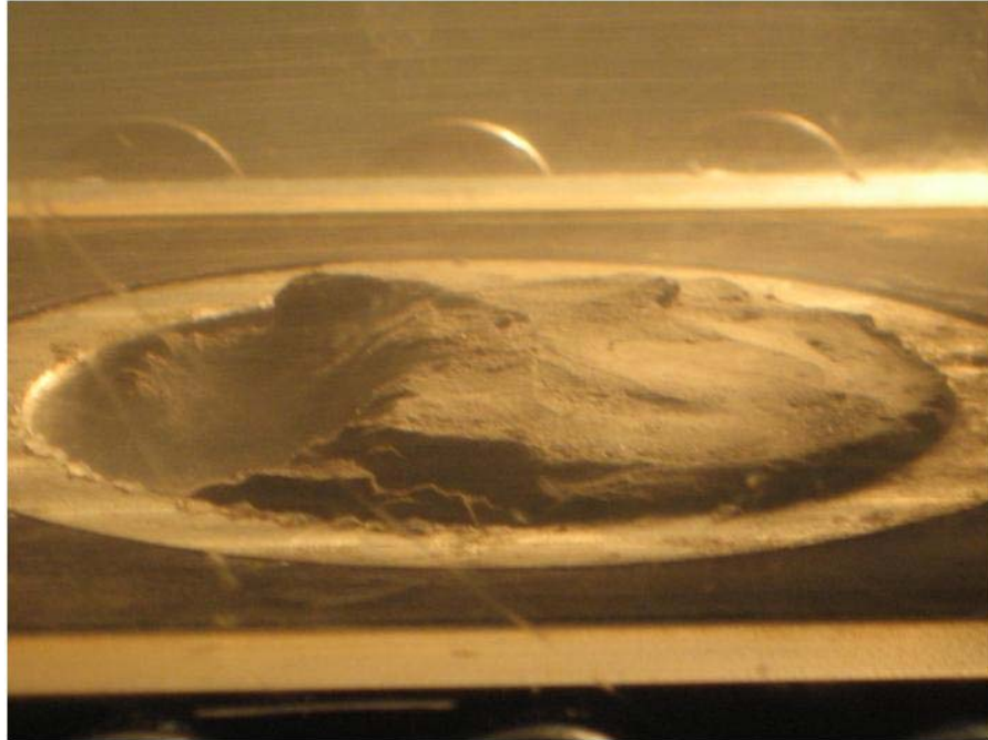
Figure C-13. Naheola Clay 19.5_4 Sample at the End of 2.0 m/s EFA Test.
