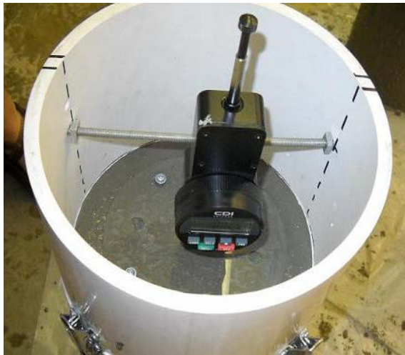
Figure 2.19: Surface settlement test equipment with digital indicator
