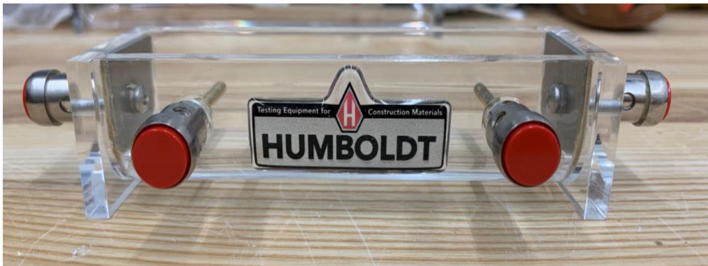
Figure 2-5: Soil box used for resistivity testing in the laboratory.
