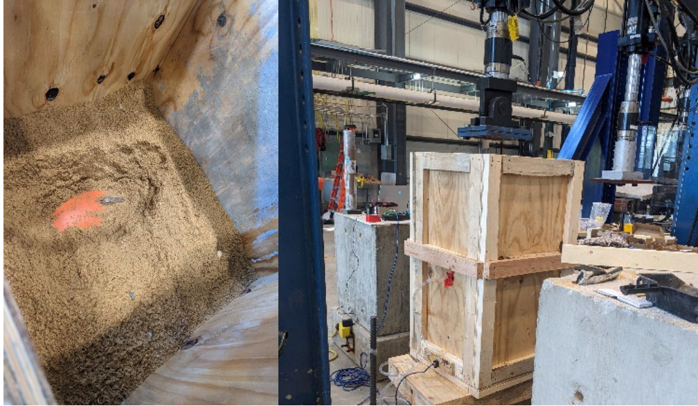
Figure 50. Setup for the sandbox testing for the air bladders.
