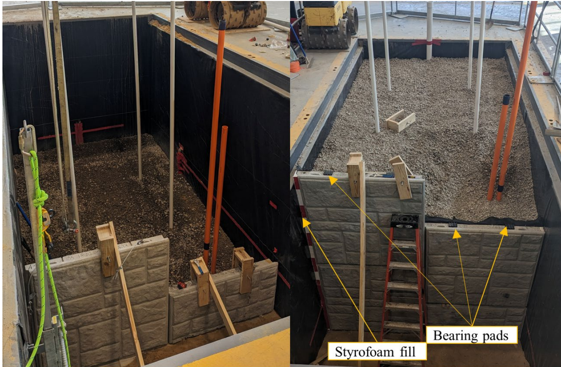
Figure 143. (left) first row of panels placed with external bracing and wedge. (right) second row of panels placed with external bracing and wedge.
