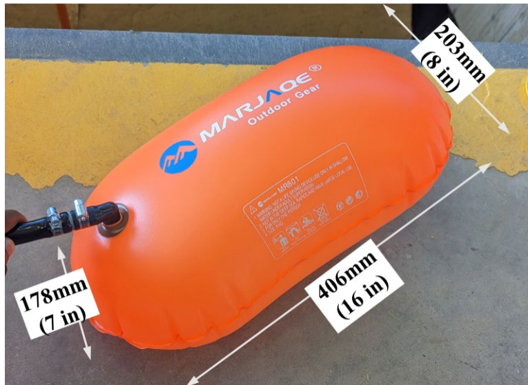
Figure 49. Inflated air bladder used for simulating zone of soft soil in foundation.
