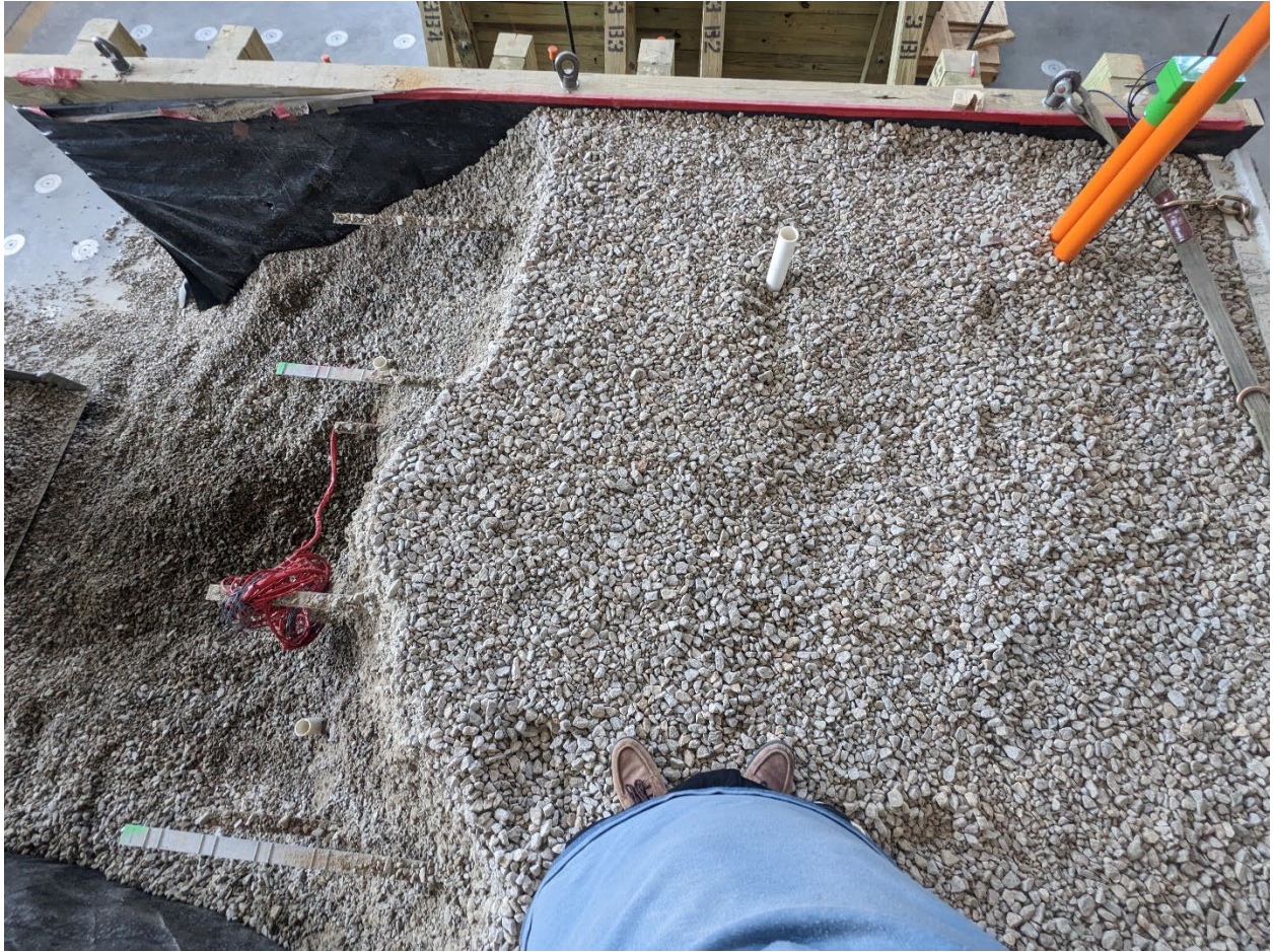
Figure 147. Apparent confinement effect resulting in near vertical face of the granular backfill during dismantling.
