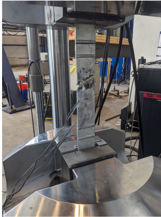
Figure 53. Failed steel specimen in the MTS tensile test setup.
