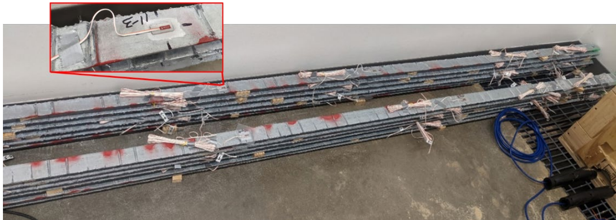
Figure 52. Strain gage installation on reinforcement straps.
