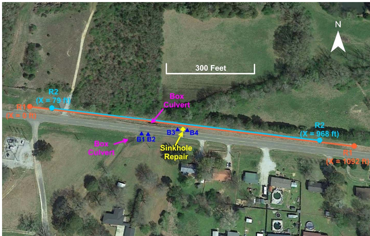
Figure 4-15: Site map with locations of resistivity lines, sinkhole repair and approximate locations of boreholes in Centreville.
