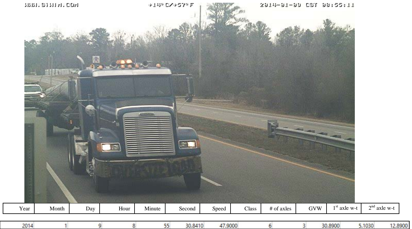
Figure 97: The example of vehicle of Class 6 (subtype A – 3 axles, GVW – 31.59 kips) 2014
