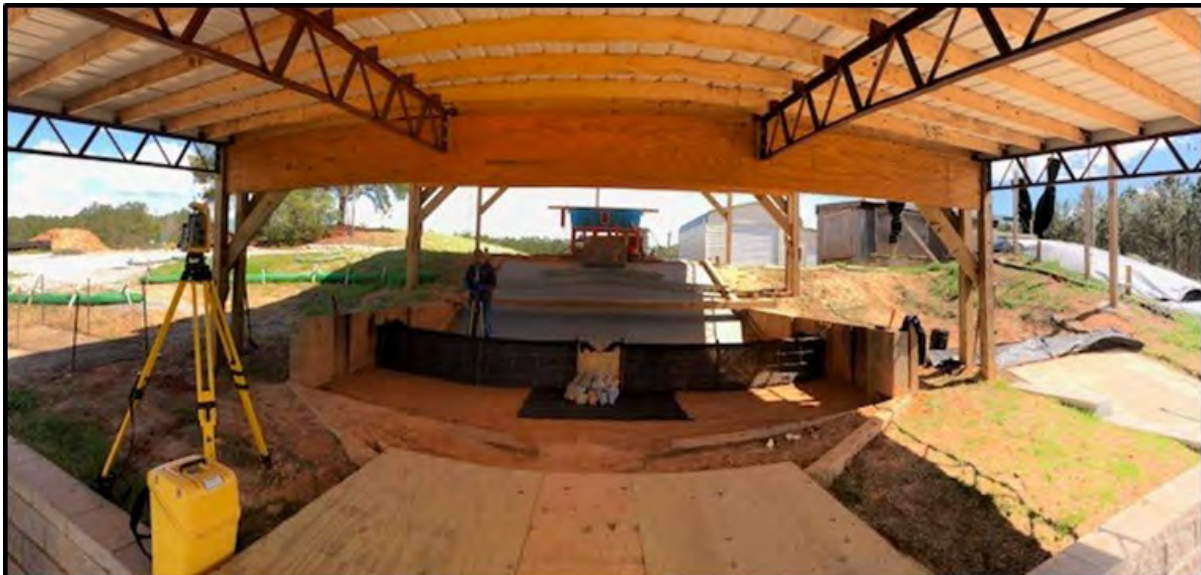
Figure 11. Robotic total station setup and survey.
