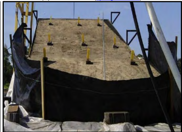
(d) tilting test bed with rainfall simulator ( Gogo-Abite and Chopra 2013 )
