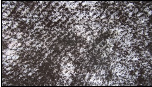
(a) nonwoven - needle punched
