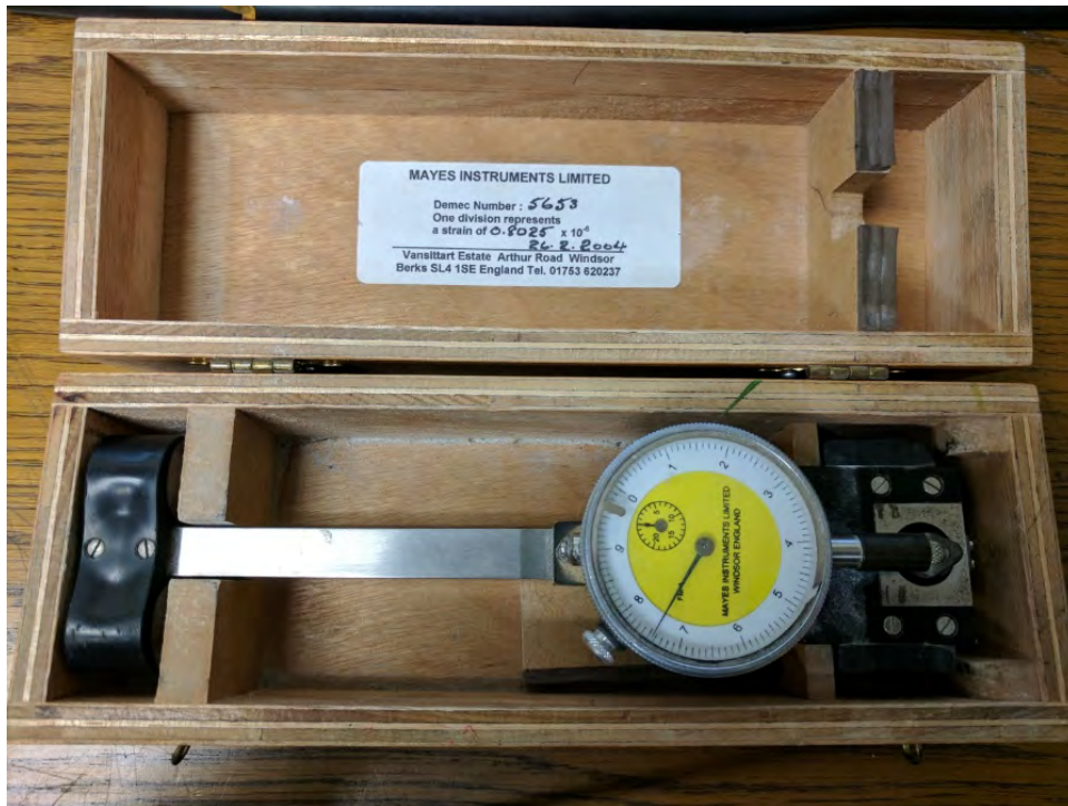
Figure 4-5. Mayes demountable mechanical concrete strain gauge (DEMEC)
