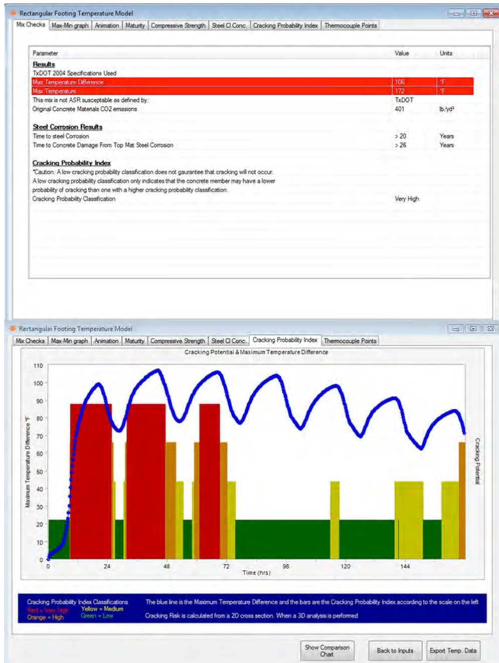
Figure 2-17: Example ConcreteWorks output summary (top) and \Delta T /cracking risk profile (bottom)
