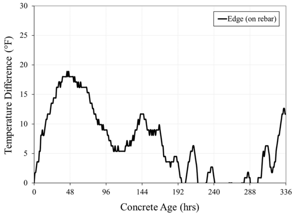
Figure 5-32: Birmingham column 14-day temperature difference data
