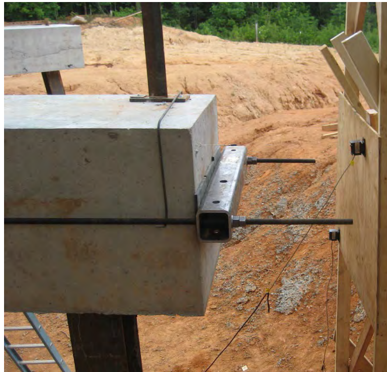
Figure 8-5 – High Strength Threaded Rod and HSS Bearing Tube
