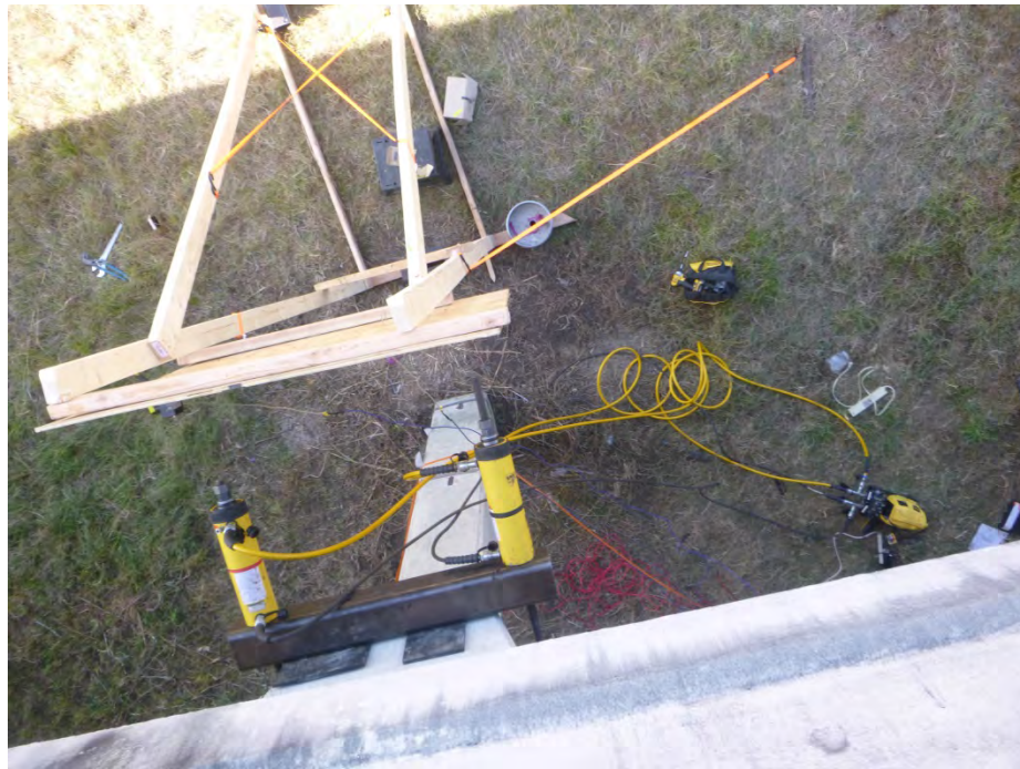
Figure 6-5 Hydraulic Cylinders and Pump Seen From Bridge Deck
