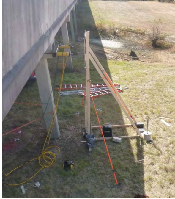
Figure 6-8 Wooden Reference Frame for Wirepots
