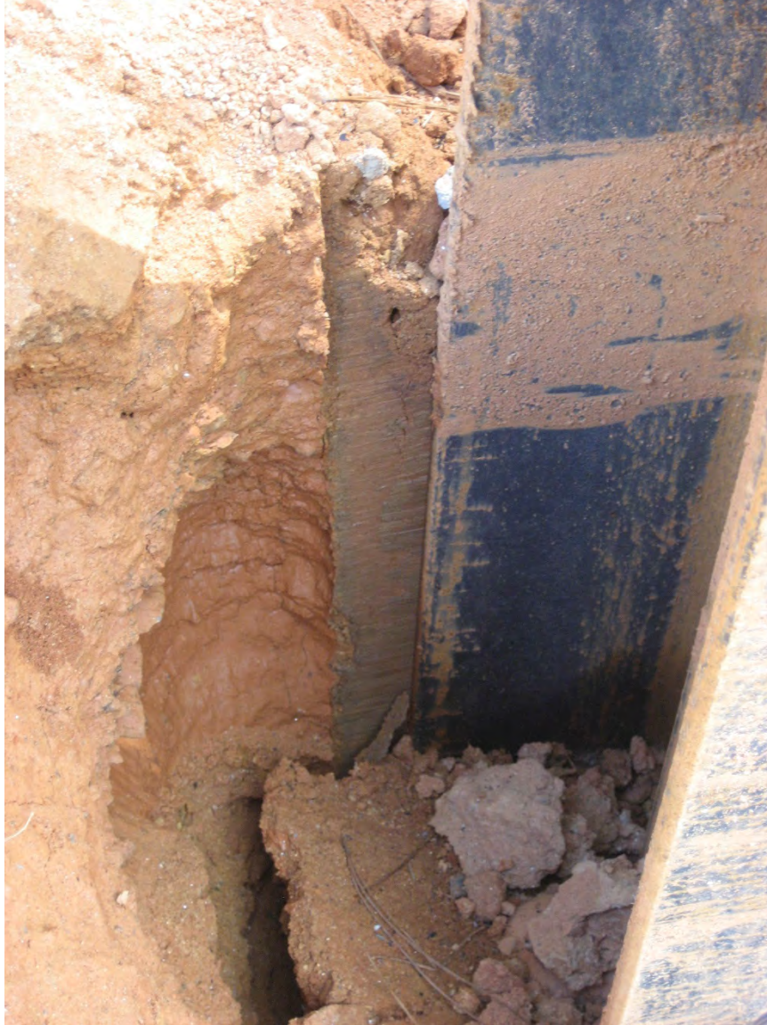
Figure 8-19 – Lateral Displacement of Test Pile
