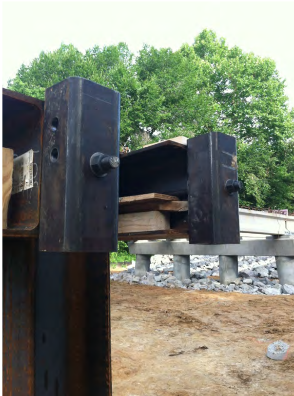
Figure 4-9 Threaded Rod End Anchorage at Reaction Frame
