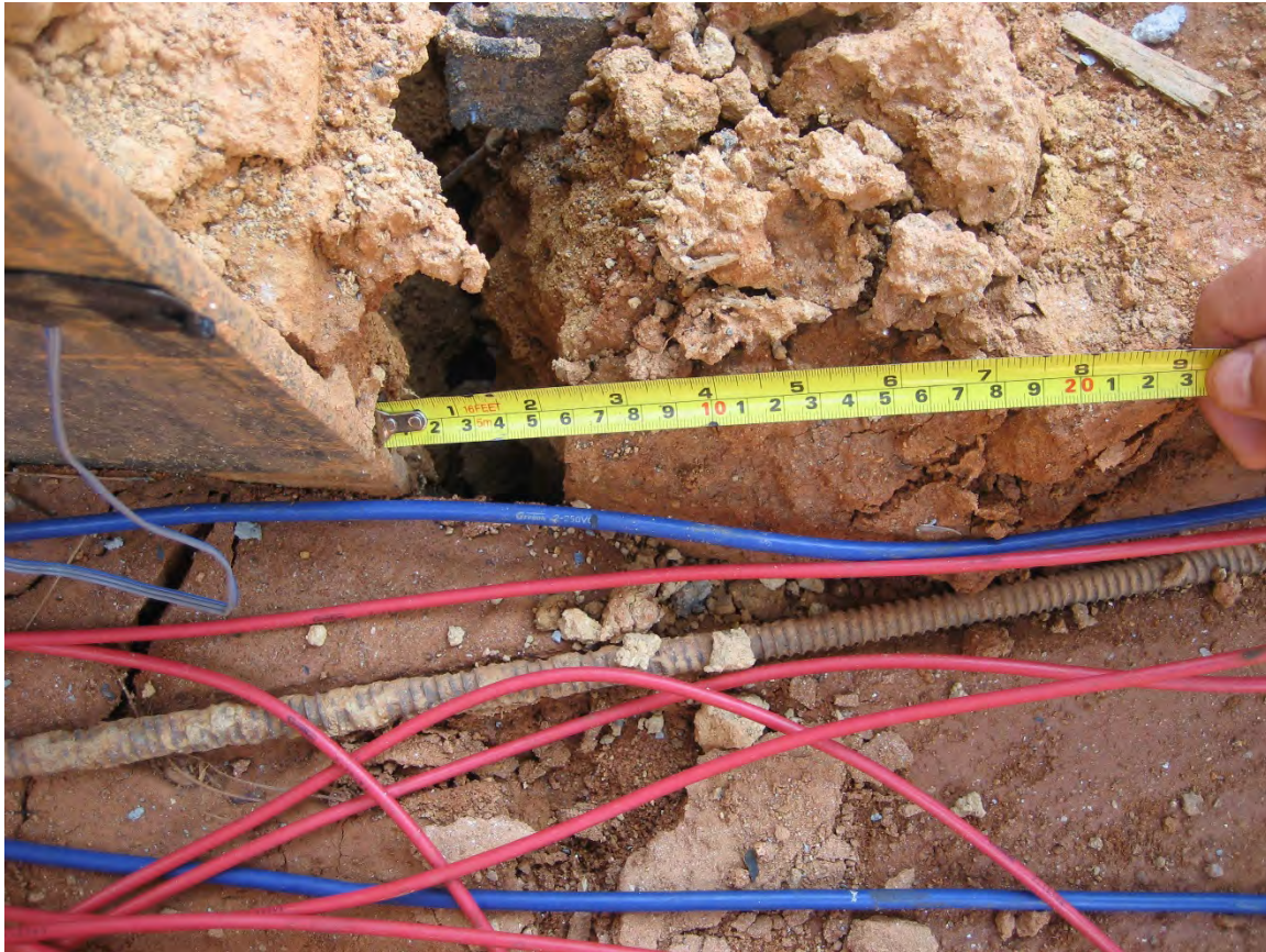
Figure 8-10 – Residual Drift due to Lateral Load Test
