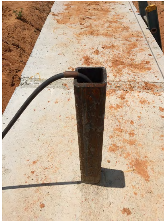
Figure 8-4 – Inclinometer Downhole at Pile 2
