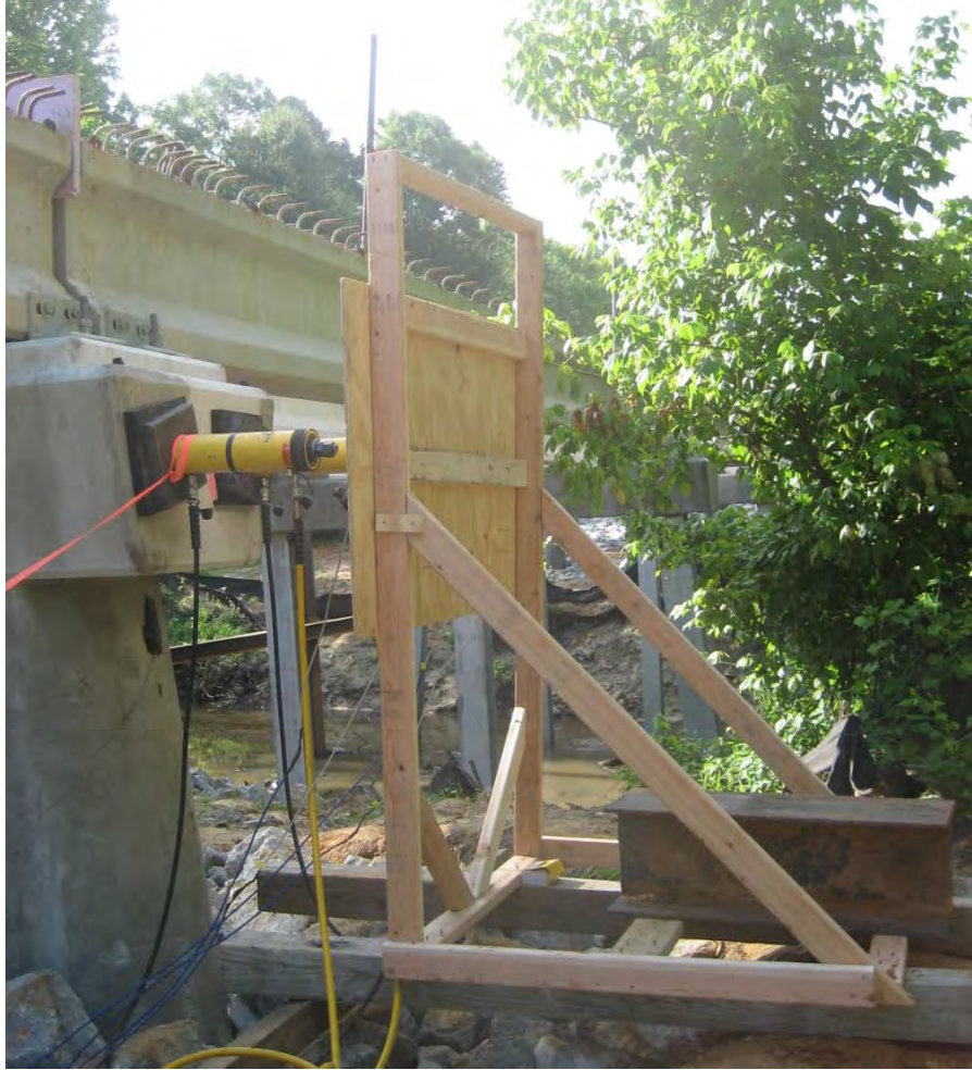
Figure 4-11 Wooden Reference Frame for Wirepot Installation
