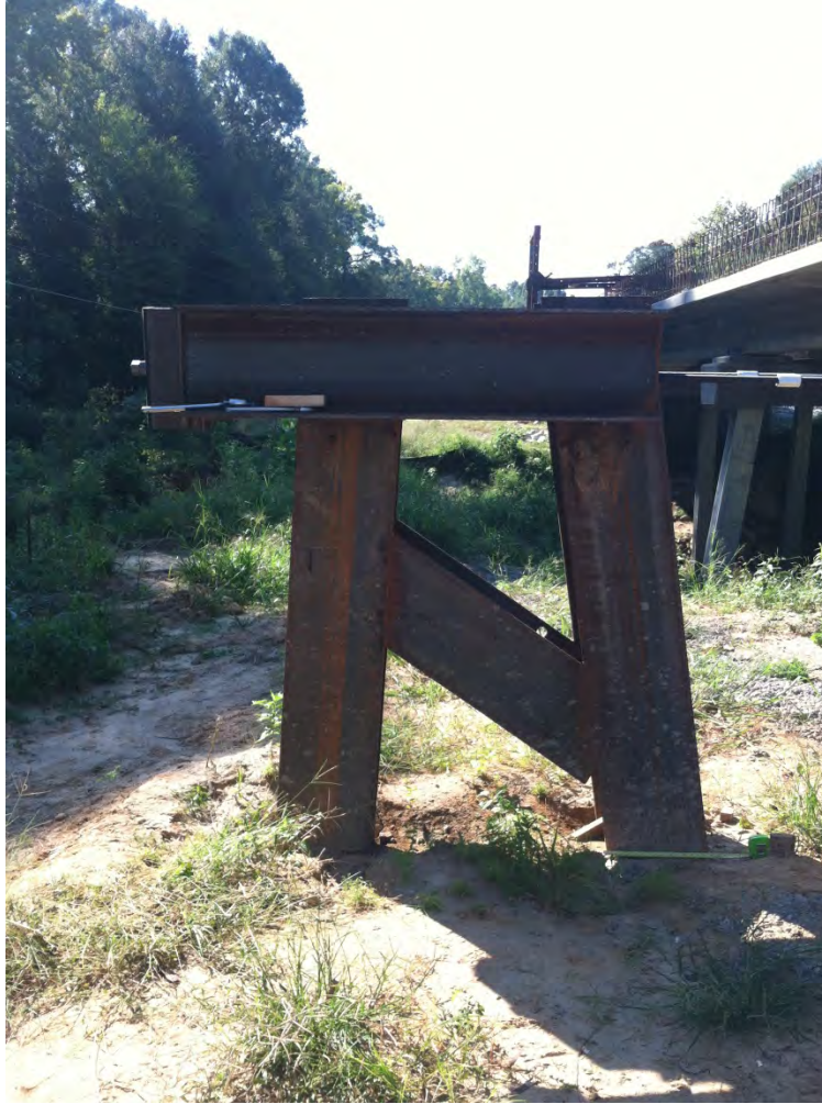
Figure 4-8 Reaction Frame Configuration
