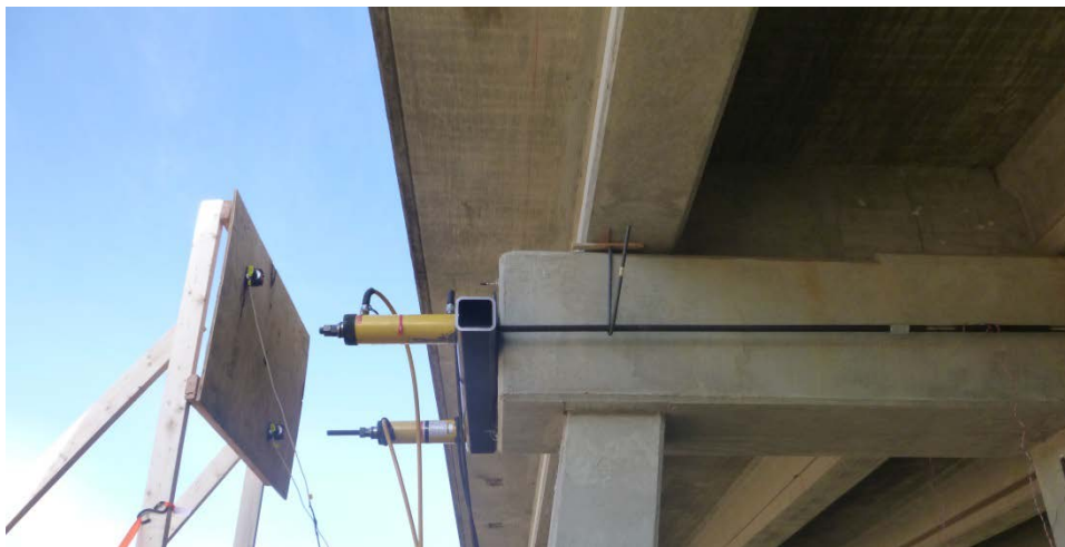
Figure 6-7 Threaded Rods Anchored on Jack End
