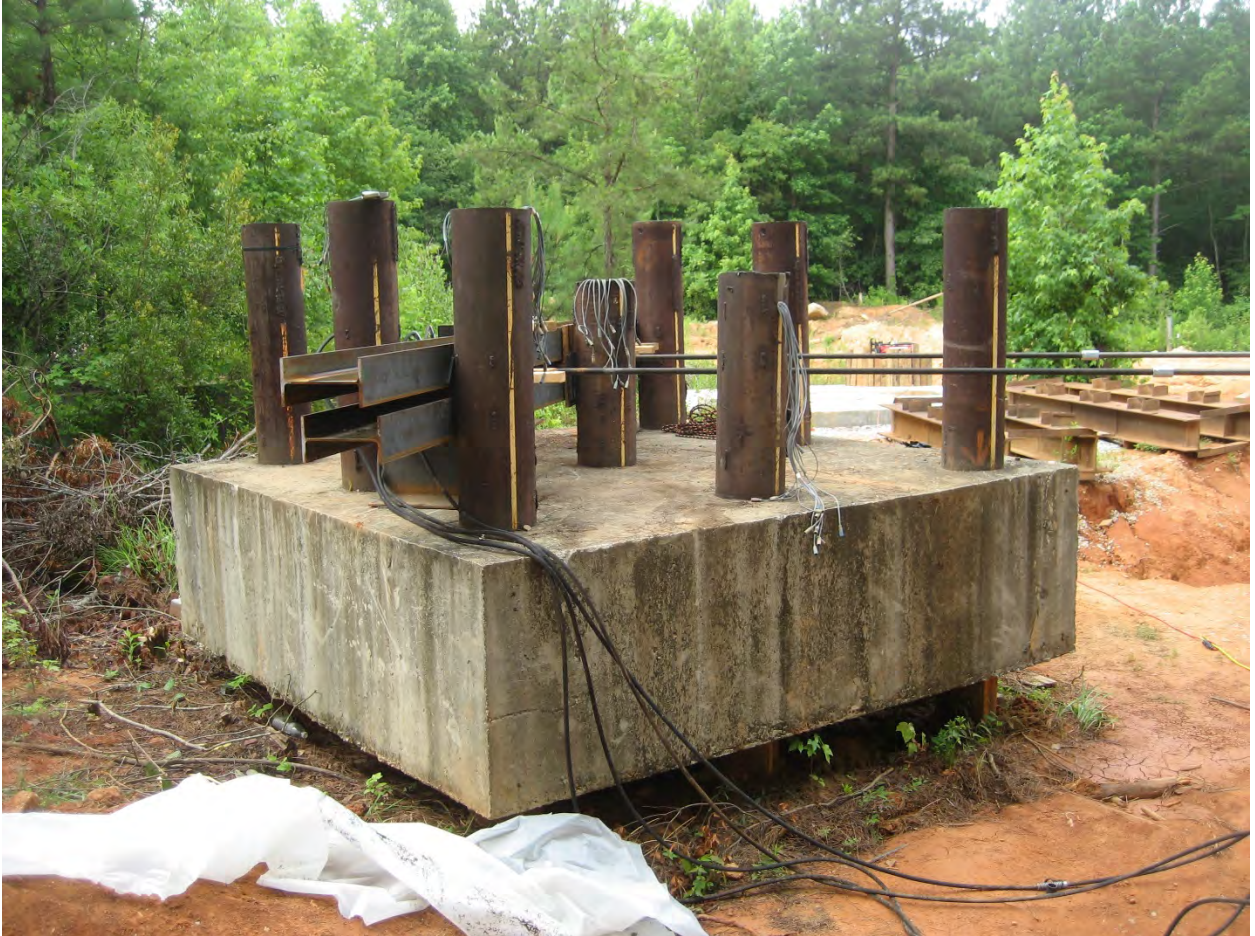
Figure 8-6 – Reaction Pile Group with W10x23 Load Beams
