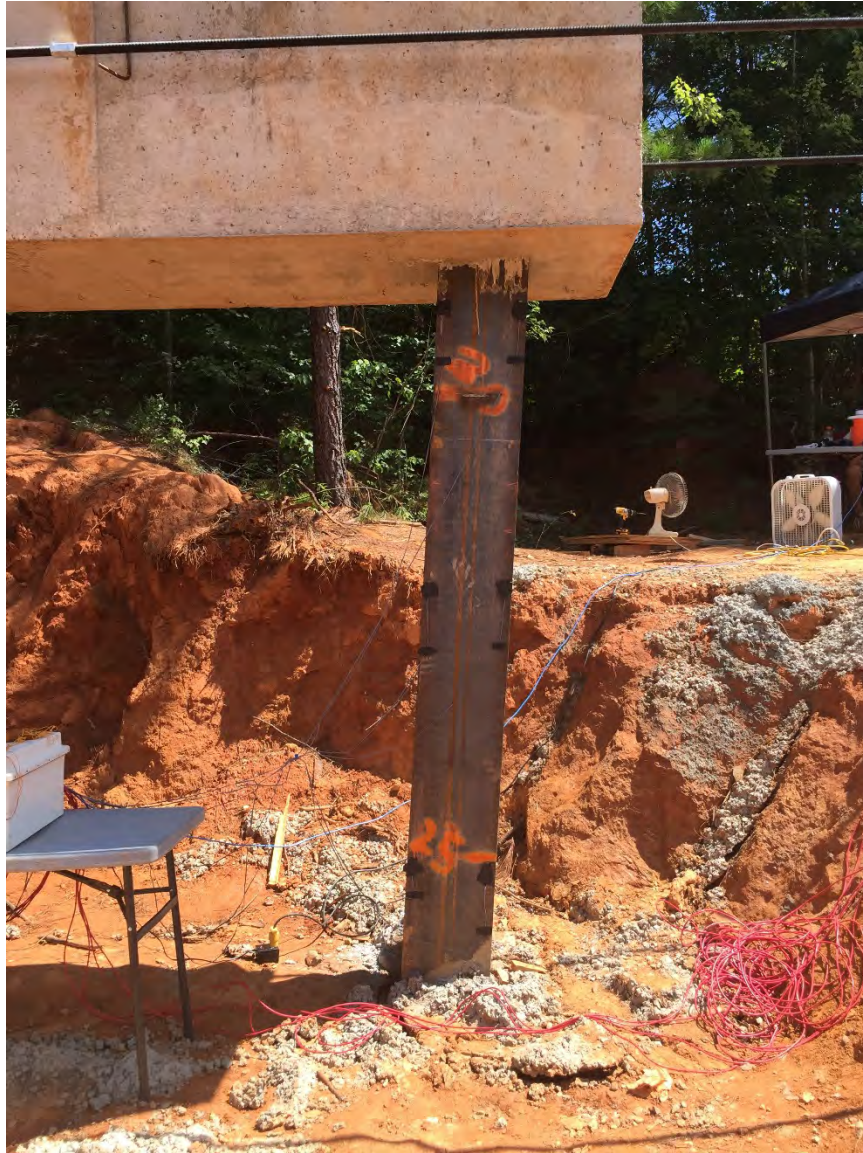
Figure 8-15 – Lateral Deflection Induced in Pile 5 during Field Load Testing
