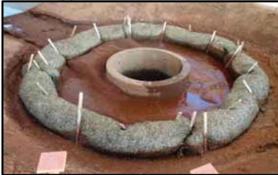
(c) ALDOT standard installation deposition
