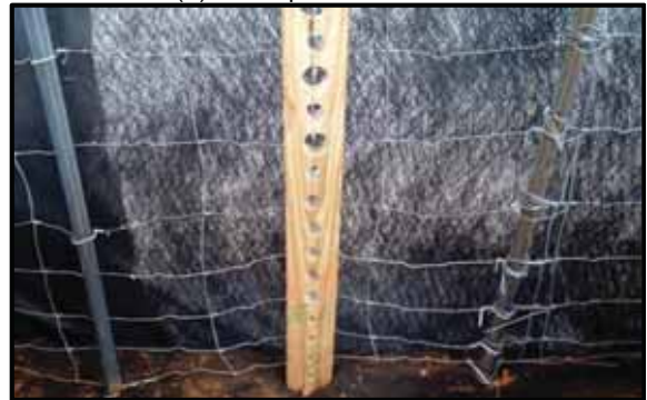
(f) MFE-I dewatering board
