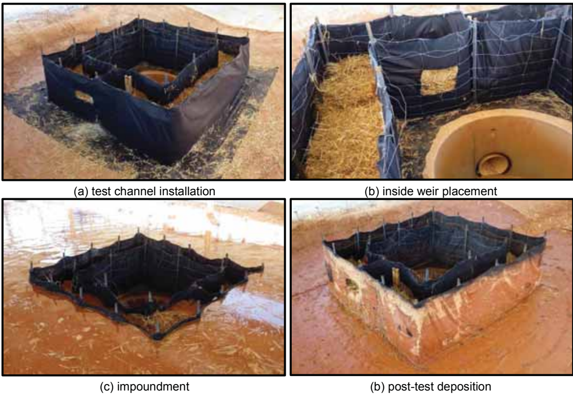
Figure 5.12 Hay Bale Flow Through System.
