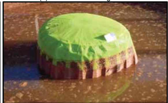
(f) round dome with add'l aggregate disfigurement
