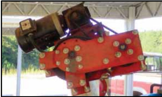
(c) motor, gearbox, sprockets, and chain
