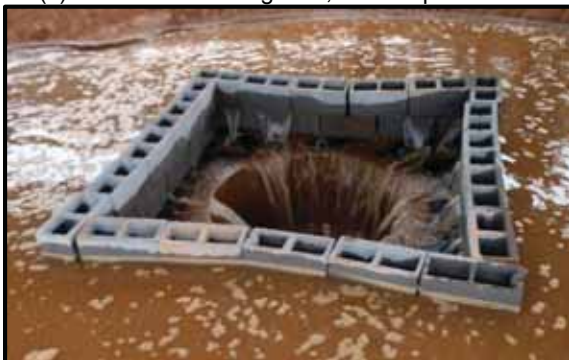
(e) block, no gravel, barrier deflection
