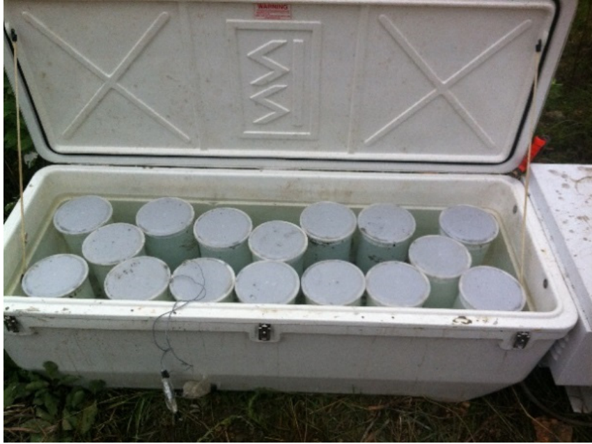
Figure 3-11: Initial Curing of Molded Cylinders
