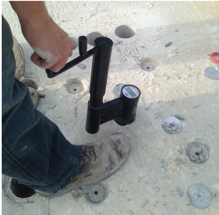
Figure 3-15: Pullout Test Being Performed
