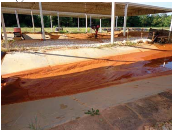
(e) large particles deposited at channel head
