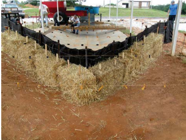
(a) hay bale dissipater pretest
