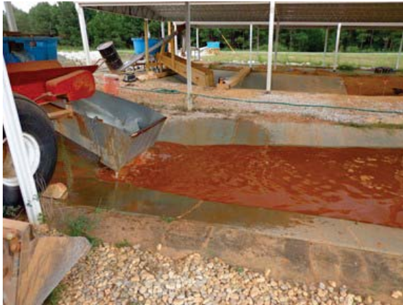
(a) introduction of sediment-laden water
