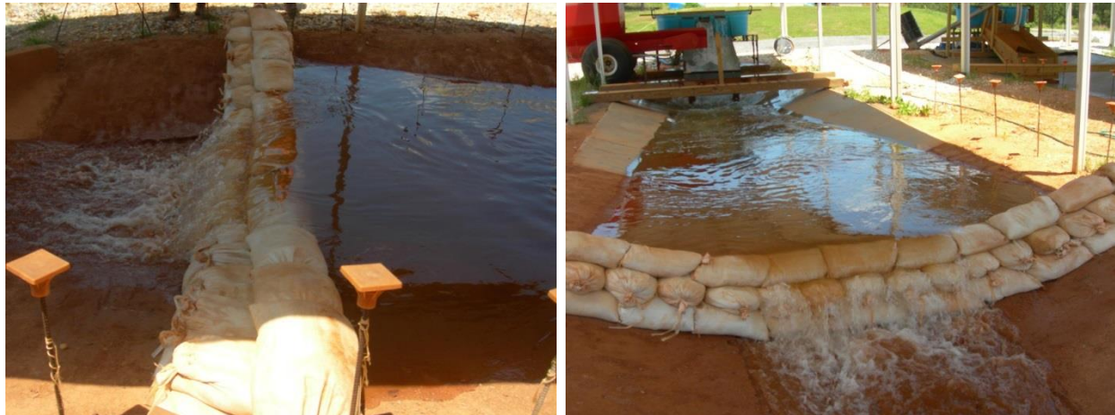
(a) top sand bag layer perpendicular to flow
