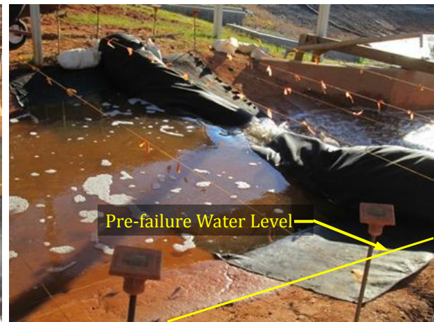
(b) failure at 1.68 cfs
