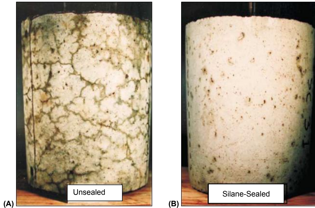
Figure 2-12: (A) Unsealed and (B) silane-sealed air-entrained concrete cylinders subjected to exposure cycle C4, after 1.5 years (Adapted from Bérubé et al. 2002a)
