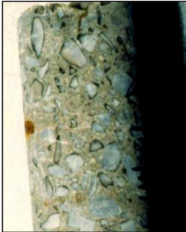
Figure 2-7: Dark rim around the perimeter of reactive aggregate particles (Fournier et al. 2010)
