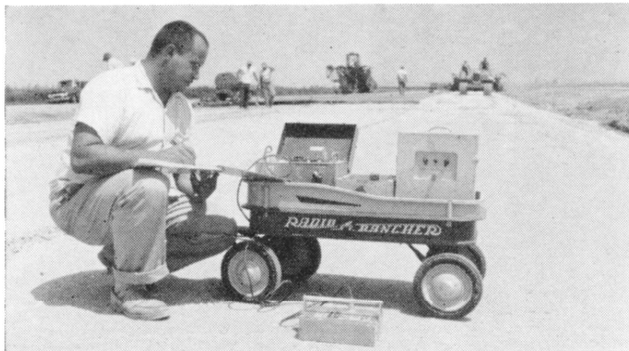
Figure 43. Nuclear density measuring device, used primarily on crushed stone base course. HRB, 1962
