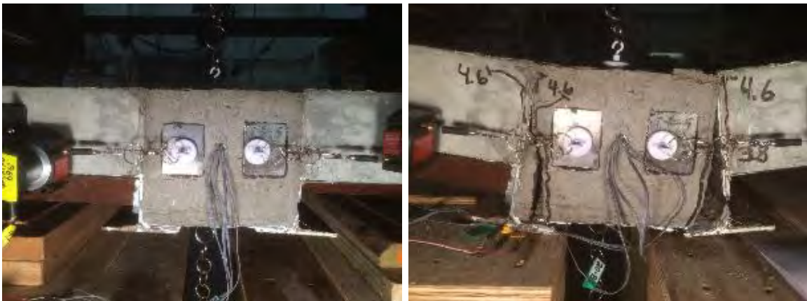
Figure 5.20 R-REV-Q Joint Before and After Test
