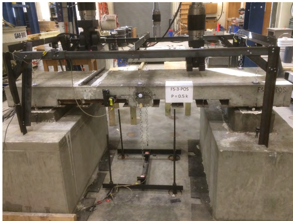
Figure 3.21 Wire Potentiometer Deflection Frame
