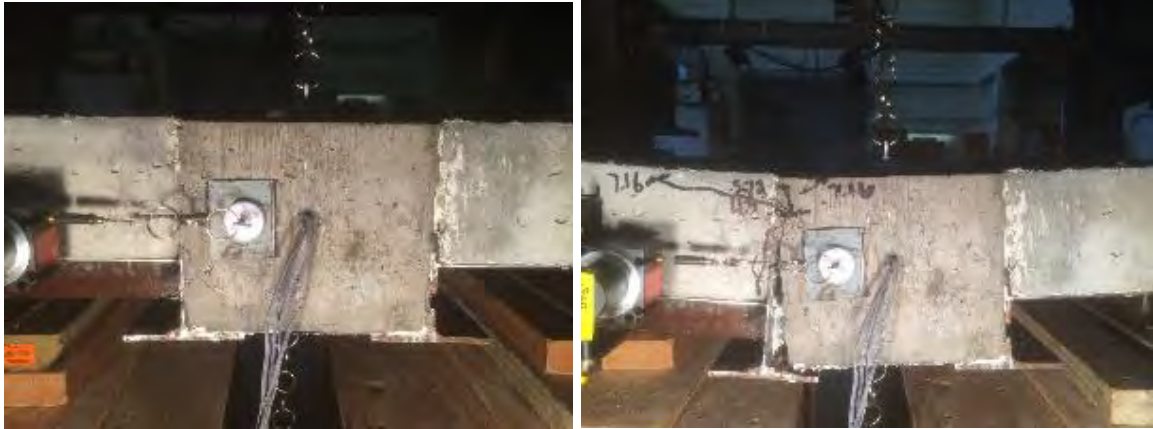
Figure 5.4 R-POS-Q Joint Before and After Test
