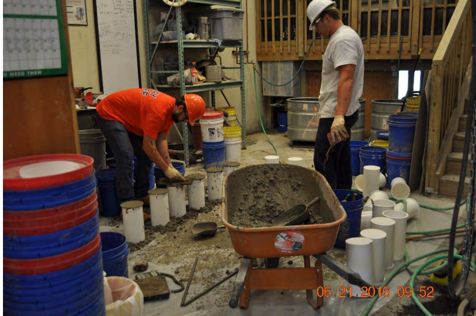
Figure 4.20 Material Testing of Deck Concrete
