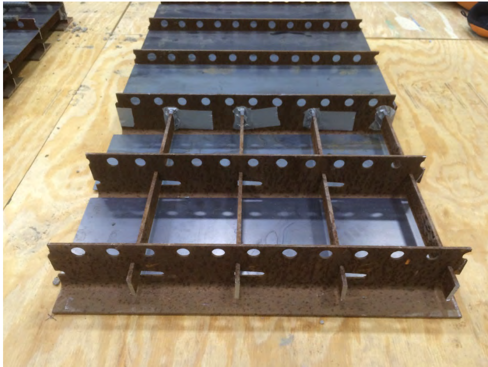
Figure 4.10 Taping Slotted Holes in Steel Grid
