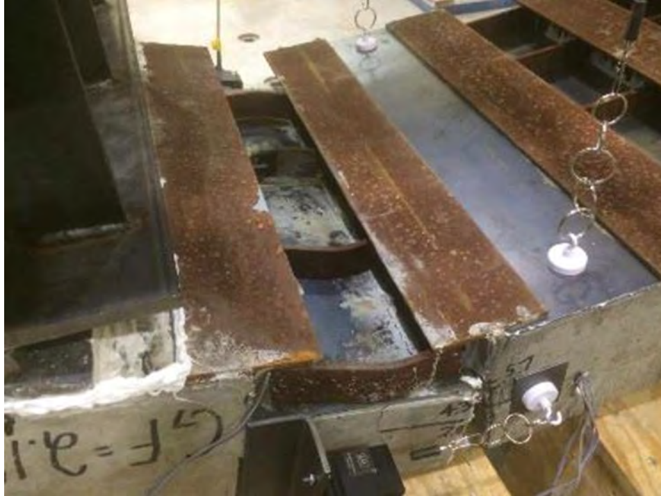
Figure 5.12 R-NEG-Q Buckled Distribution Bars (Inverted Specimen)
