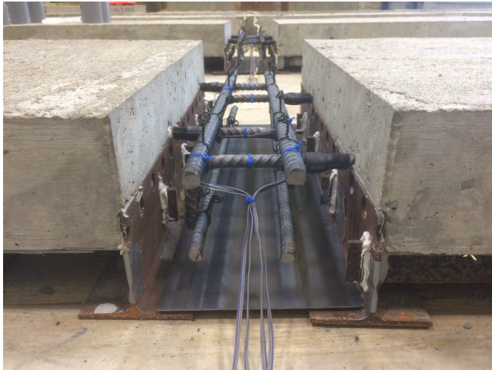
Figure 4.27 Protected ERSGs Mounted on Reinforcing Steel
