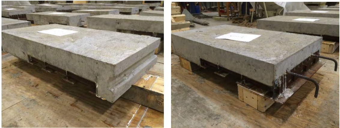
Figure 4.22 Unreinforced Shear Key Joint and Staggered Hook Reinforced Joint Panels with Forms Removed
