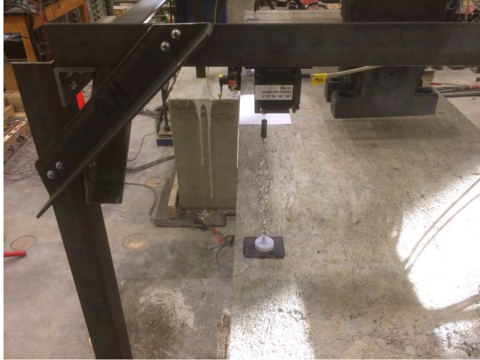
Figure 3.22 Top Wire Potentiometer Set-Up
