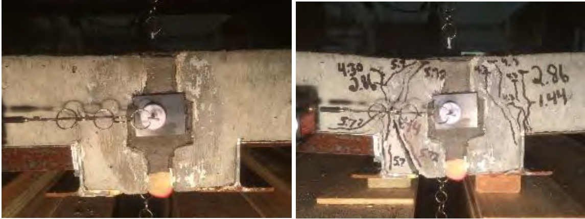
Figure 5.1 U-POS-Q Joint Before and After Test
