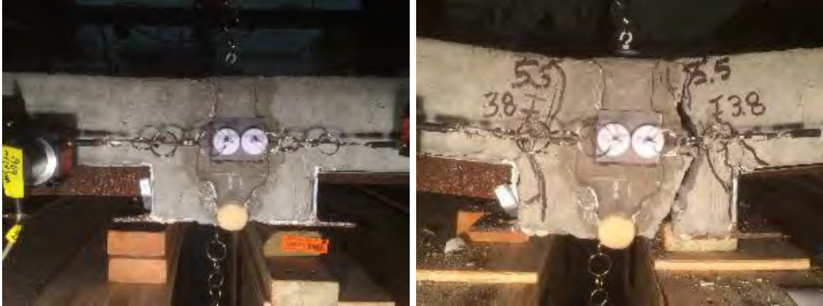
Figure 5.17 U-REV-Q Joint Before and After Test
