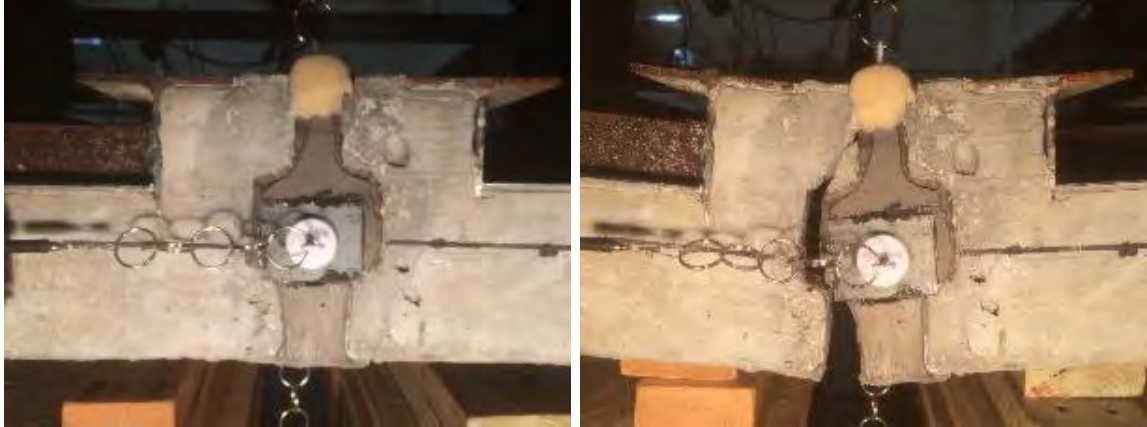
Figure 5.8 U-NEG-Q Joint Before and After Test (Inverted Specimen)
