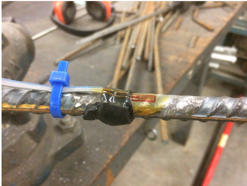
Figure 4.25 Electrical-Resistance Strain Gage (ERSG)
