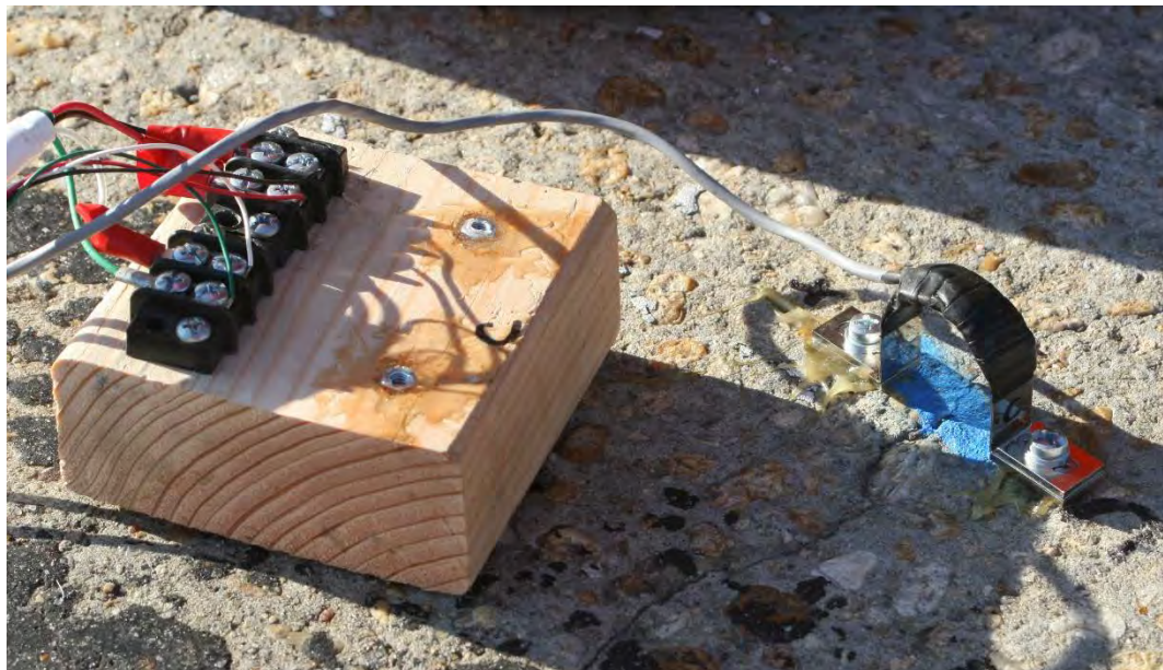
Figure 5.23 Installed Crack Opening Displacement Transducer
