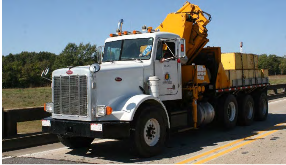
Figure 5.13 ALDOT Load Truck with LC-5 Configuration
