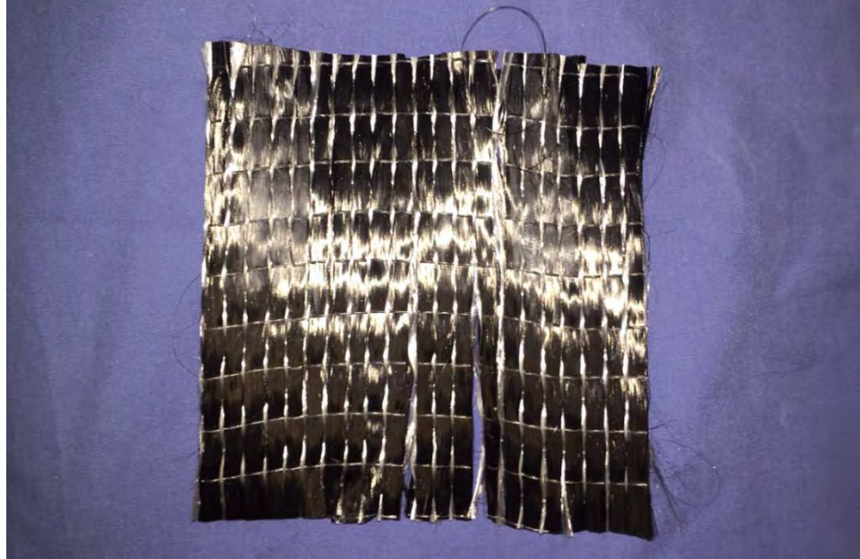
Figure 2.2 FRP Fabric Sample (Prior to Epoxy Saturation)
