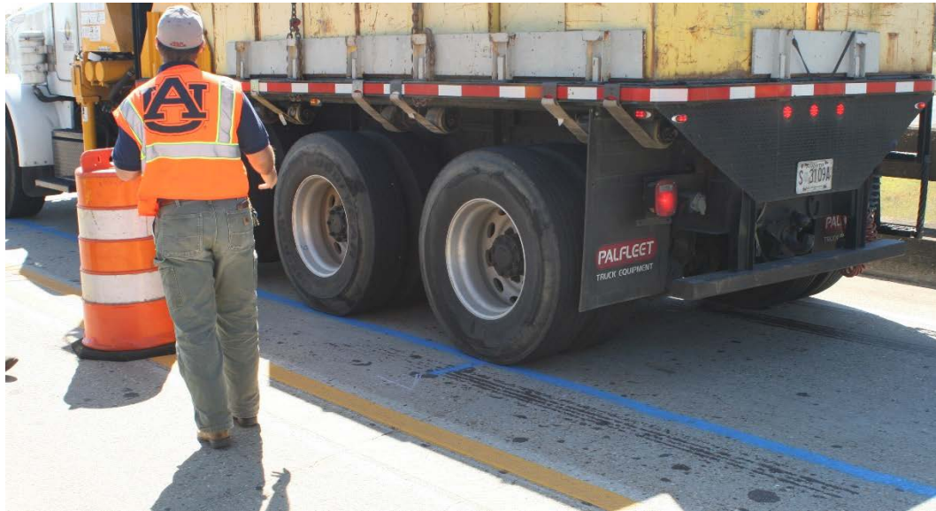
Figure 5.17 Load Truck Placement with Back Left Tire along Guideline Positions
