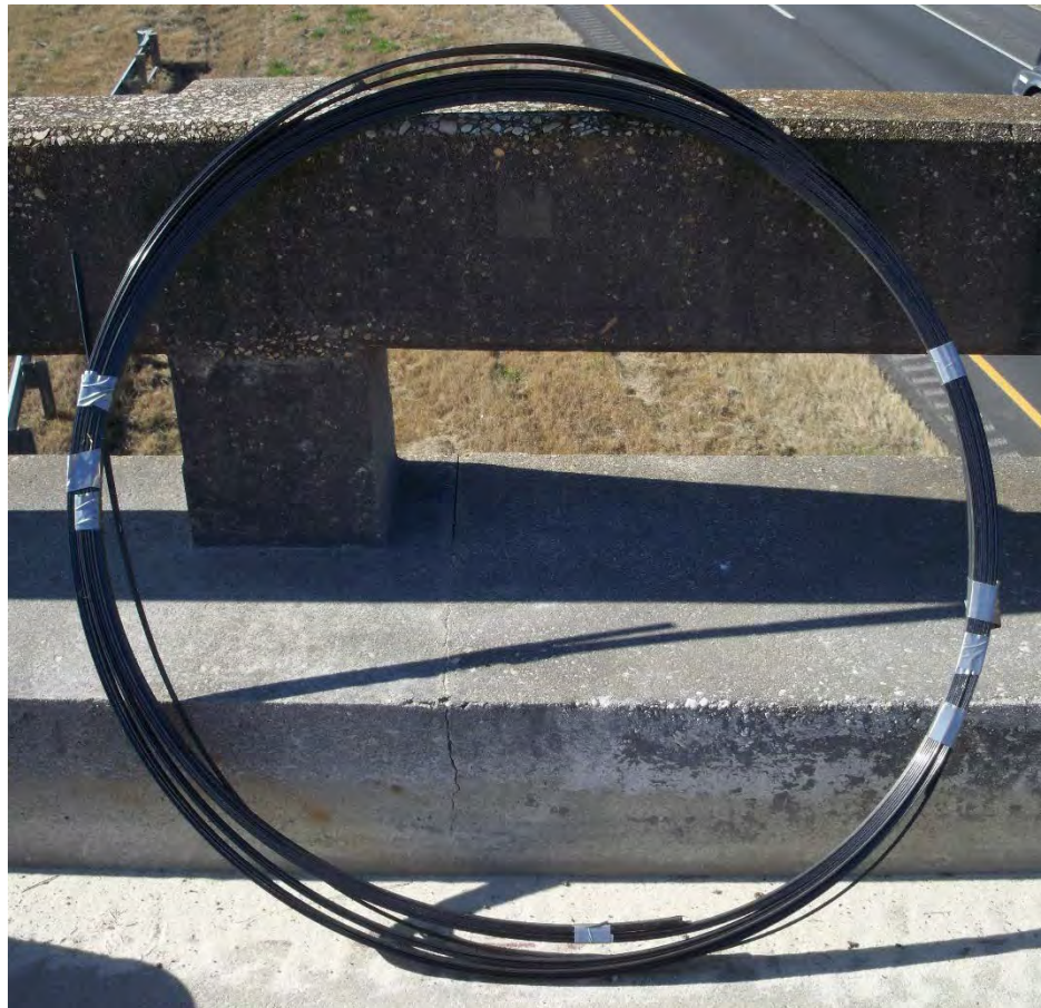
Figure 4.1 Rolls of FRP Strips Before Installation
