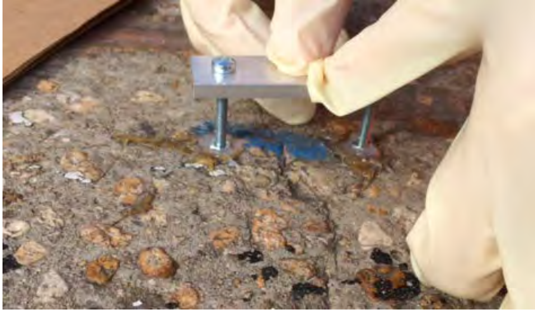
Figure 5.10 Hex Nut Placement in Epoxy
