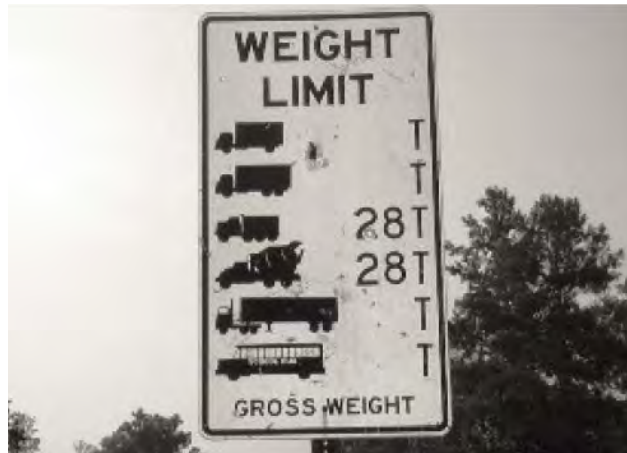
Figure 3.6 Typical ALDOT Load-Posting Sign (Alexy 2009)
