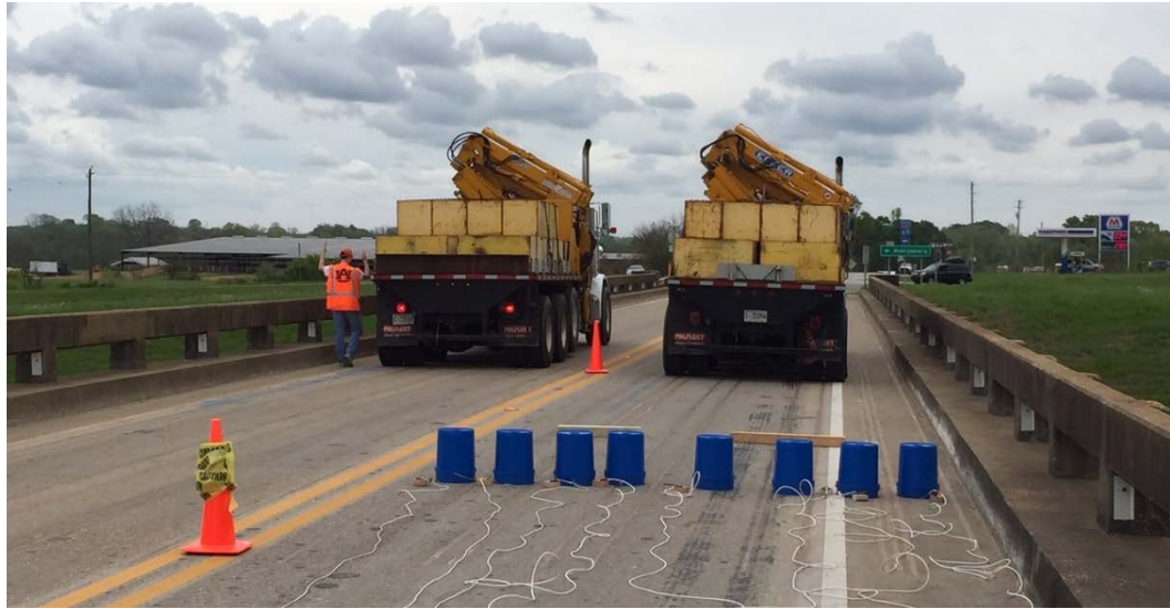
Figure 5.31 Load Test with Two Load Trucks
