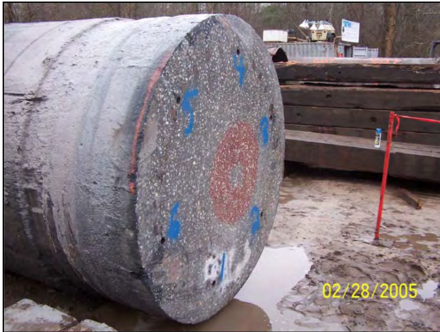
Figure 3.66: South Carolina SCC: Cross-sectional cut 6 ft from bottom (Holley et al. 2005)
