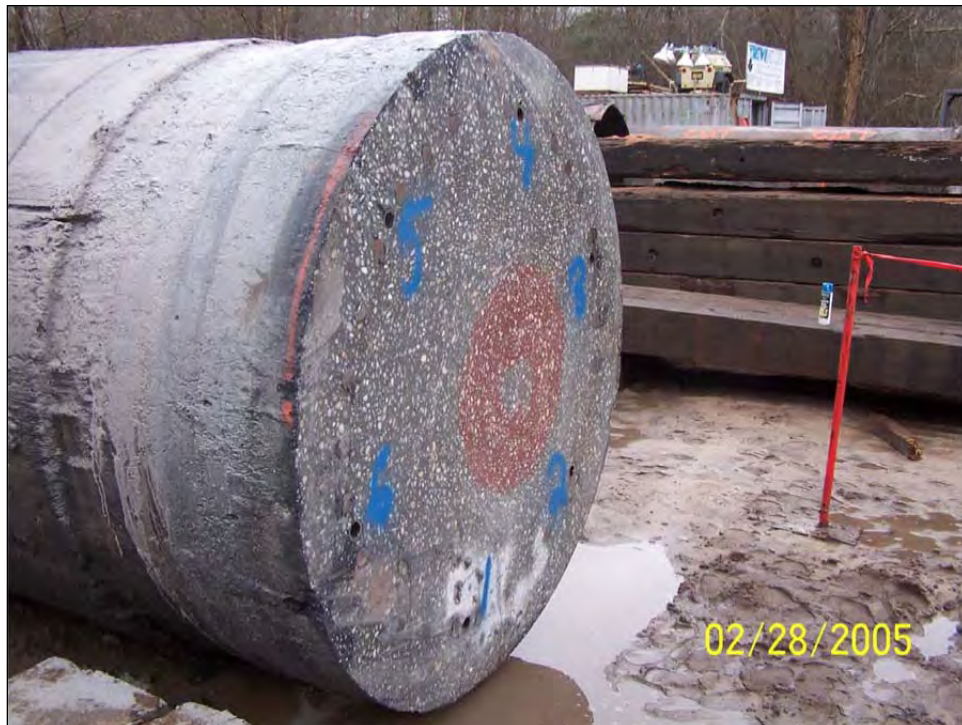
Figure 2.17: SC SCC: Cross-sectional Cut 6 ft from Bottom (Holley et al. 2005)
