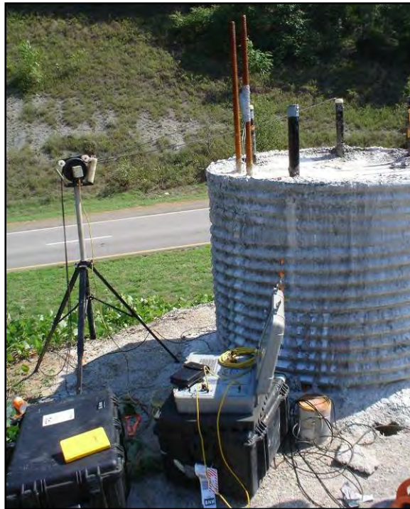
Figure 3.25: CSL testing conducted on-site
