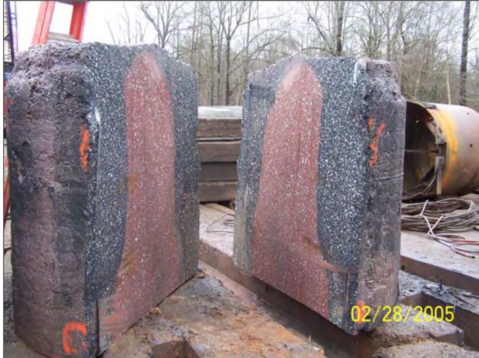
Figure 2.16: Dyed concrete showing the first concrete in the shaft staying near the bottom, filling the bottom corners of the shaft (Holley et al. 2005)
