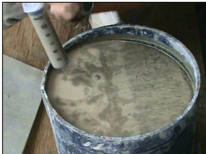
Figure 3.44: SCC bleed water after 80 minutes
