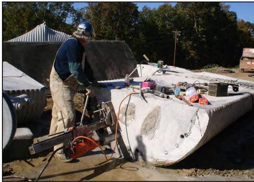
Figure 3.31: Coring SCC approximately seven feet from top of shaft
