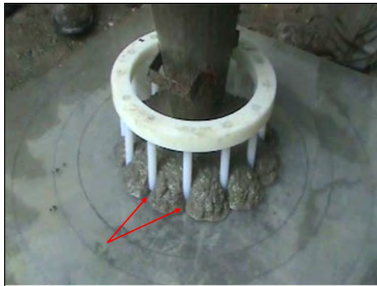
Figure 3.56: J-Ring test showing possible reason for poor consolidation on the cover of the ODSC shaft
