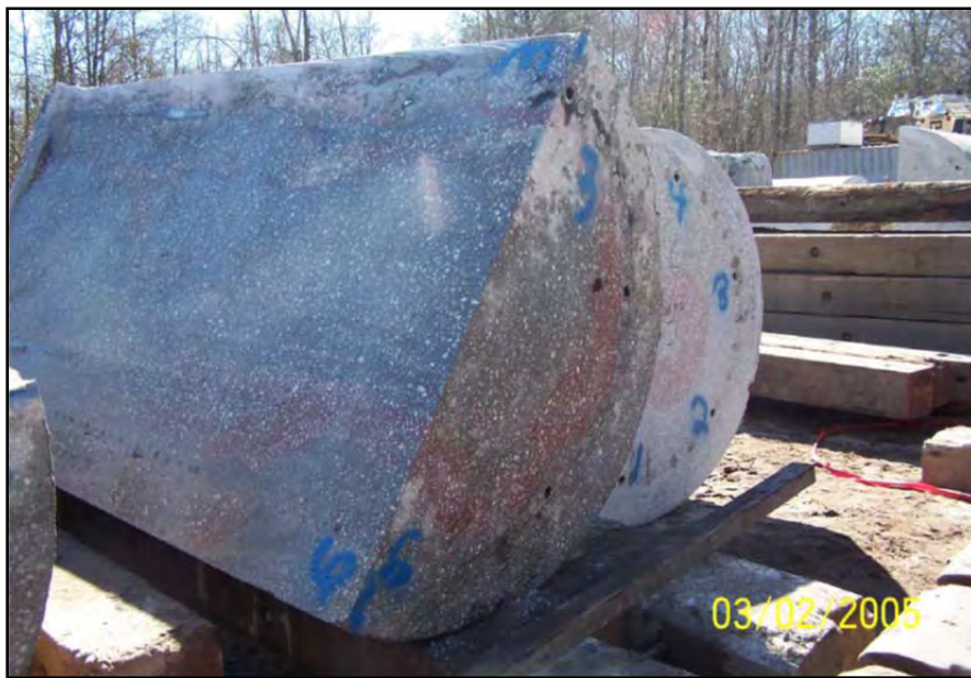
Figure 3.67: South Carolina SCC: Cross section 13 ft from bottom (Holley et al. 2005)
