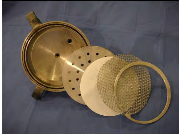
Figure 3.8: Piston cap with metal filter, filter paper, and a metal plate with holes to prevent aggregate and paste from leaving the piston chamber
