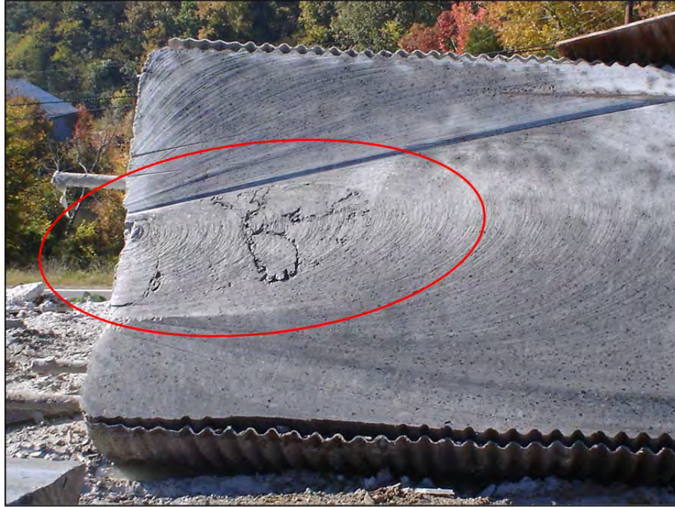
Figure 3.57: Anomaly observed near the top of the SCC-LP shaft
