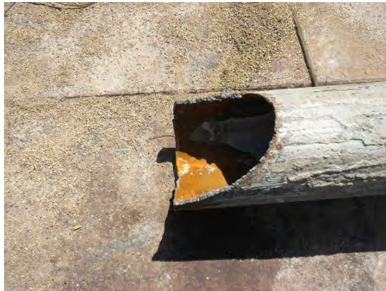
Figure 2.3: Cut groove at the bottom of the tremie
