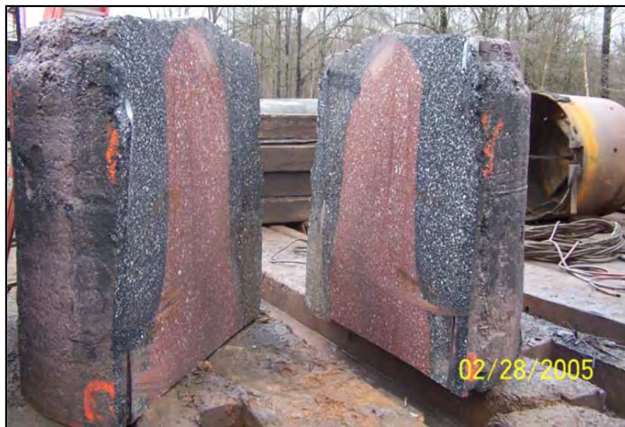
Figure 3.65: Dyed concrete in the bottom of the SC Coastal shaft (Holley et al. 2005)
