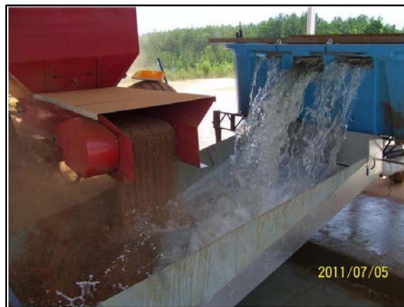
Figure 4: Water/Sediment Introduction System
