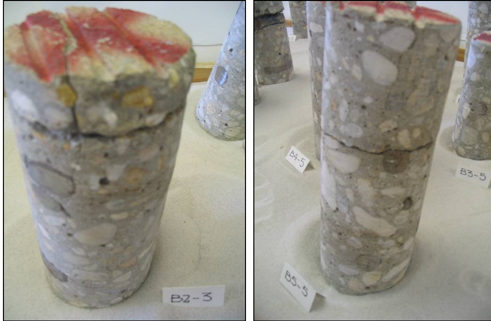
Figure 3-6: Cores from the US 331 deck with vertical and horizontal cracks
