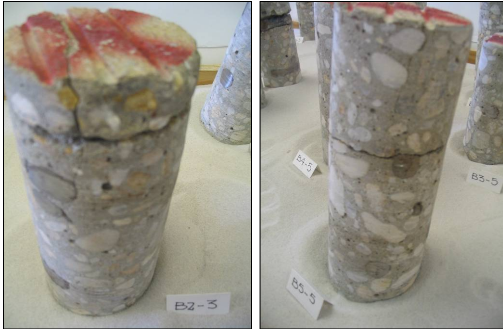
Figure 1-4: Cores from the US 331 deck with vertical and horizontal cracks
