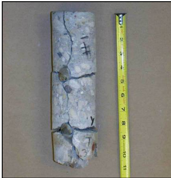
Figure 3-14: Core from CRC pavement in Texas with vertical and horizontal cracks (Courtesy of Dr. Moon Won)
