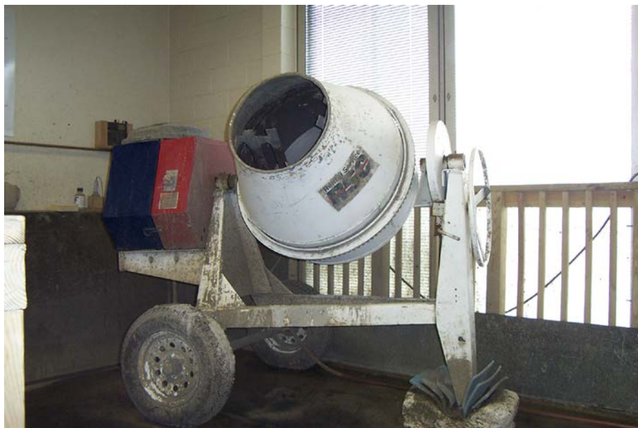
Figure 3-2: 12-ft 3 concrete mixer used for this project
