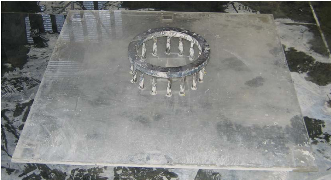
Figure 3-4: J-Ring used for this research
