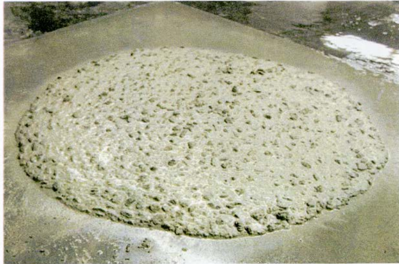
Figure 2-4: Typical Visual Stability Index Rating of 0.5 (PCI 2003)
