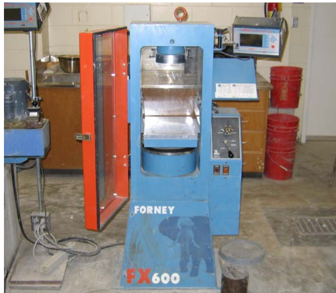
Figure 3-10: Forney compression machine
