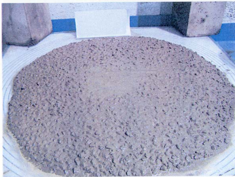
Figure 2-8: Typical Visual Stability Index Rating of 2.0 (PCI 2003)
