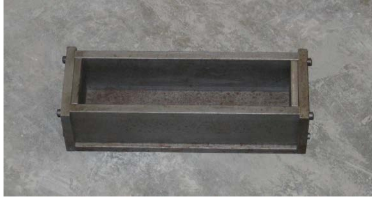
Figure 3-8: Shrinkage prism mold
