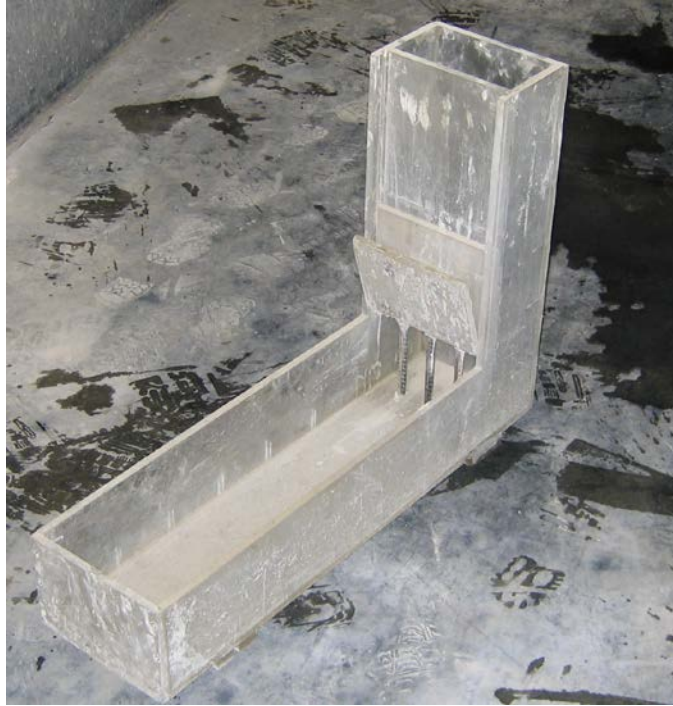
Figure 3-6: L-Box used for this project
