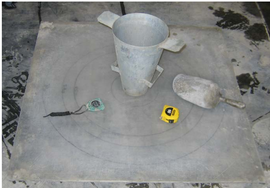
Figure 3-3: Testing equipment for slump flow test
