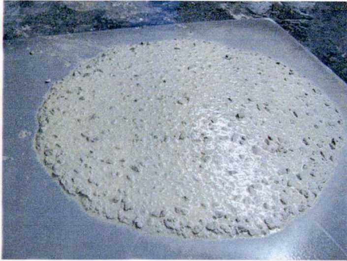
Figure 2-7: Typical Visual Stability Index Rating of 1.5 (PCI 2003)
