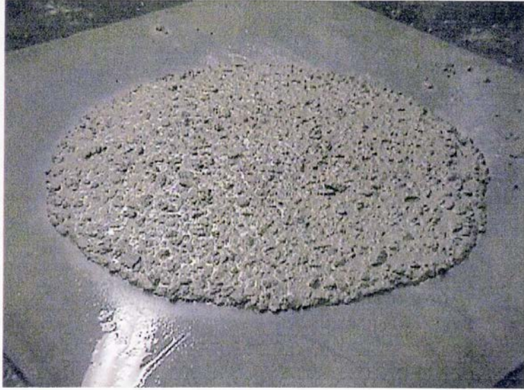
Figure 2-3: Typical Visual Stability Index Rating of 0 (PCI 2003)
