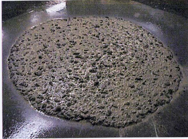
Figure 2-5: Typical Visual Stability Index Rating of 1.0 (PCI 2003)
