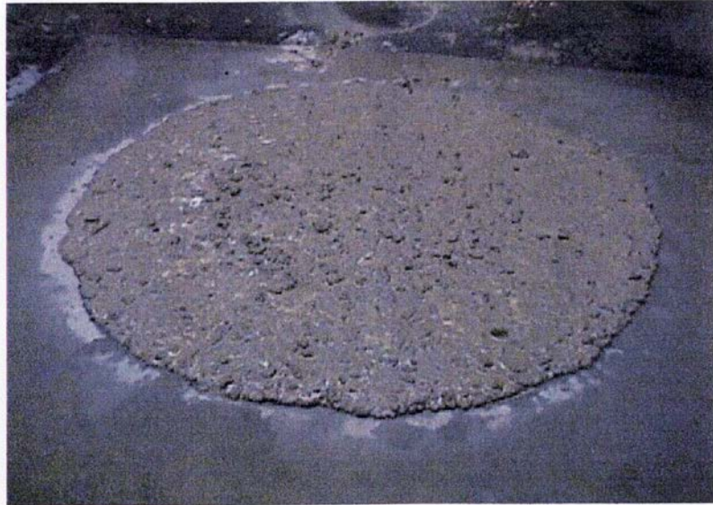
Figure 2-6: Typical Visual Stability Index Rating of 1.0 (PCI 2003)
