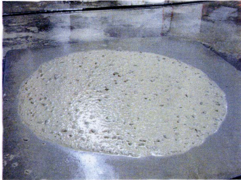
Figure 2-9: Typical Visual Stability Index Rating of 2.0 (PCI 2003)
