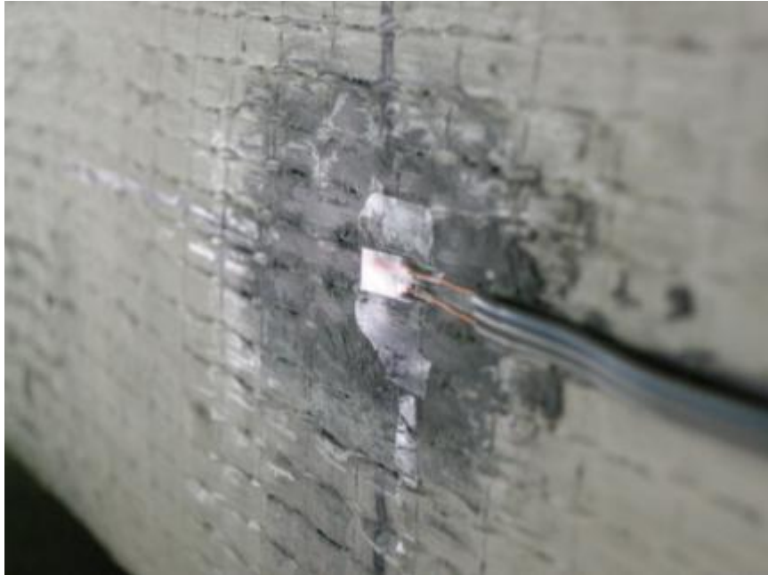
Figure M.9: Strain gage installation—gage application with thin epoxy
