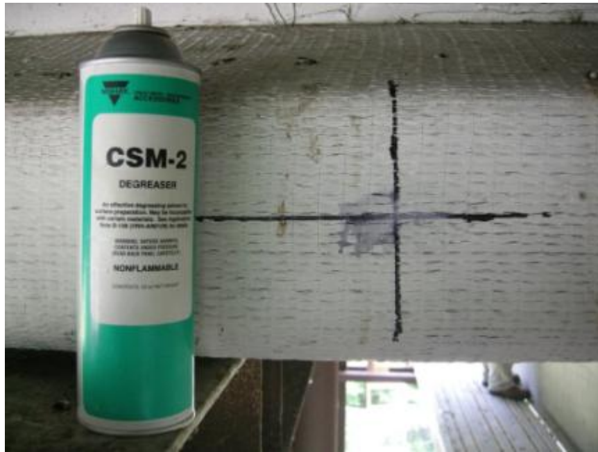
Figure 3.25: Strain gage installation—applying degreaser to gage location
