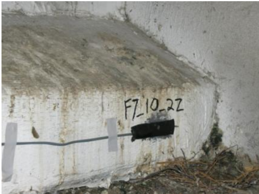
Figure M.12: Strain gage installation—mastic tape for mechanical protection
