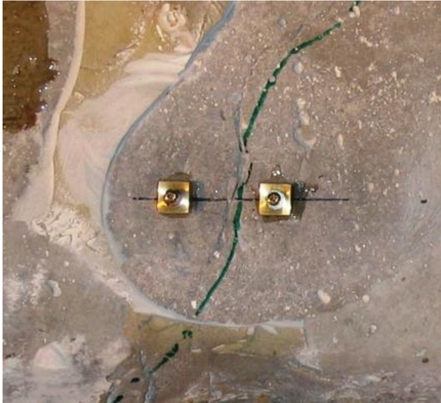
Figure 3.3: Anchor blocks for COD gage installation (Fason 2009)
