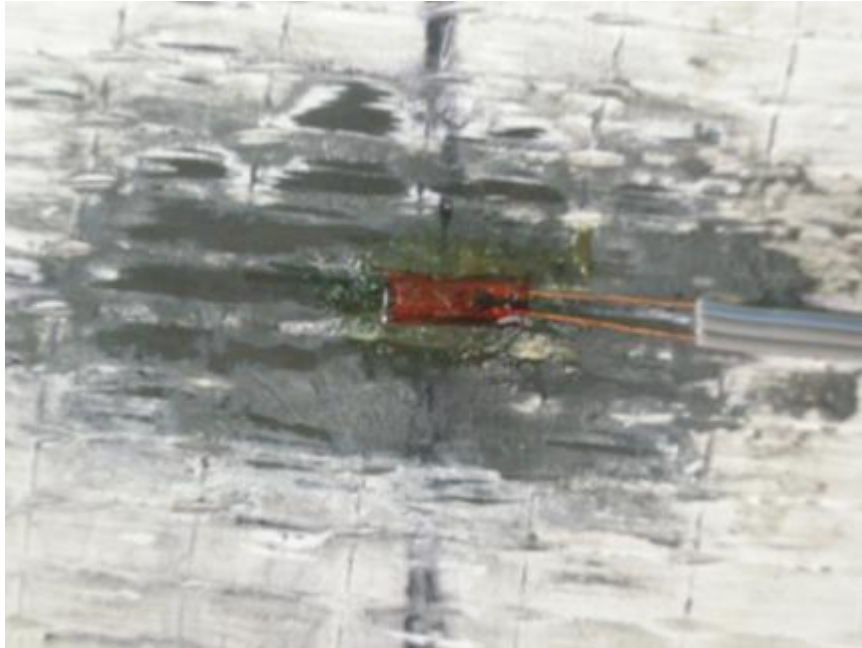
Figure 3.33: Strain gage installation—rubber coating for moisture protection
