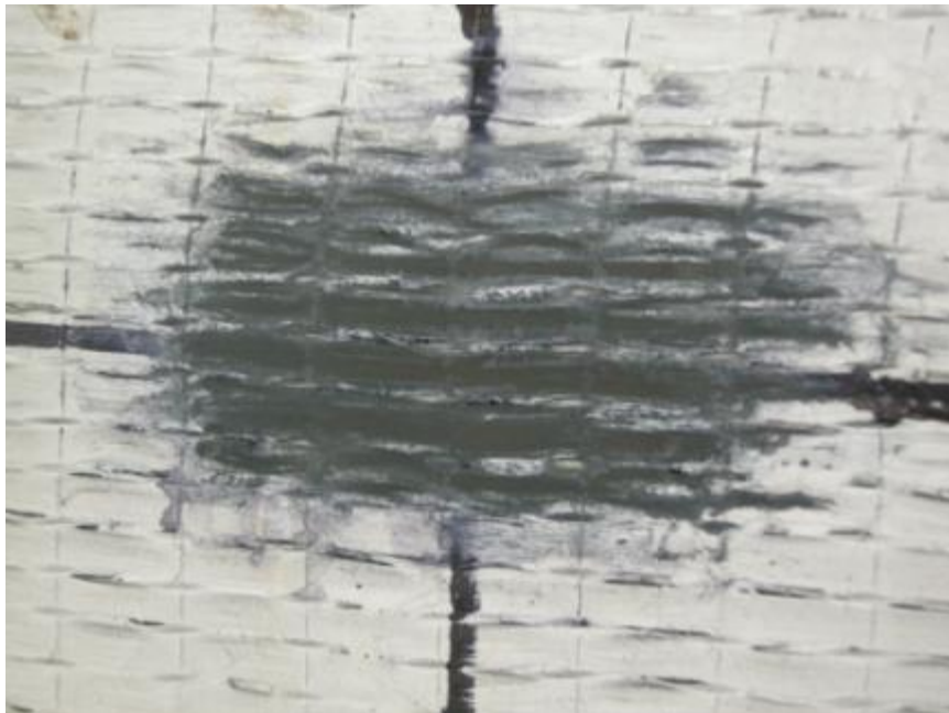
Figure M.4: Strain gage installation—clean surface prepared for solid epoxy
