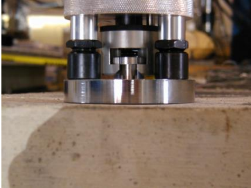
Figure 2.34: Adhesion test equipment (Swenson 2007)
