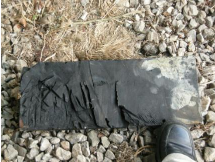
Figure 2.33: Bearing pad after forceful removal
