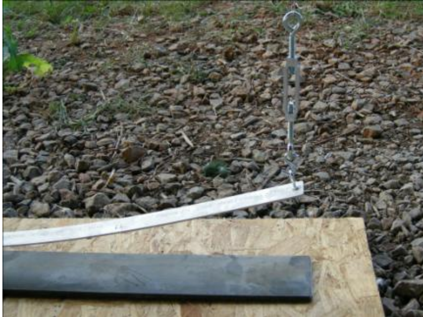
Figure 3.9: Deflector aluminum bar—pre-bent with adjusted turnbuckle
