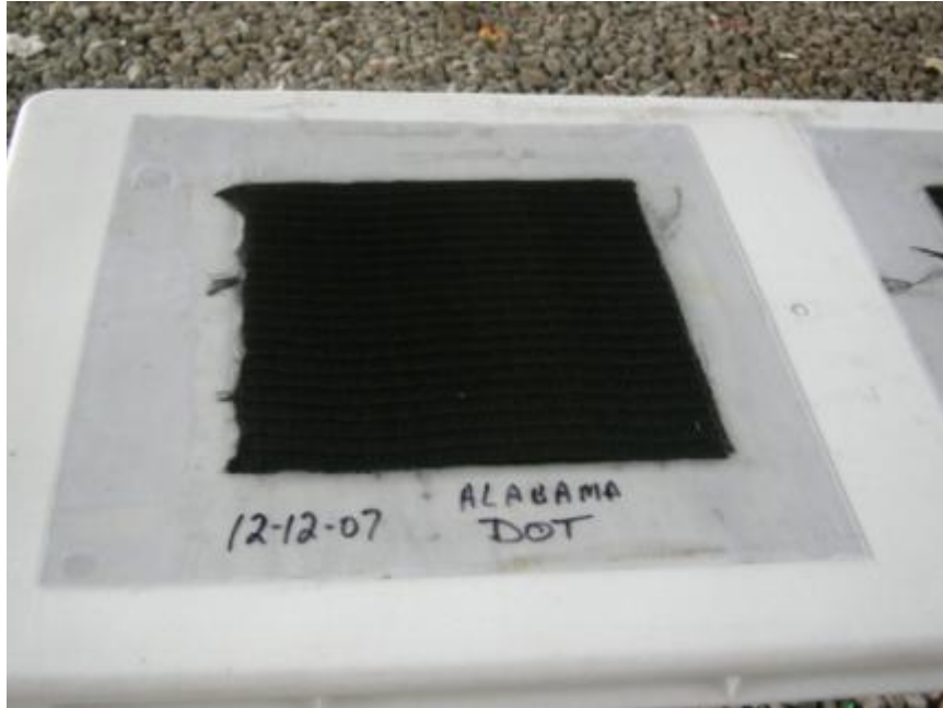
Figure 2.37: Representative sample for tension testing
