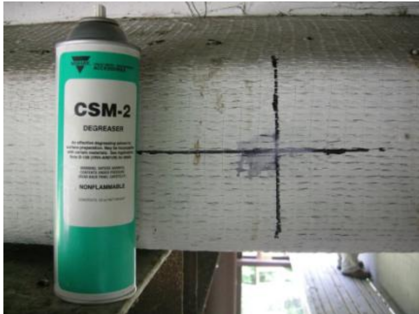
Figure M.1: Strain gage installation—applying degreaser to gage location
