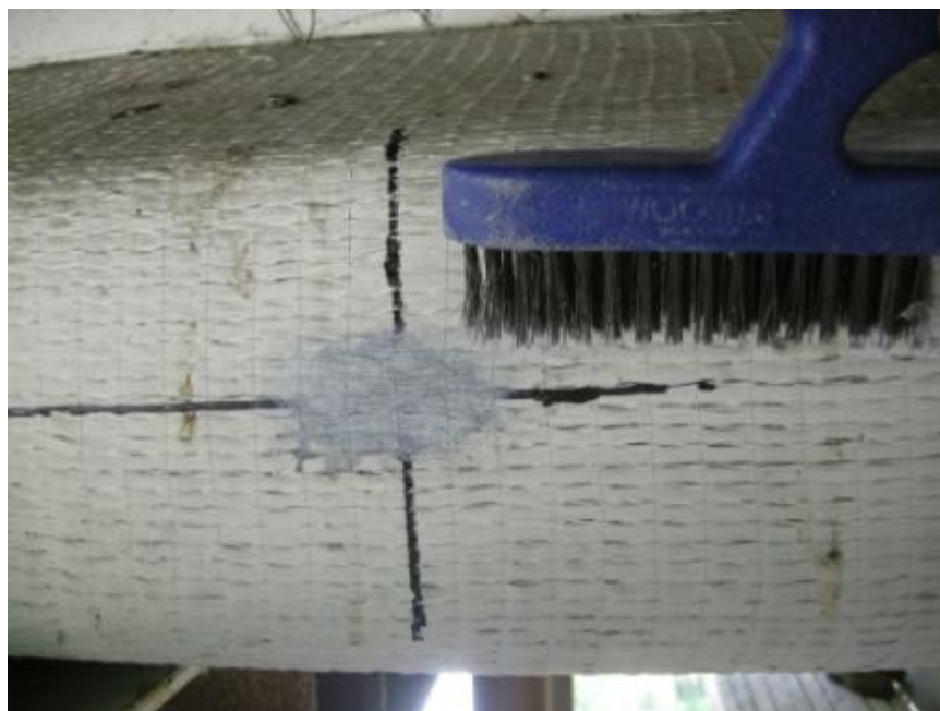
Figure 3.26: Strain gage installation—removal of surface irregularities
