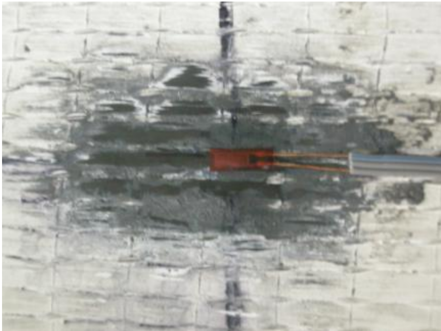
Figure M.10: Strain gage installation—gage applied to FRP reinforcement
