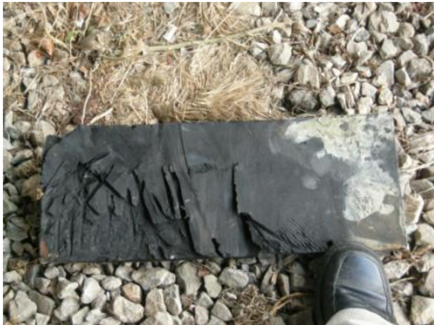
Figure K.9: Bearing pad after forceful removal
