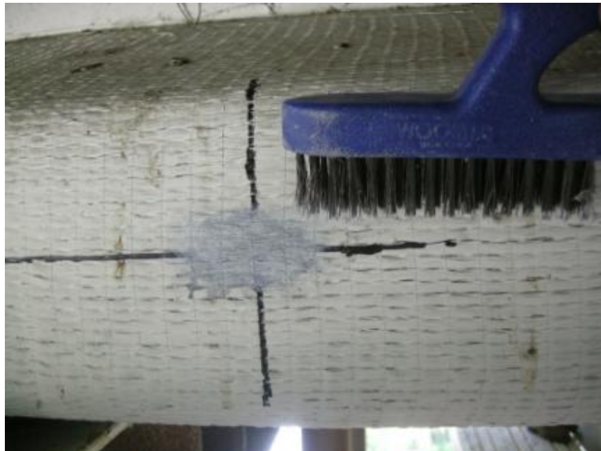
Figure M.2: Strain gage installation—removal of surface irregularities
