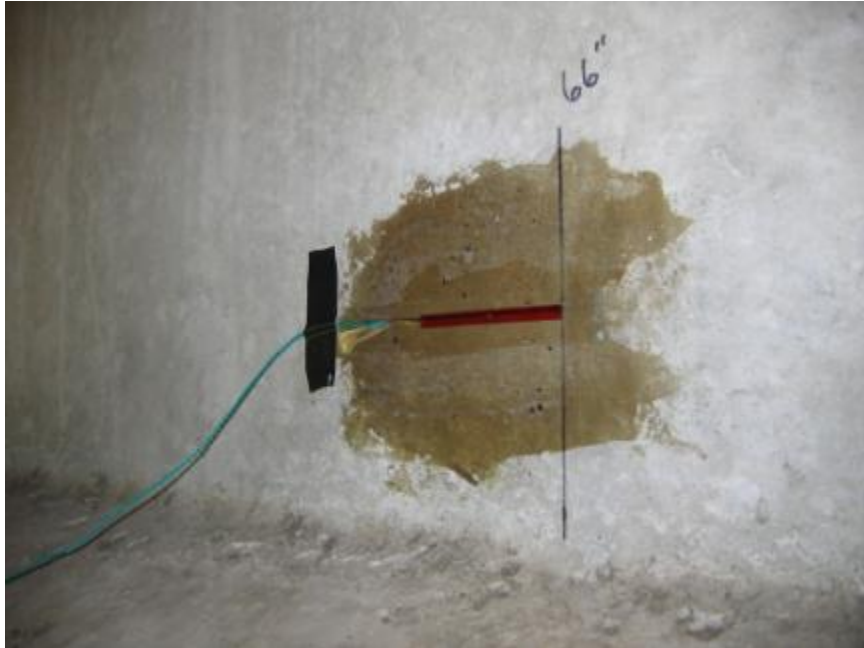
Figure 3.23: Surface-mounted strain gage—concrete (Fason 2009)
