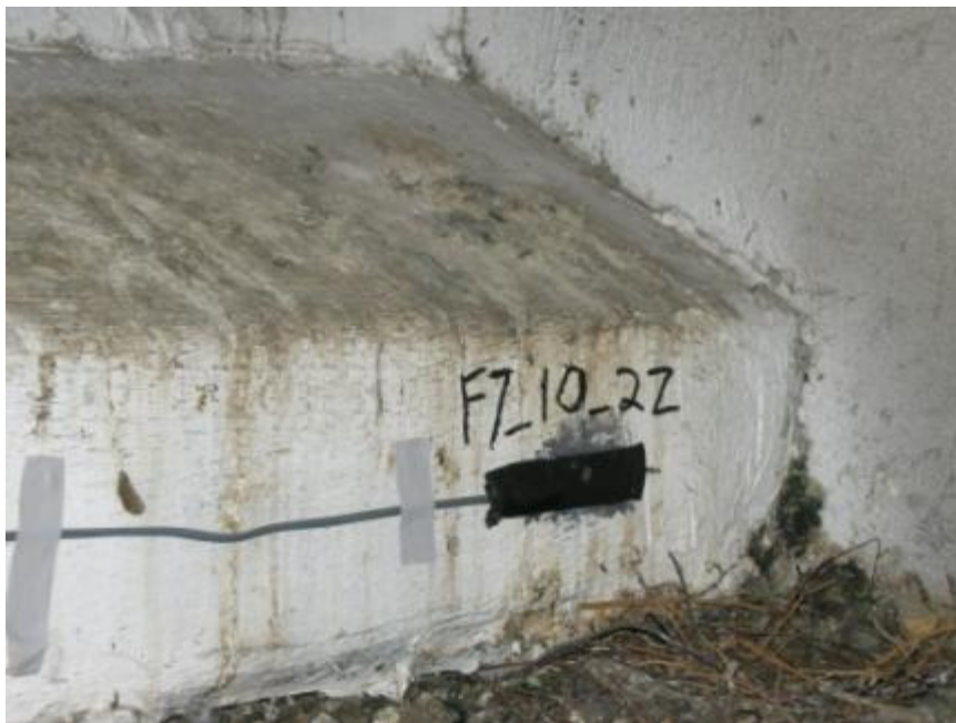
Figure 3.34: Strain gage installation—mastic tape for mechanical protection
