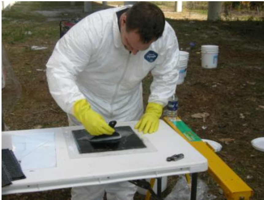
Figure 2.36: Preparation of sample for tension testing
