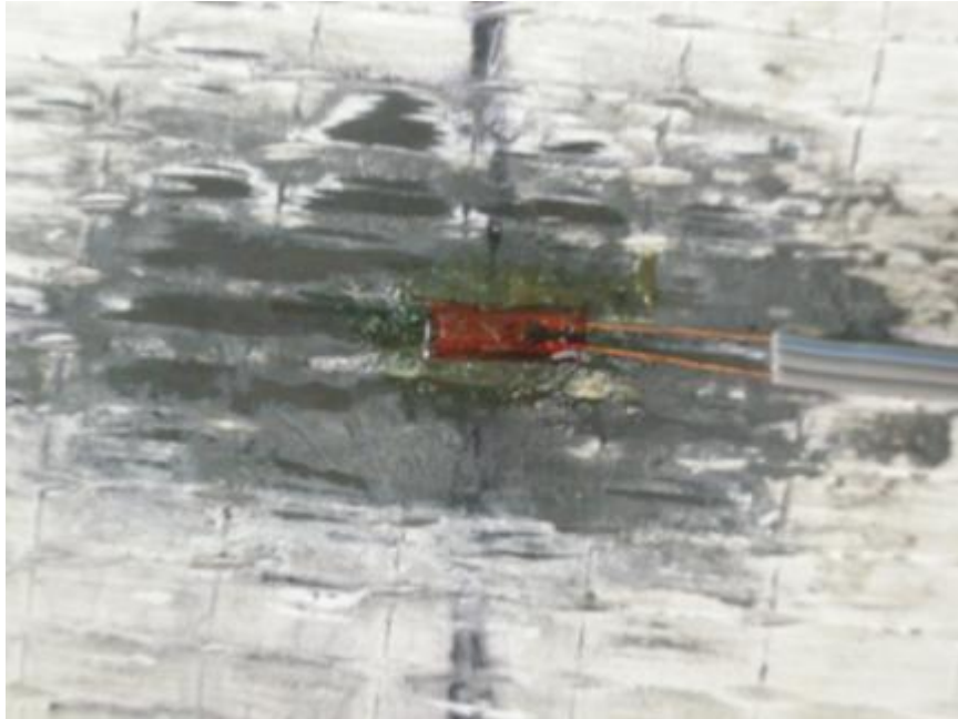
Figure M.7: Strain gage installation—rubber coating for moisture protection
