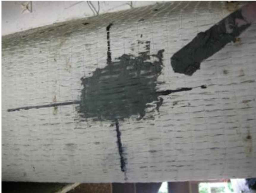
Figure 3.29: Strain gage installation—application of solid epoxy
