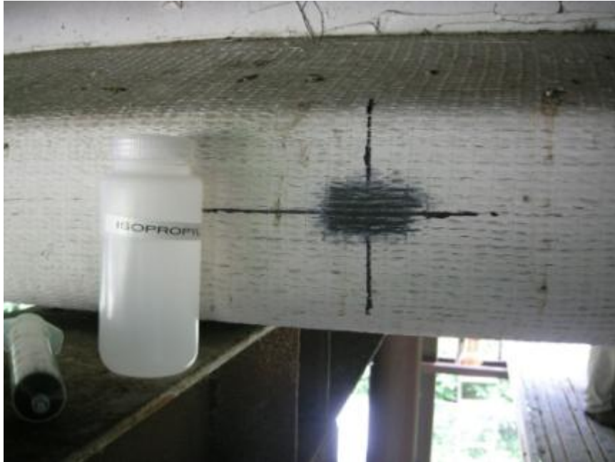
Figure M.3: Strain gage installation—initial surface cleaning
