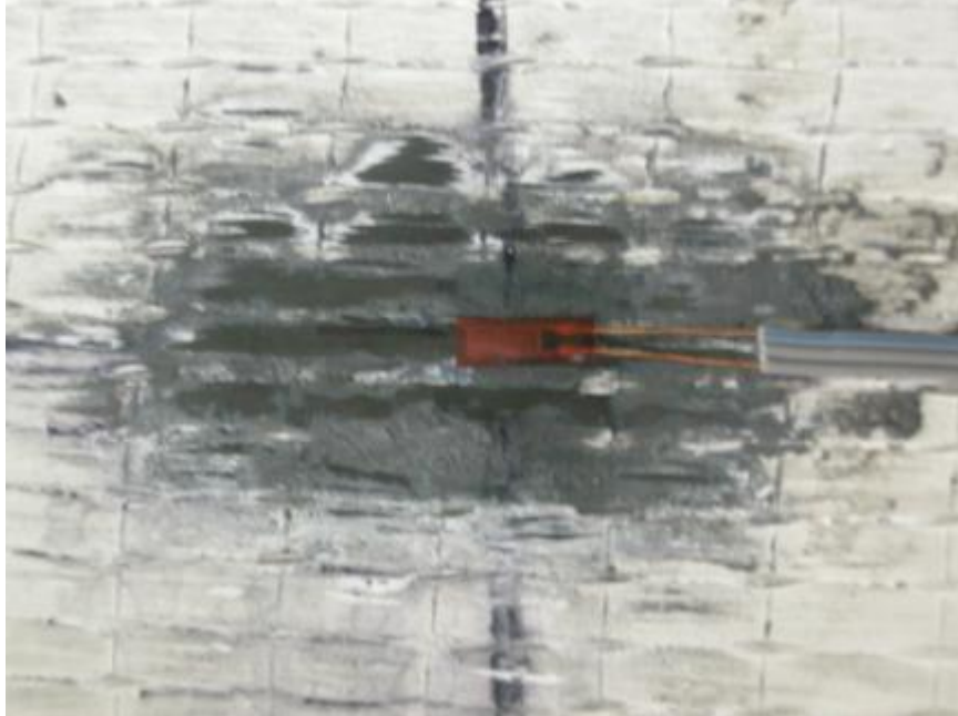
Figure 3.32: Strain gage installation—gage applied to FRP reinforcement
