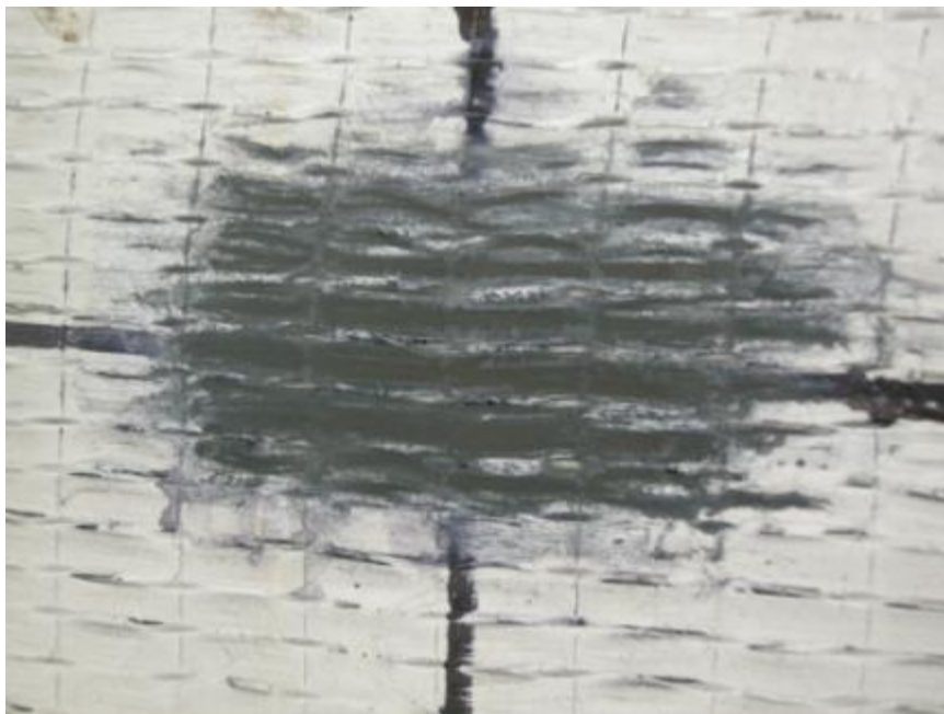
Figure 3.28: Strain gage installation—clean surface prepared for solid epoxy
