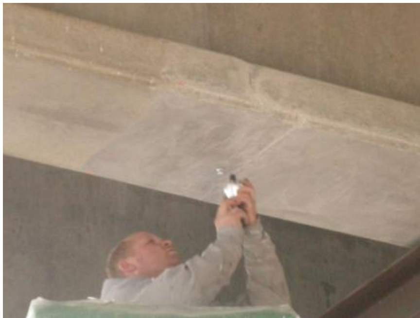
Figure 2.35: Performance of on-site adhesion test
