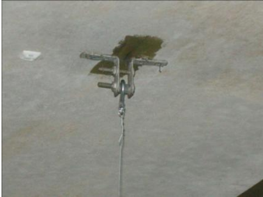
Figure 3.8: Girder attachment point for deflectometer wire
