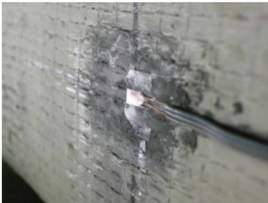
Figure 3.31: Strain gage installation—gage application with thin epoxy
