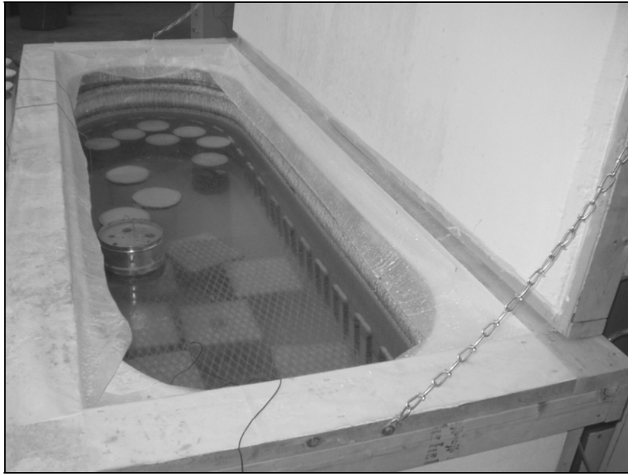
Figure 3.2: Inside of a temperature-controlled curing tank
